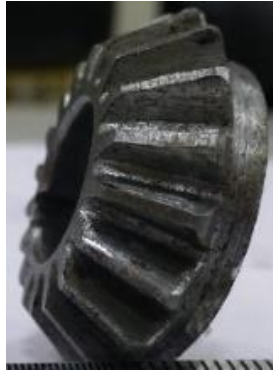
Figure 2. 4 Healthy bevel gear.
