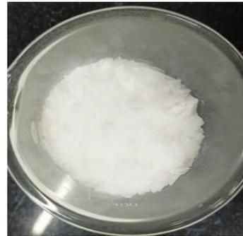
**Fig. 1.9** Polyethylene glycol - 6000 as phase change material
