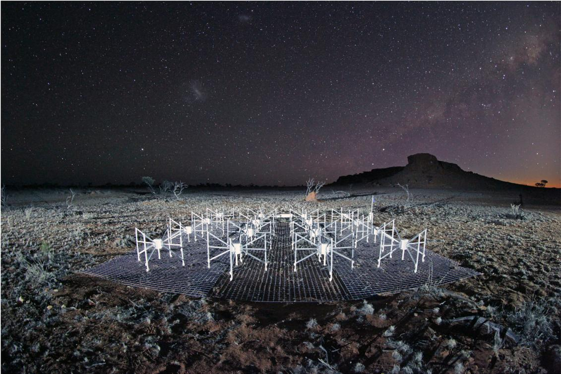
Figure 2.2: One of the 256 “tiles” that make up the MWA telescope. Each tile has 16 cross-dipole antennas, which are connected to an analogue beamformer (white box). (Image credit: Dr John Goldsmith/Celestial Visions, 2012)
