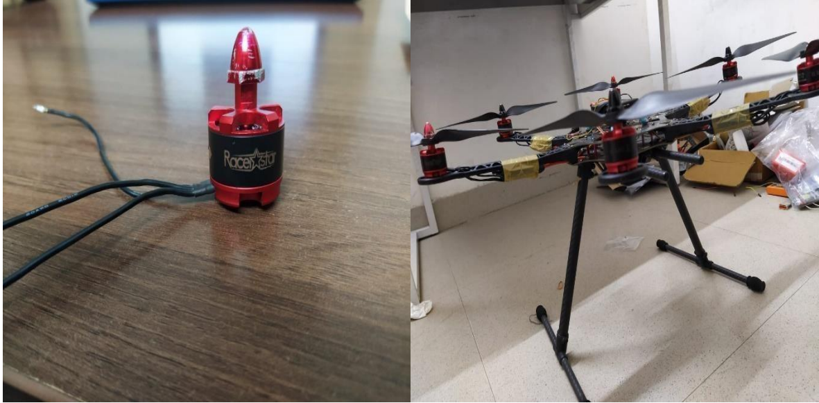
Fig2.3: Racer-star BR2212 brushless motors
