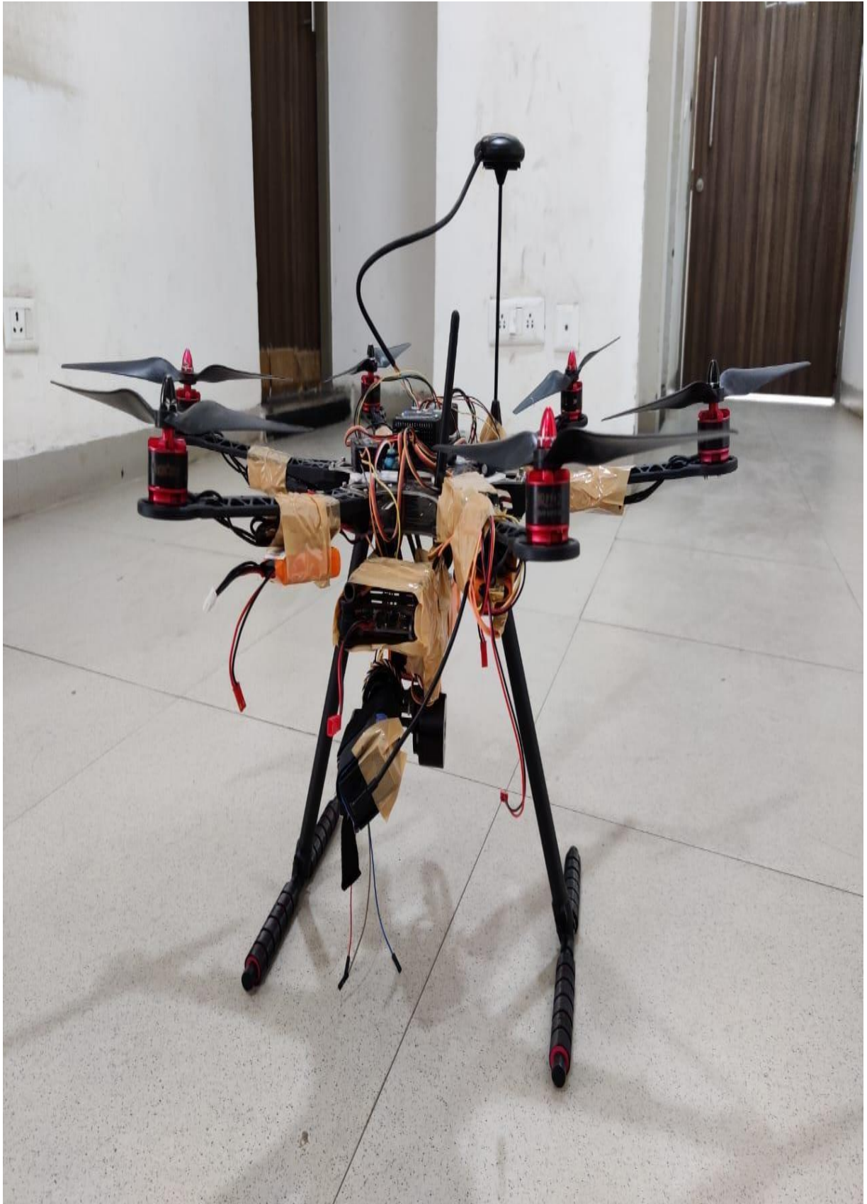
Fig2.29(b): Hexa-copter from side-view
