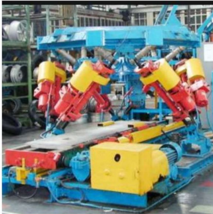
Fig.5 Tyre Testing Application of Stewart Platform
