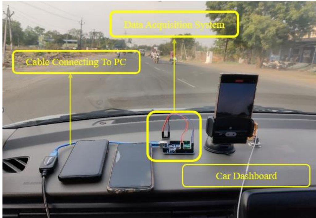
Fig 4. 1 Data acquisition system on car dashboard
