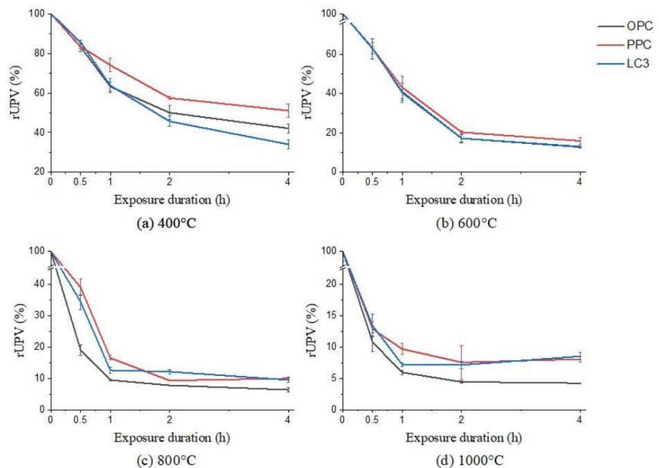
Fig. B.7 Residual UPV value of OPC, PPC, and LC3 concrete after exposure to elevated temperature at (a) 400°C, (b) 600°C, (c) 800°C, and (d) 1000°C
