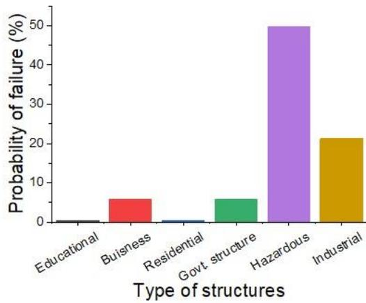
(a) Probability of failure in different structures
