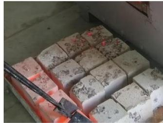
(b) Air cooling of specimen
