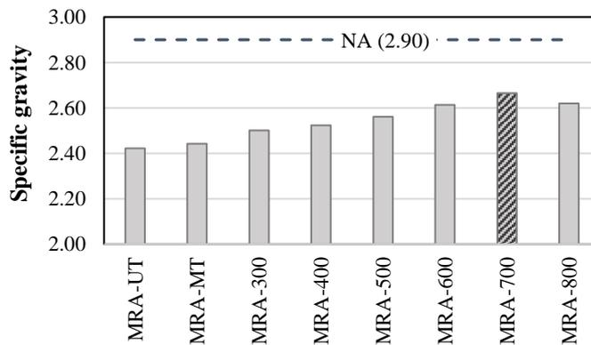
Fig. 4.7 Specific gravity of thermo-mechanically treated MRA
