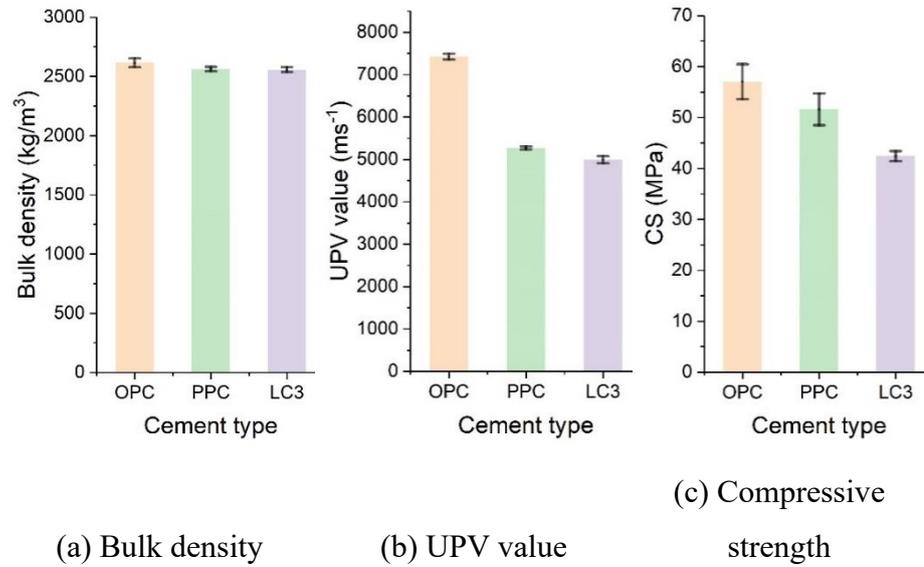
Fig. B.5 Performance of concrete at ambient temperature
