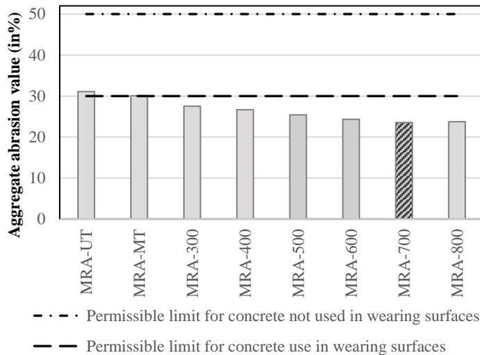
Fig. 4.11 Aggregate abrasion value of treated MRA
