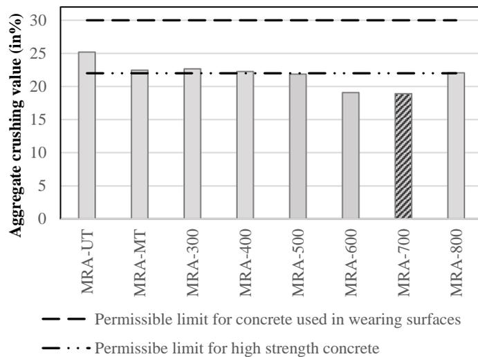
Fig. 4.9 Aggregate crushing value of treated MRA
