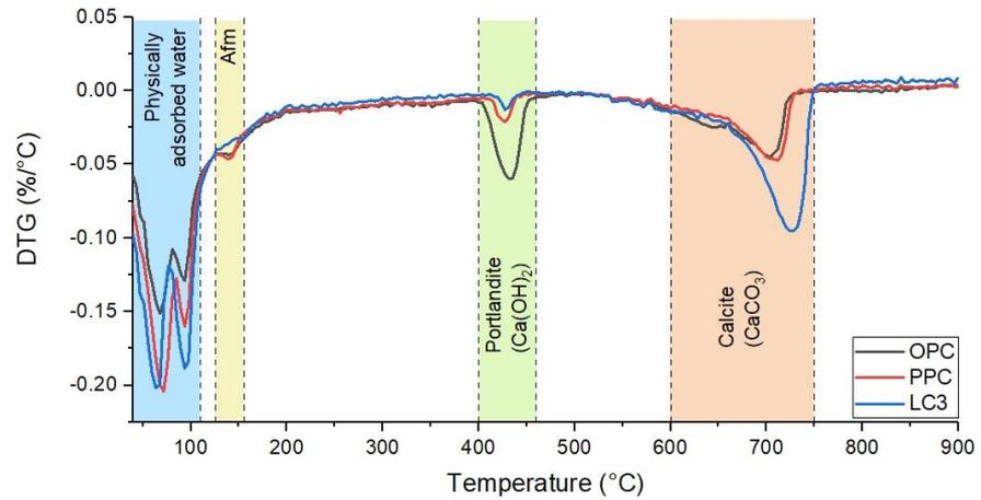
Fig. 3. TGA using DTG curve for OPC, PPC, and LC<sup>3</sup> pastes
