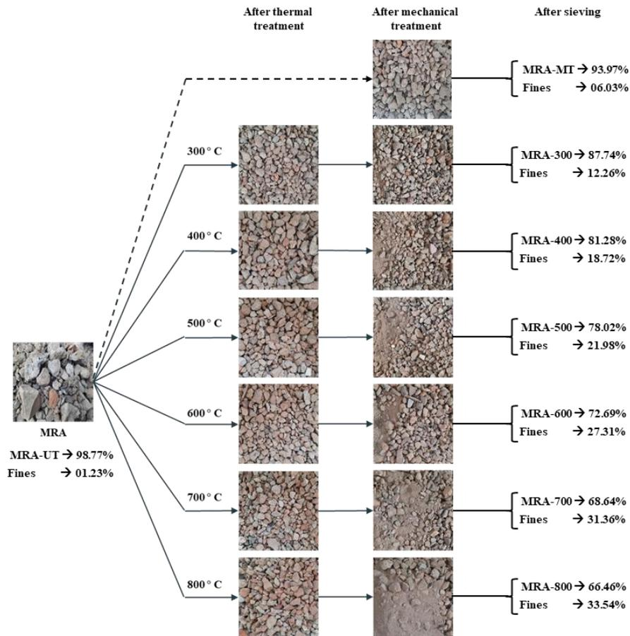
Fig. 4.5 Thermo-mechanically treated MRA(s)
