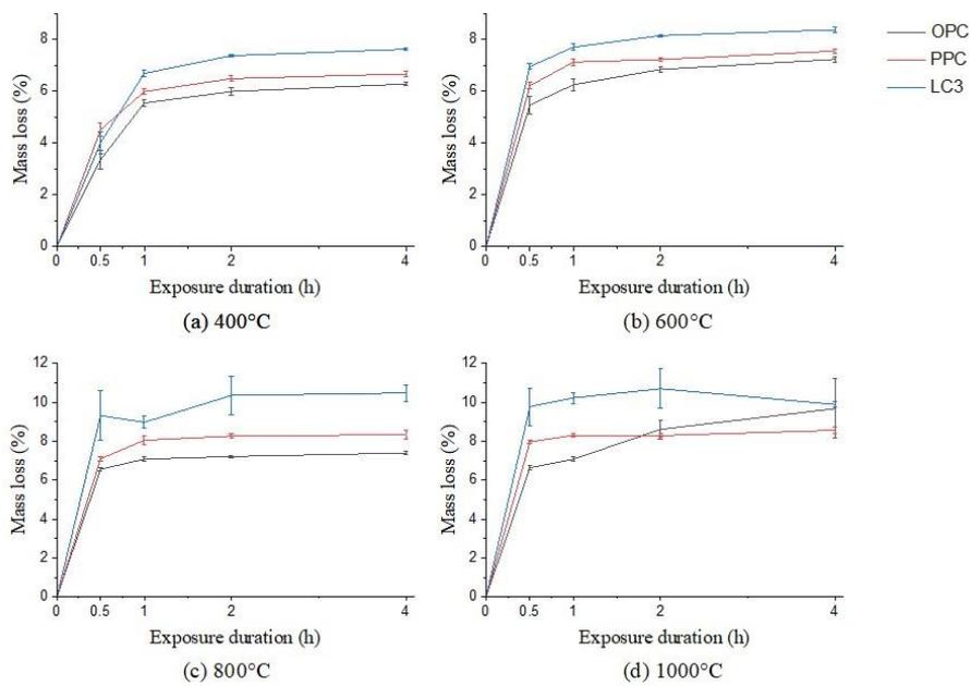
Fig. B.6 Mass loss in OPC, PPC, and LC3 concrete after exposure to elevated temperature at: (a) 400°C, (b) 600°C, (c) 800°C, and (d) 1000°C
