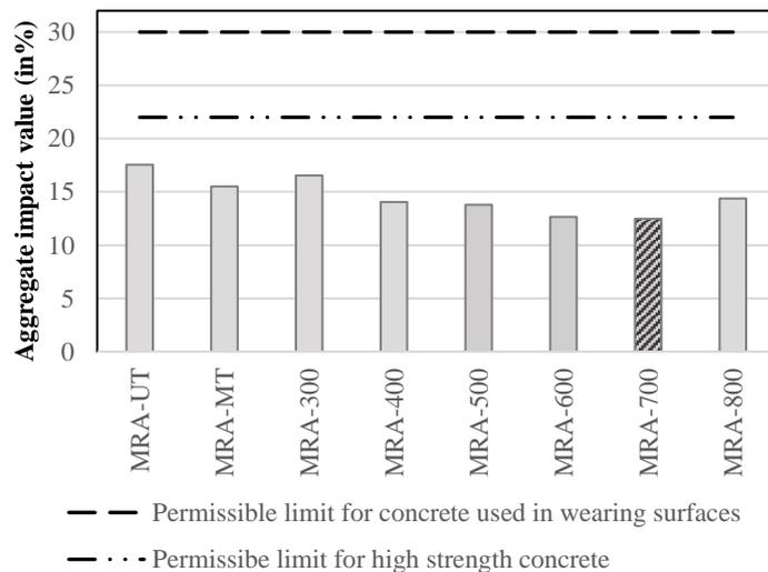
Fig. 4.10 Aggregate impact value of treated MRA
