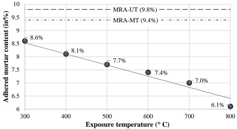
Fig. 4.6 Residual adhered mortar content in treated MRA
