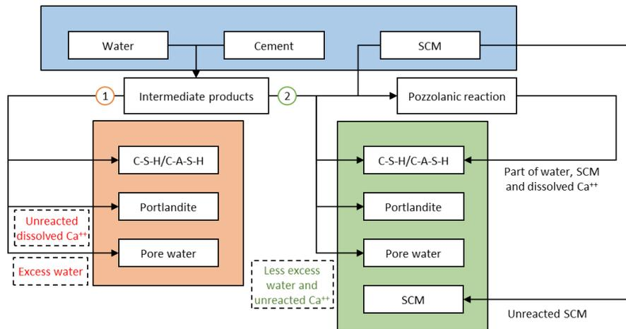
Fig. 3.8 Mineral phase changes due to clinker substitution from a durability perspective
