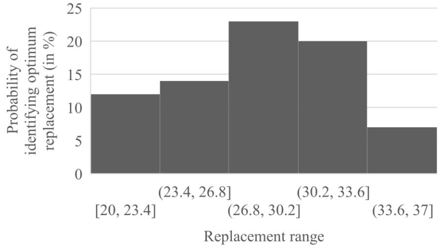
Fig. 3.10 Probability distribution function for optimum replacement of a given SCM
