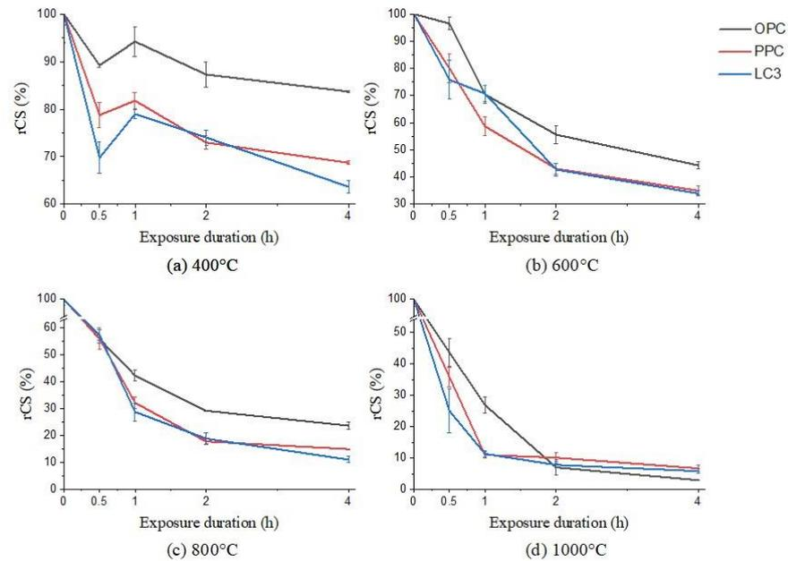
Fig. B.8 Residual compressive strength of OPC, PPC, and LC3 concrete after exposure to elevated temperature at (a) 400°C, (b) 600°C, (c) 800°C, and (d) 1000°C
