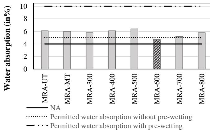
Fig. 4.8 Water absorption of treated MRA
