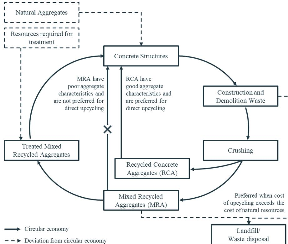
Fig. 4.1 Circular use of C&D waste as construction materials
