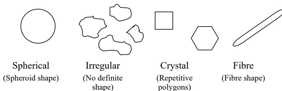
Fig. 3.3 Morphology of SCM particles
