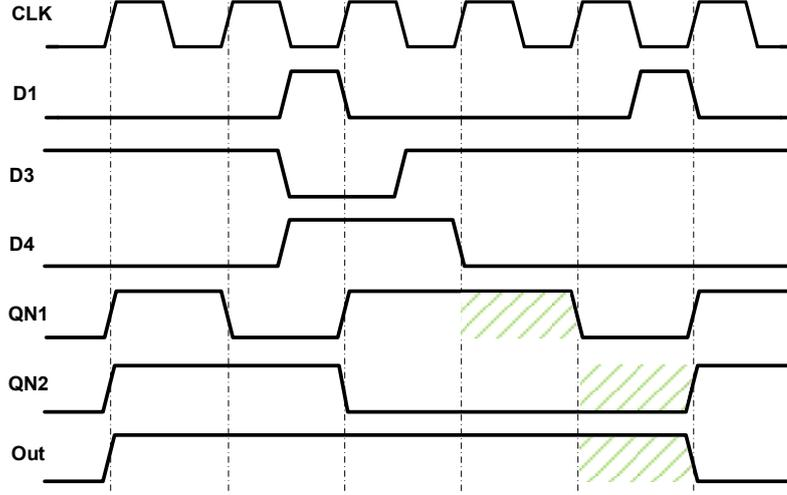
**Figure 3.10:** Divide-by-9 operation of the proposed 8/9 prescaler when MC is "1"
