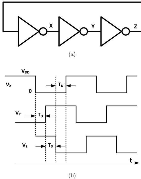
**Figure 2.12:** (a) Ring oscillator with three inverter stages (b) Working principle of three stage ring oscillator
