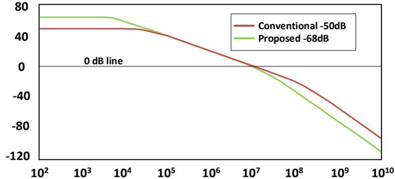
**Figure 6.6:** Frequency response of the Proposed and Conventional Opamp
