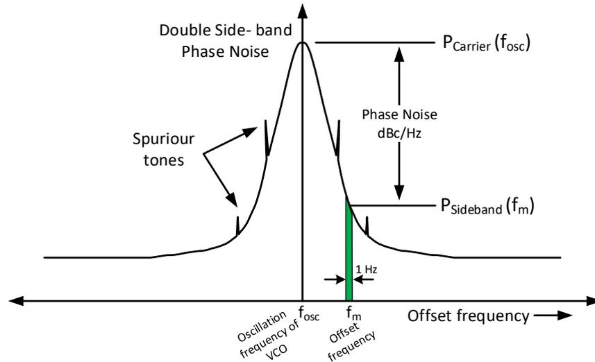
**Figure 2.21:** Presence of reference spurs in phase noise of PLL
