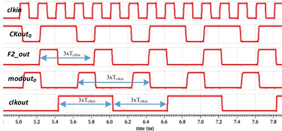
Figure 4.11: Timing waveform during divide-by-6 operation at 5 GHz input frequency
