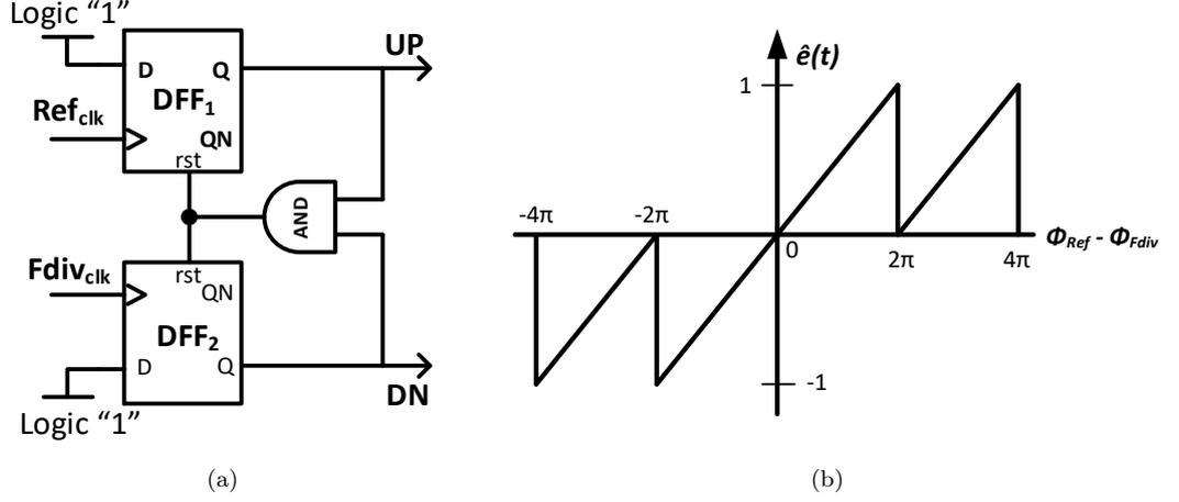
**Figure 2.6:** (a) Tri-state PFD (b) Gain of PFD
