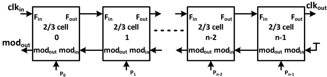
Figure 2.16: 2/3 prescaler based programmable divider
