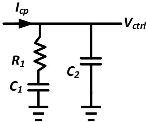
Figure 7.5: Second order passive loop filter
