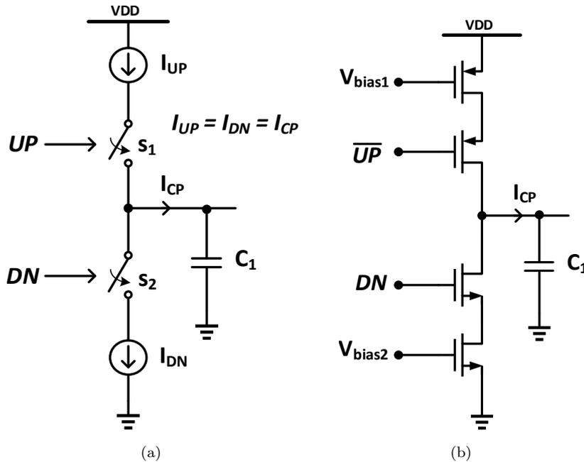
**Figure 2.9:** (a) Basic concept of a charge pump (b) Transistor level implementation
