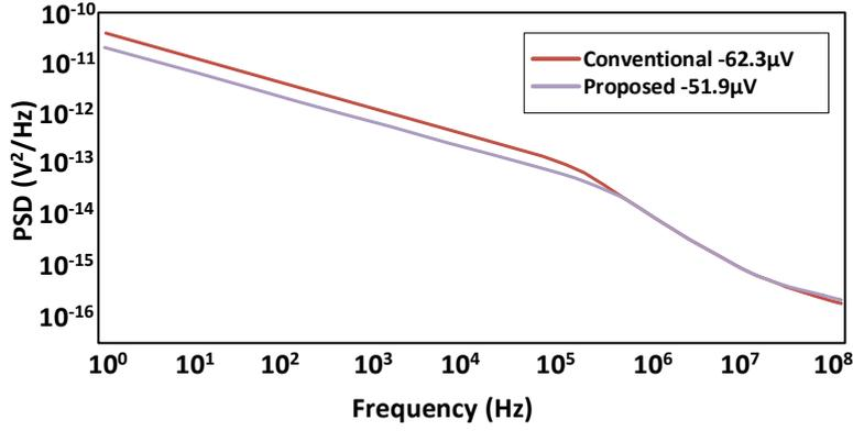
Figure 6.7: Simulated noise of the Proposed and Conventional Opamp
