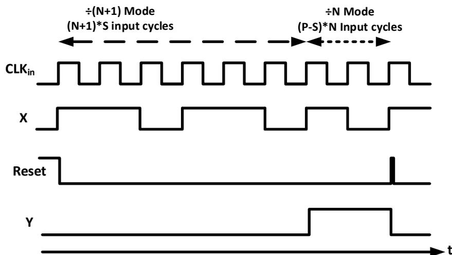
Figure 2.15: Timing waveform of Pulse Swallow Divider
