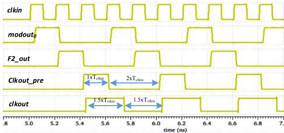
Figure 4.8: Timing waveform during divide-by-3 operation at 5 GHz input frequency
