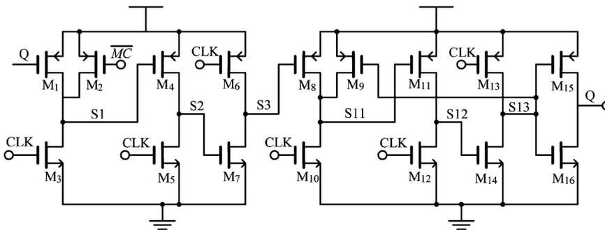
**Figure 3.5:** Gate level schematic of 2/3 prescaler proposed in [61]
