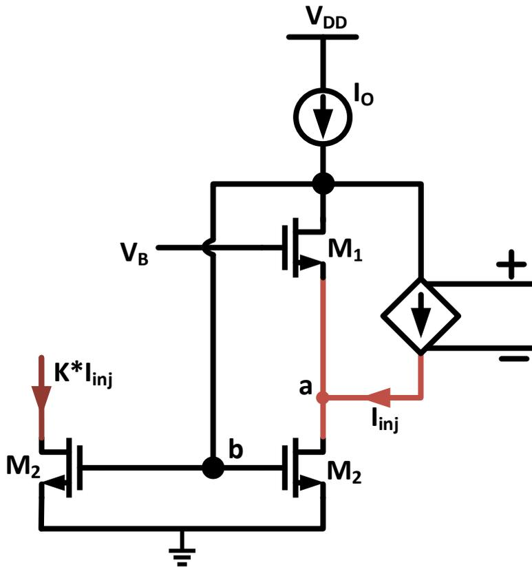
Figure 6.3: Flipped Voltage Follower (FVF) assisted differential pair
