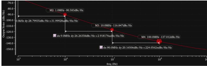
Figure 7.4: Simulated open loop phase noise of the VCO
