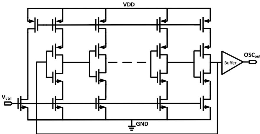
**Figure 2.13:** Basic architecture of Current Starved VCO
