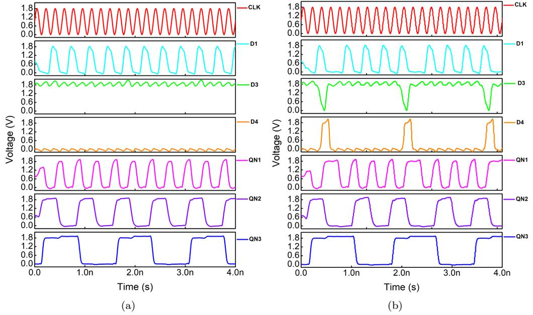
**Figure 3.12:** Waveform of internal nodes at 5.5 GHz during (a) divide-by-8 mode (b) divide-by-9 mode
