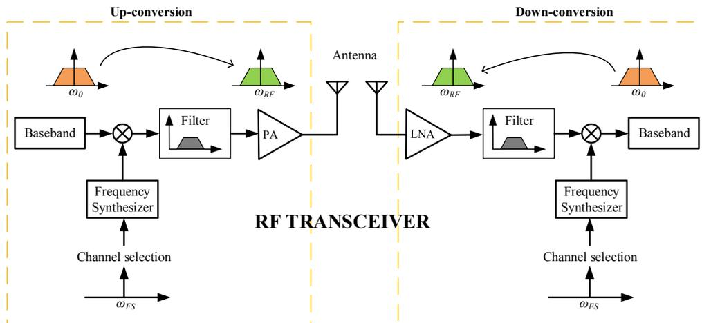
Figure 1.3: Frequency synthesis in RF transceiver
