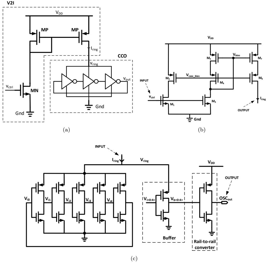
**Figure 7.2:** (a) Conceptual block diagram of VCO (b) Schematic of voltage to current converter (c) Schematic of current controlled oscillator
