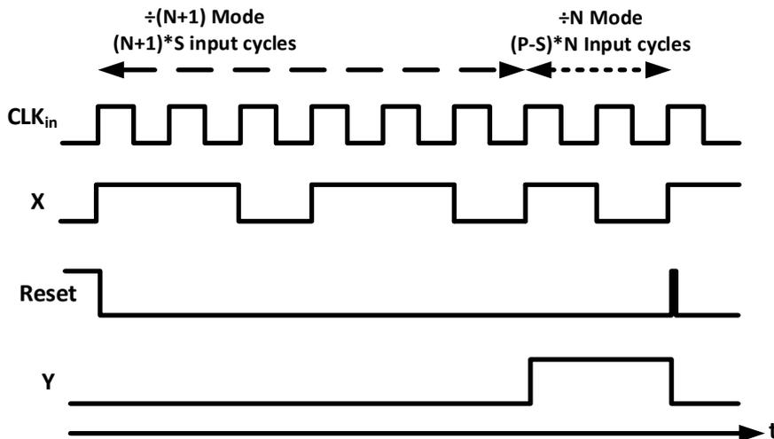
Figure 4.4: Waveform of internal node in Pulse Swallow Counter based frequency divider
