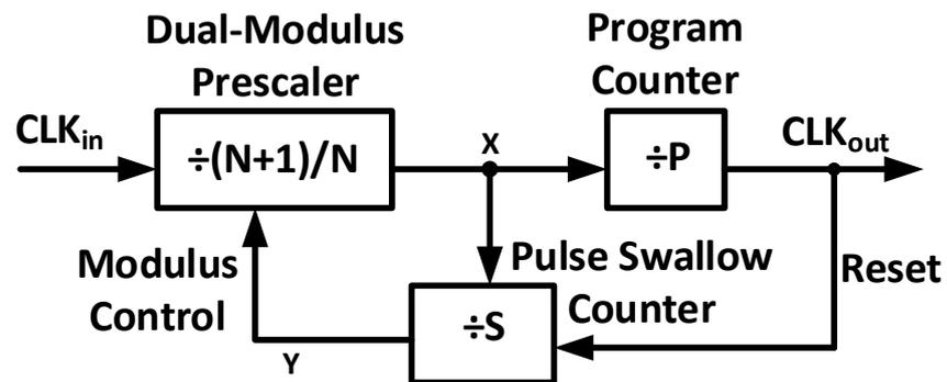
Figure 2.14: Block diagram of Pulse Swallow Divider
