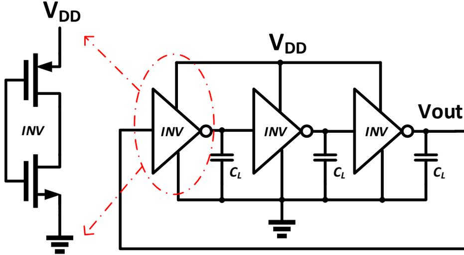
Figure 5.5: Simplified diagram of ring oscillator
