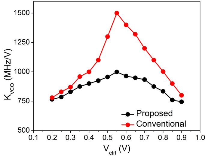
Figure 5.11:  $K_{VCO}$  variation with  $V_{ctrl}$
