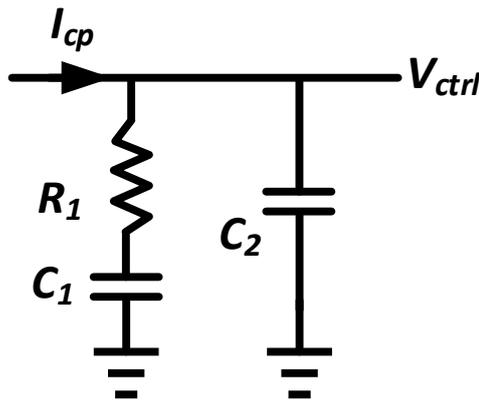
Figure 2.11: Second order passive loop filter
