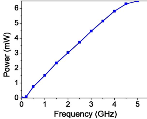
Figure 4.16: Power versus frequency of the proposed circuit
