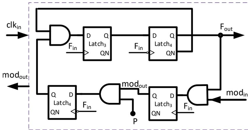
Figure 2.17: Architecture of Vaucher's 2/3 dual modulus prescaler
