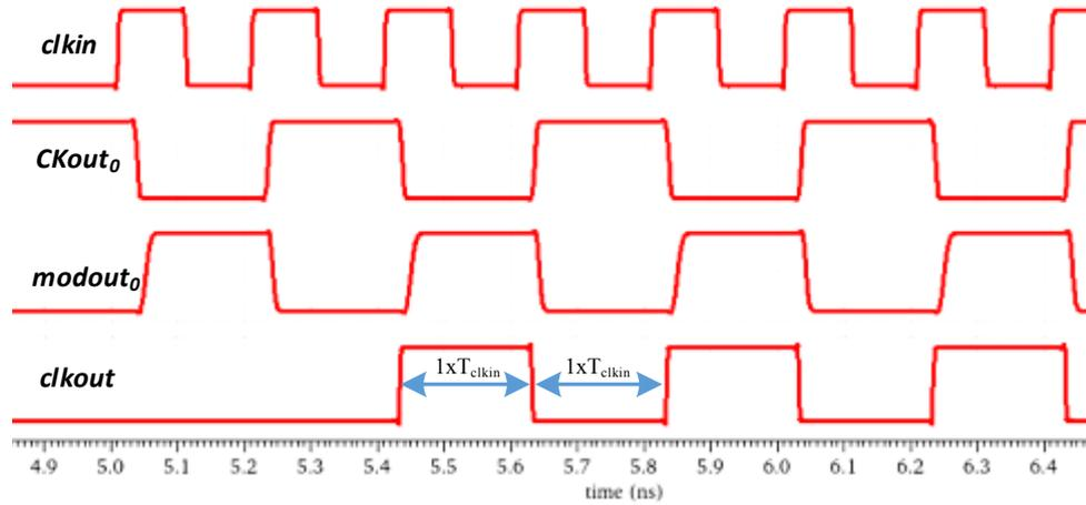
Figure 4.7: Timing waveform during divide-by-2 operation at 5 GHz input frequency
