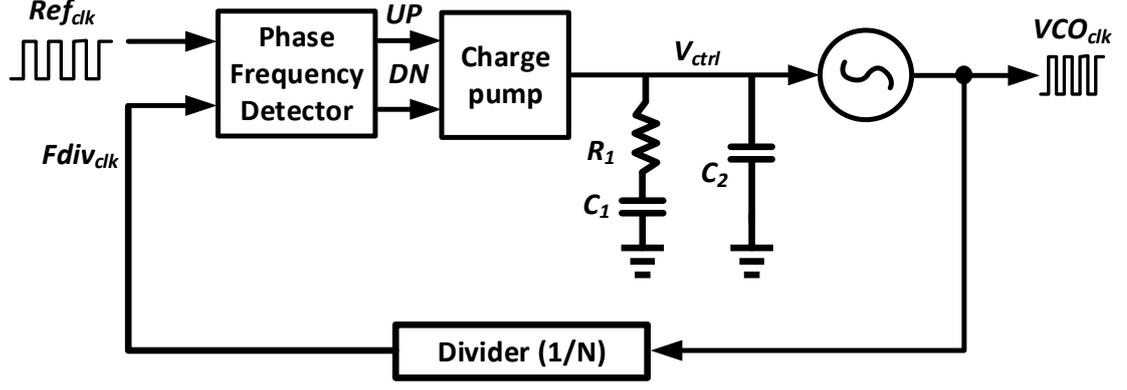
Figure 2.3: Block diagram of a type-II third order charge pump PLL
