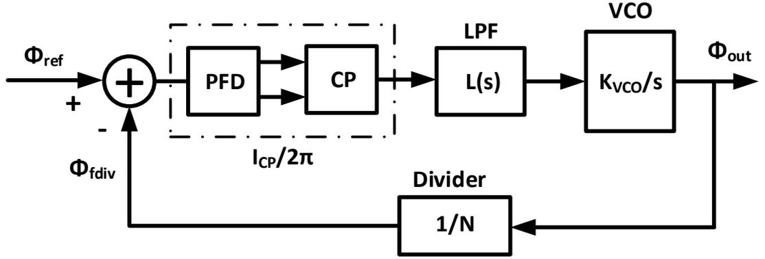
Figure 2.4: Linear Model of the Charge Pump PLL
