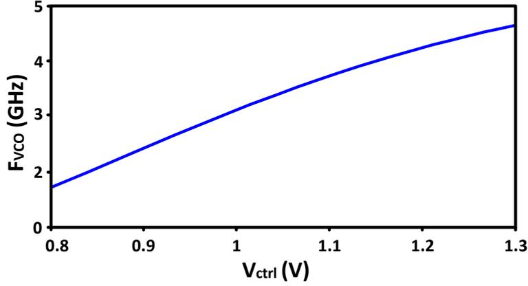
Figure 7.3: Output frequency of VCO as a function of control voltage
