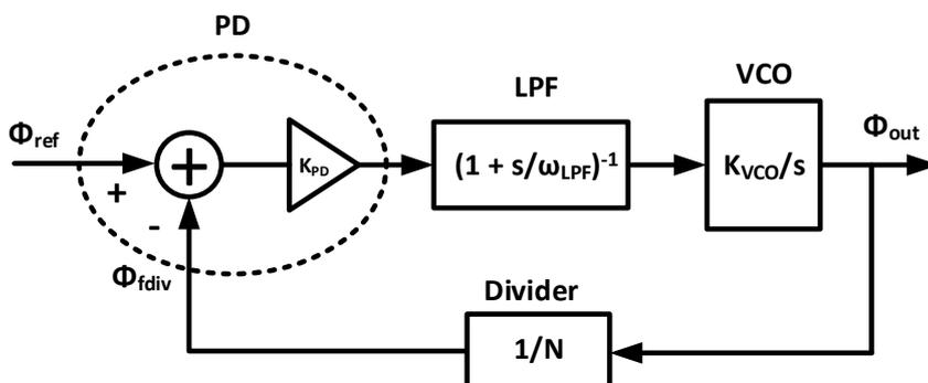
Figure 2.2: Block diagram of the type-I PLL's linear model
