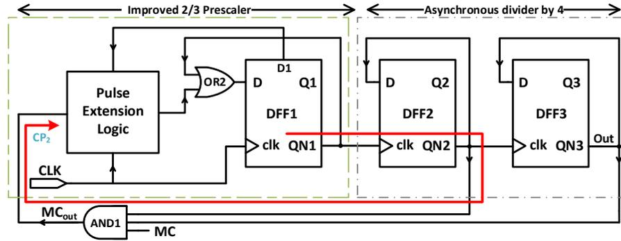
**Figure 3.7:** Block diagram of the proposed 8/9 prescaler
