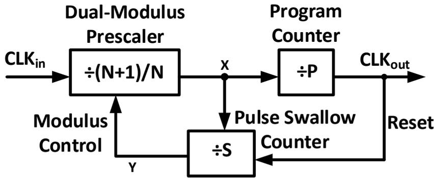
Figure 4.3: Pulse Swallow Counter based frequency divider
