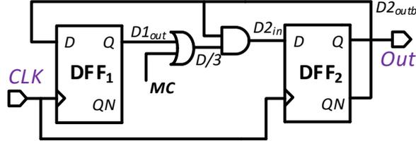
**Figure 3.1:** Block diagram of a conventional synchronous 2/3 prescaler
