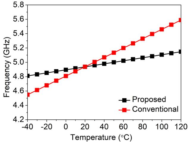
**Figure 5.10:** Variation of oscillation frequency with temperature
