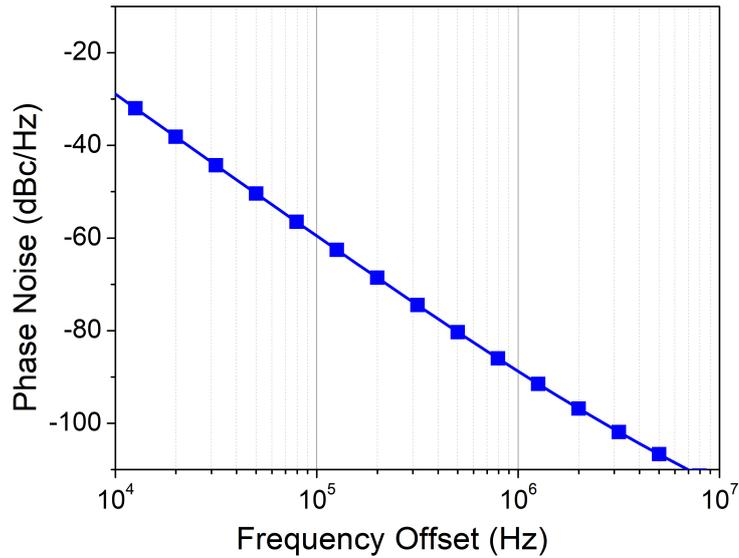
**Figure 5.13:** Phase Noise plot of the 4-stage VCO
