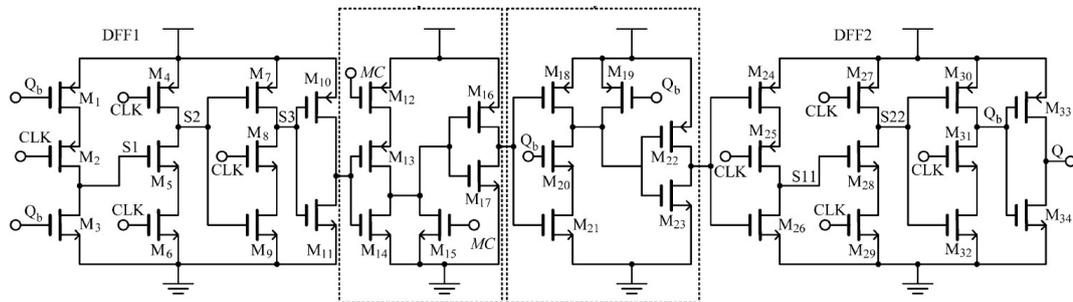
**Figure 3.3:** Gate level schematic of conventional 2/3 prescaler
