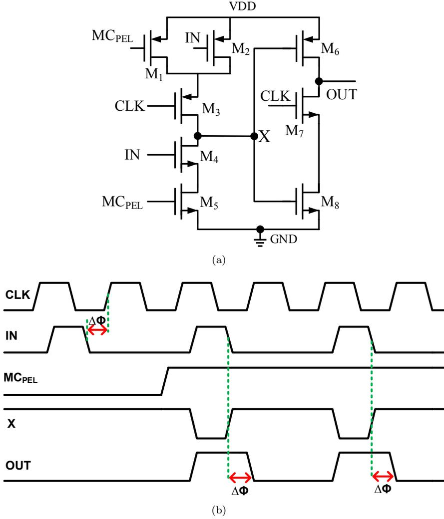
**Figure 3.8:** (a) Pulse Extension Logic circuit (b) Timing waveform of the Pulse Extension Logic
