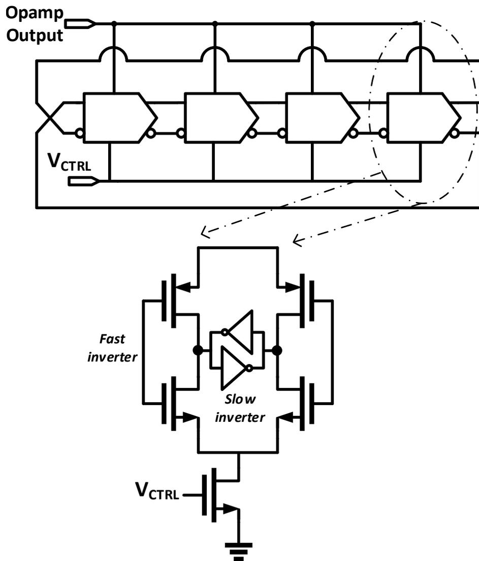
Figure 5.7: Schematic of the differential ring oscillator
