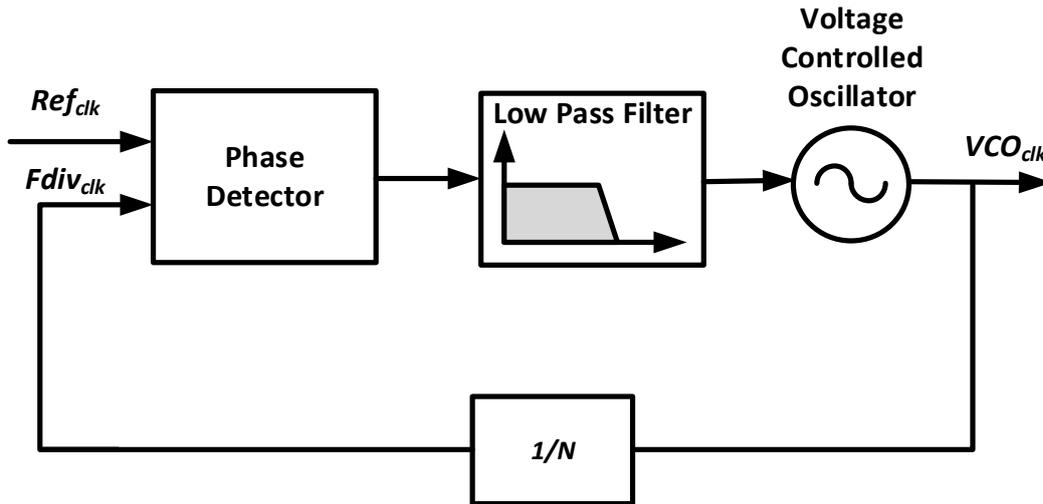
Figure 2.1: Block diagram of a basic Phase Locked Loop
