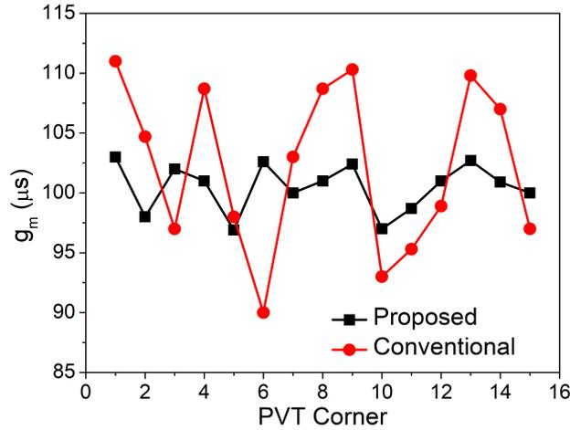
**Figure 5.9:** Inverter  $g_m$  of conventional and proposed technique
