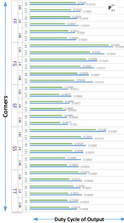
**Figure 4.15:** Output duty cycle of the proposed prescaler when Piv = 2 and 3
