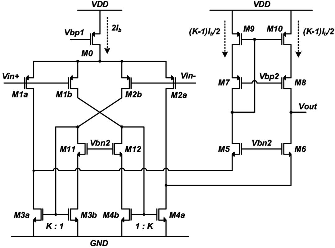
Figure 6.1: PMOS input folded Cascode Opamp proposed in [122]
