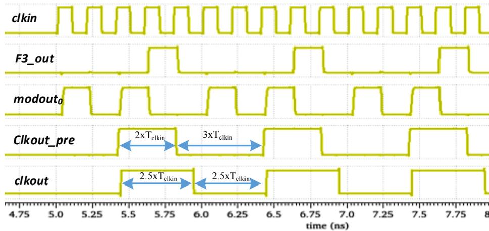
Figure 4.10: Timing waveform during divide-by-5 operation at 5 GHz input frequency
