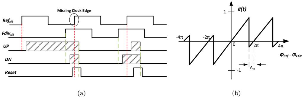
**Figure 2.8:** (a) Rising edge of  $Ref_{clk}$  being missed by PFD (b) blindzone in a PFD
