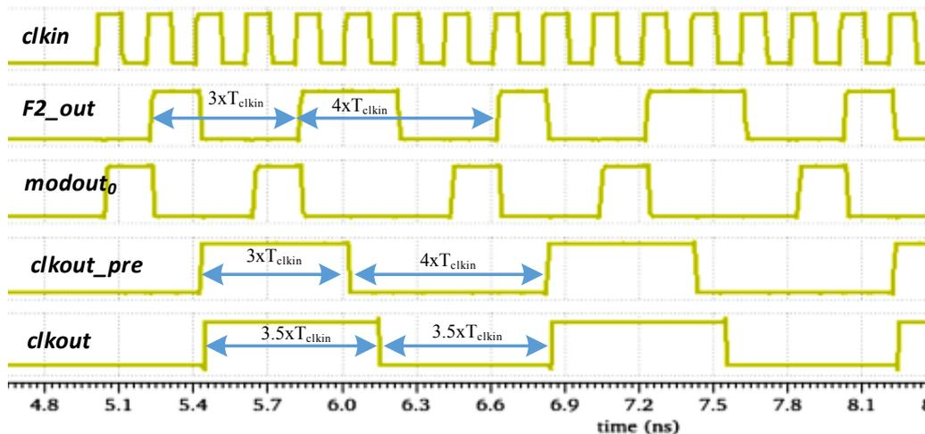
Figure 4.12: Timing waveform during divide-by-7 operation at 5 GHz input frequency
