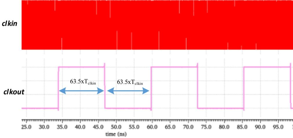
**Figure 4.13:** Timing waveform during divide-by-127 operation at 5 GHz input frequency
