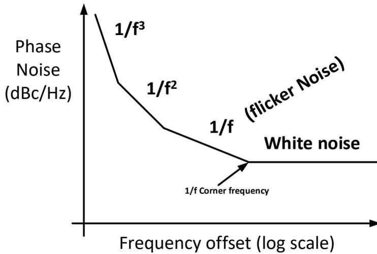
**Figure 2.19:** Oscillator's phase noise
