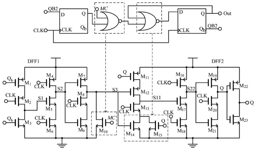
**Figure 3.4:** Gate level schematic of 2/3 prescaler proposed in [49]
