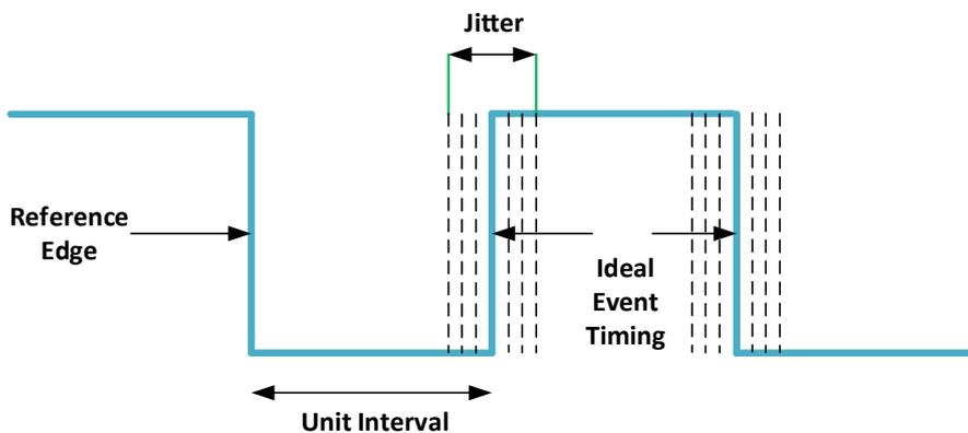
**Figure 2.20:** Deviation of a clock signal from its ideal position
