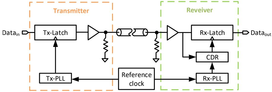
Figure 1.2: Typical serial link transceiver
