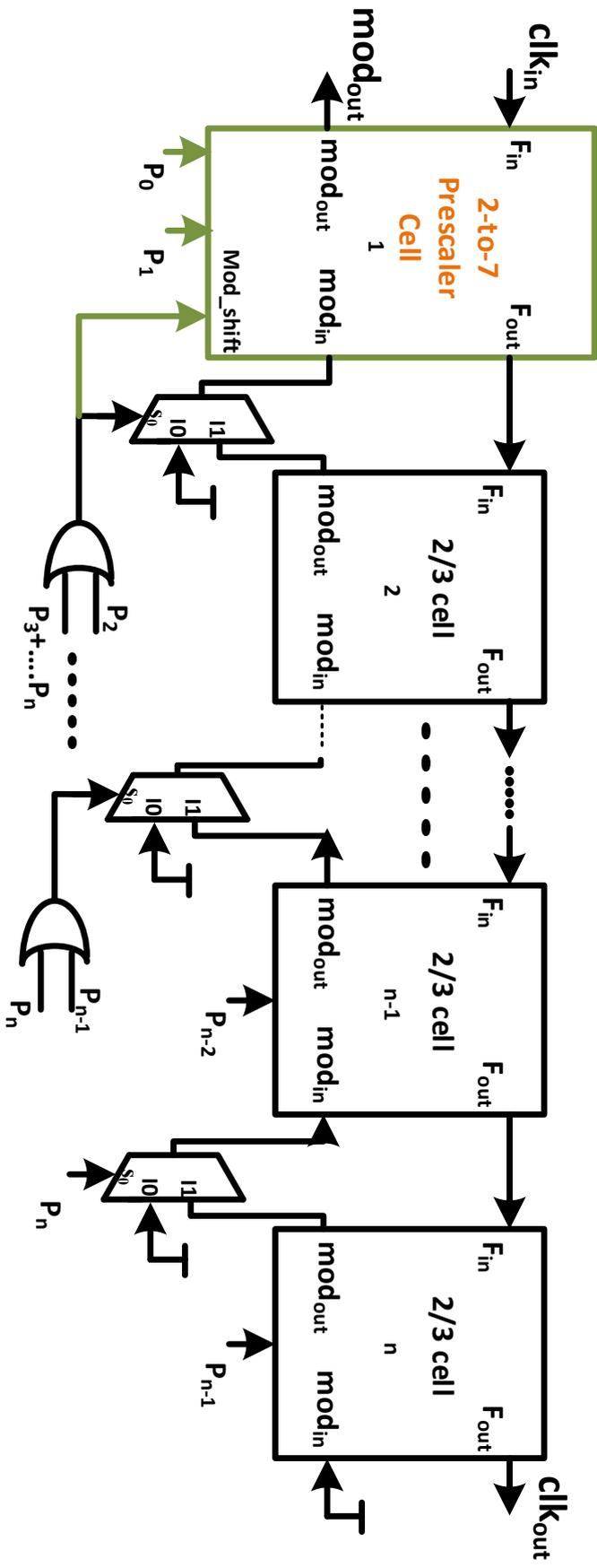
Figure 4.5: Proposed frequency divider's block diagram consisting of a novel 2-to-7 modulus prescaler
