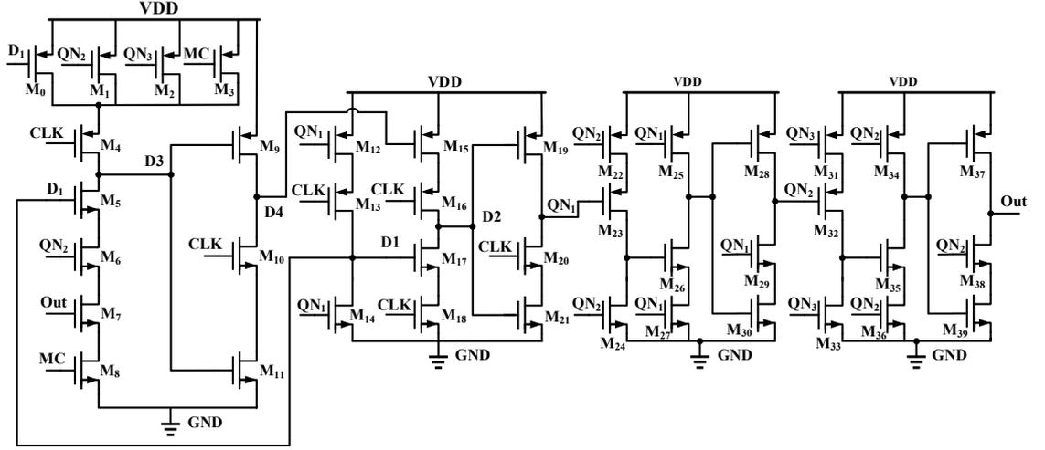
**Figure 3.9:** Transistor level architecture of the proposed 8/9 prescaler ( $L = 0.18\mu\text{m}$ )
