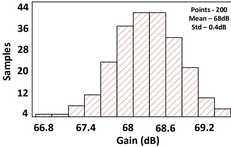
Figure 6.8: 200 point Histogram of the DC gain
