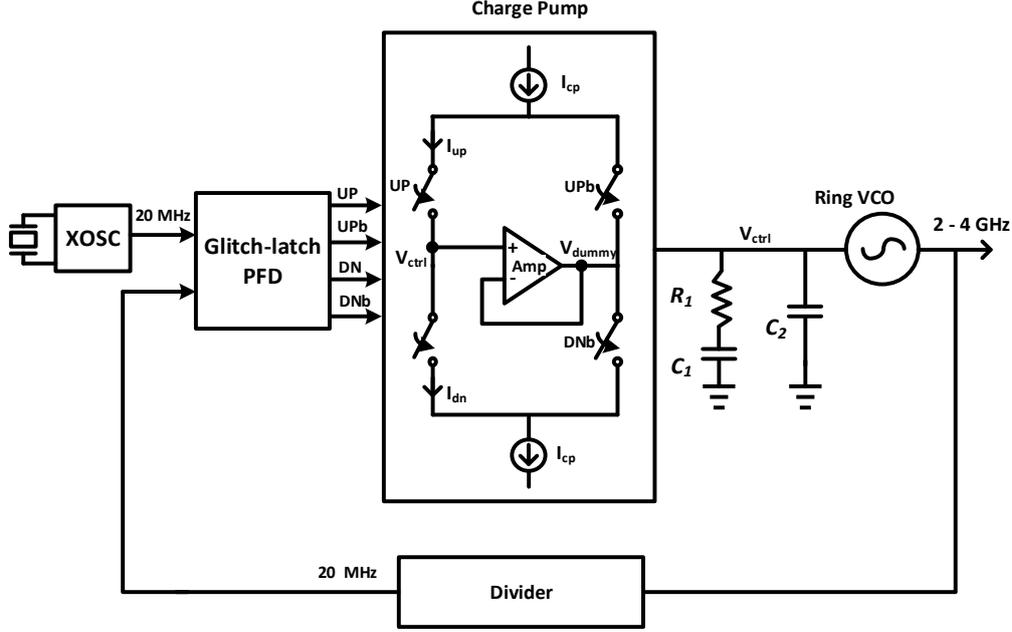
**Figure 7.1:** Top level block diagram of the implemented 2.4 GHz PLL
