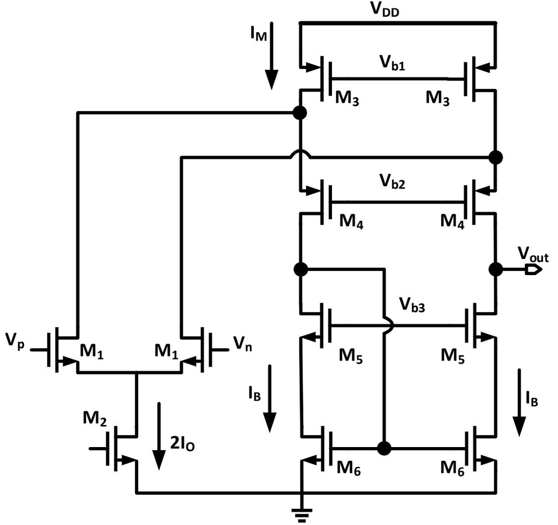
**Figure 6.2:** Conventional NMOS input folded Cascode Opamp
