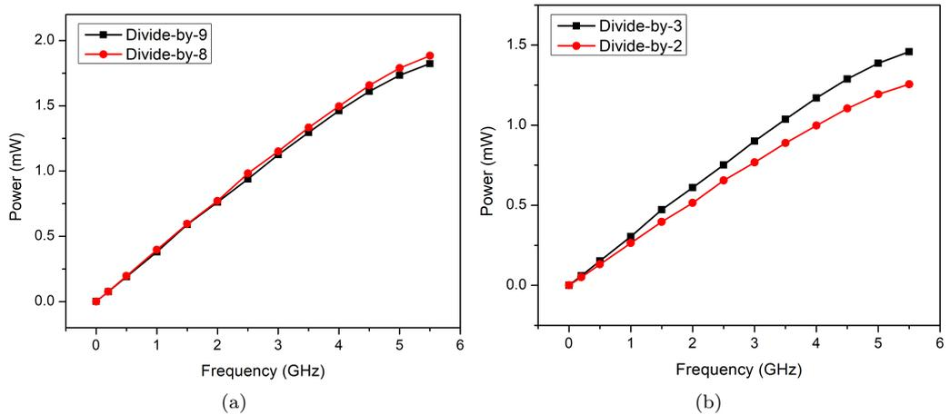
**Figure 3.13:** (a) Power vs frequency of the implemented 8/9 Prescaler (b) Power vs frequency of the proposed 2/3 Prescaler
