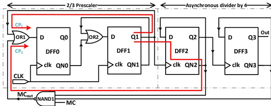
Figure 3.6: Block diagram of the conventional 8/9 prescaler
