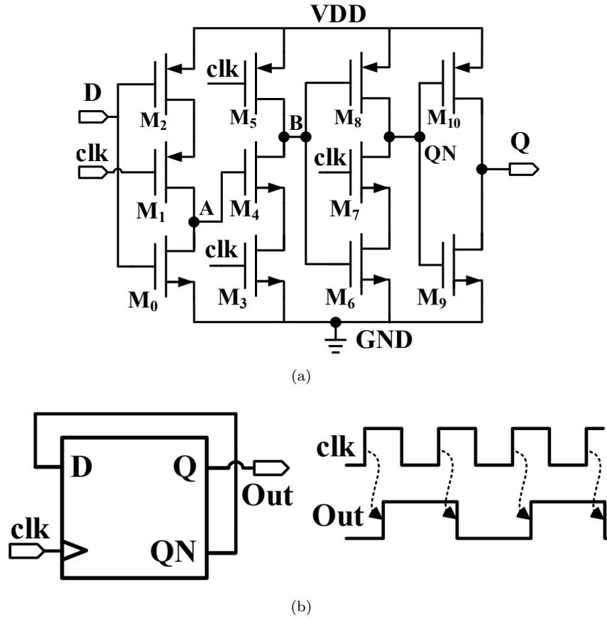
**Figure 2.18:** (a) TSPC flip flop (b) Divide-by-2 operation
