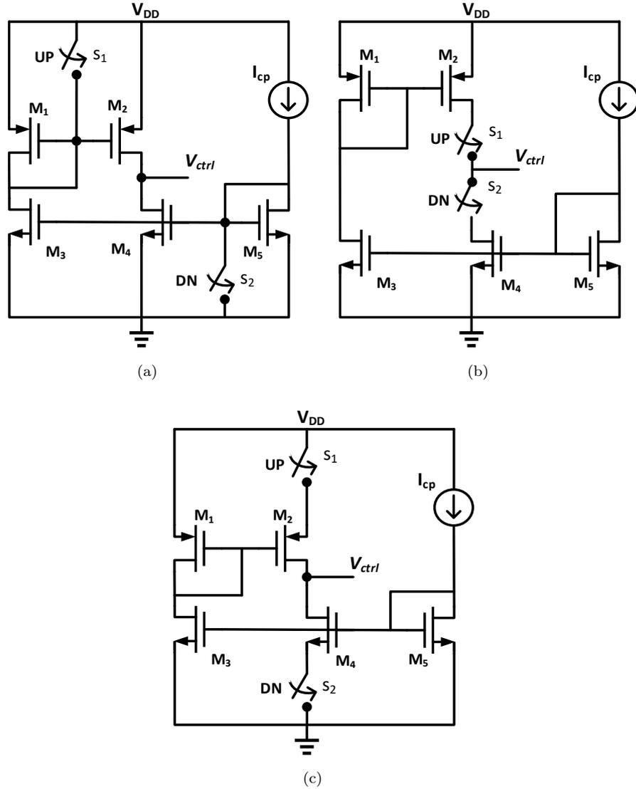
**Figure 2.10:** (a) Gate-switched charge pump (b) Drain-switched charge pump (c) Source-switched charge pump
