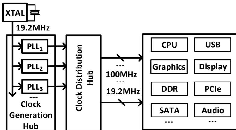
**Figure 1.1:** Clock generation and distribution in typical SoC with single crystal (XTAL)
