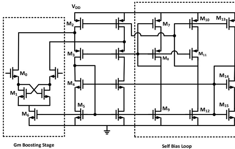
**Figure 5.8:** Schematic of the folded cascode Opamp used in proposed technique
