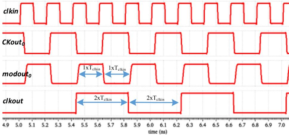
Figure 4.9: Timing waveform during divide-by-4 operation at 5 GHz input frequency
