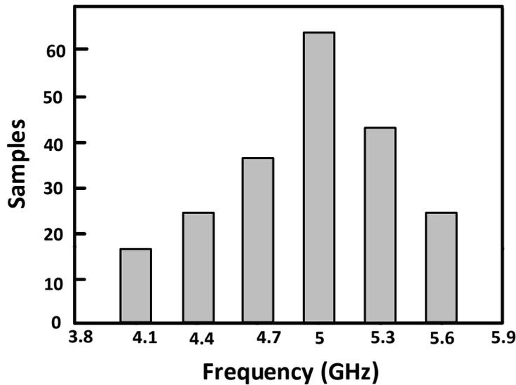
Figure 5.12: Output Frequency Histogram of the 4-stage VCO
