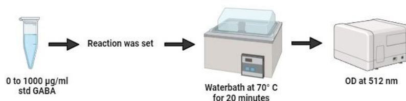
Fig. 4.3. Quantitative detection of GABA using UV-Vis spectrophotometry
