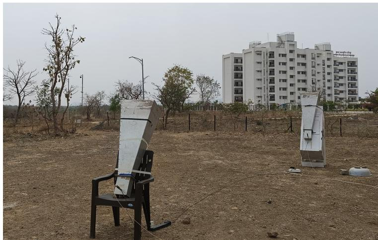
Figure 5.11: Setup of a Two-Element Interferometer with Horn Antennas
