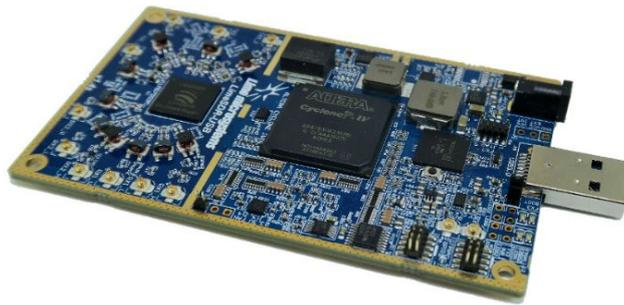
Figure 3.3: LimeSDR-USB Development Board [7]
