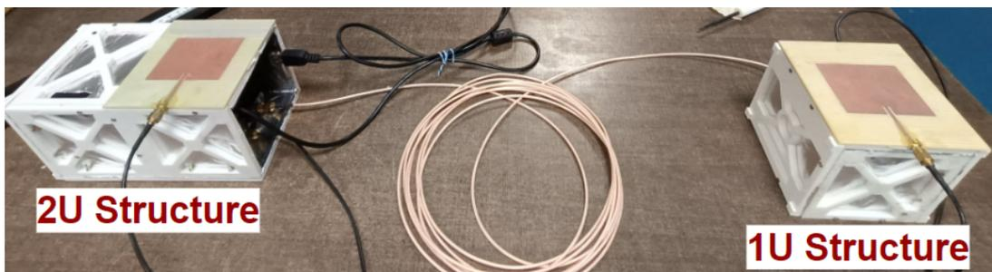
Figure 5.13: Test setup using patch housed by 3D printed CubeSat structure
