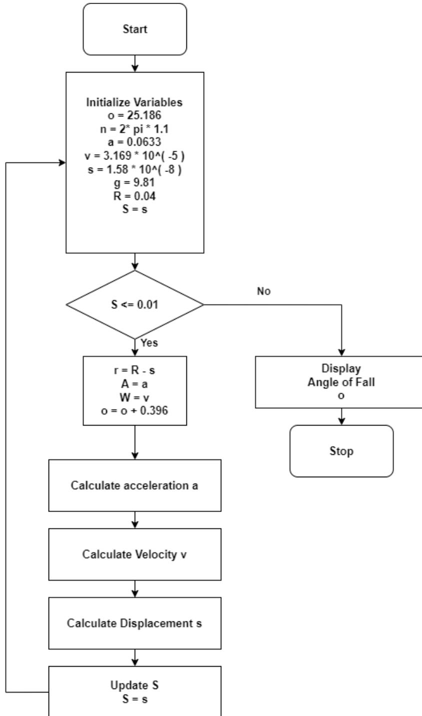
Figure 3.16: Flowchart For Determining the Threshold Speed of Motor
