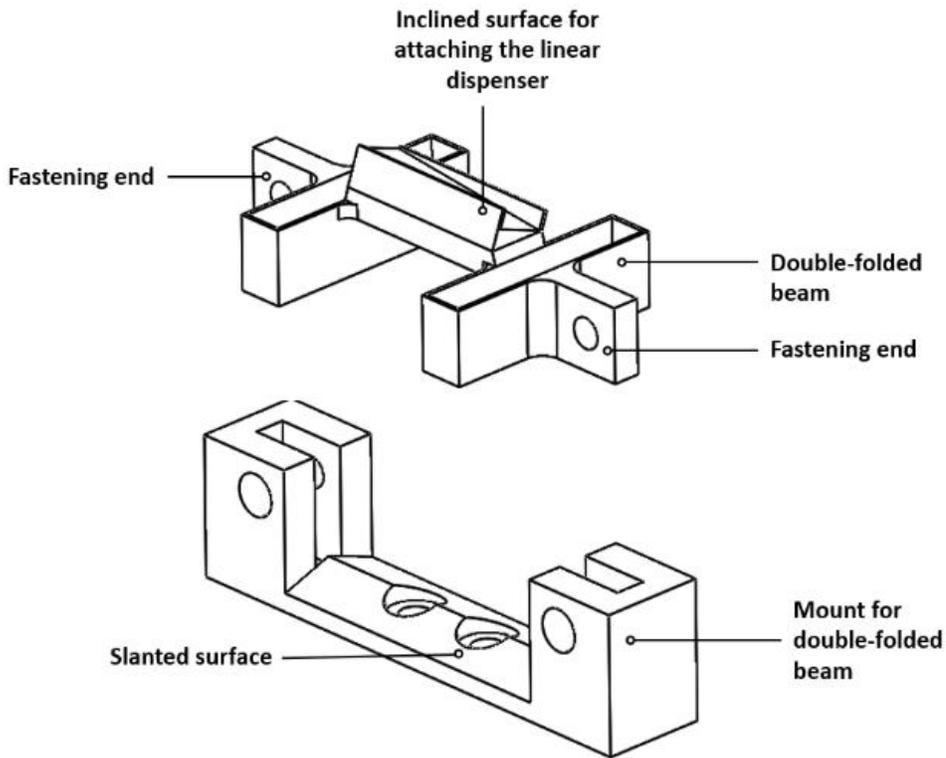
Figure 3.11: Isometric View of Double-Folded Beam
