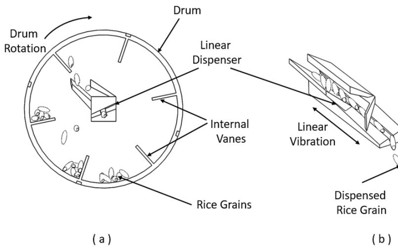
Figure 3.2: Concept Diagram of Modified Drum Feeder
