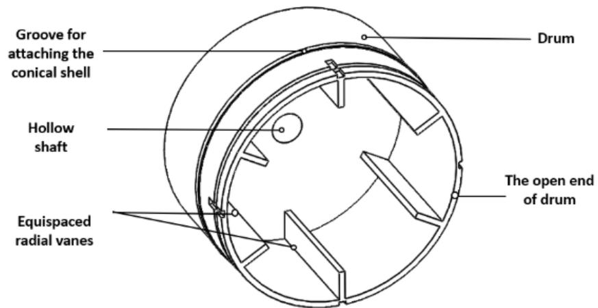
Figure 3.12: Isometric View of Rotary Drum
