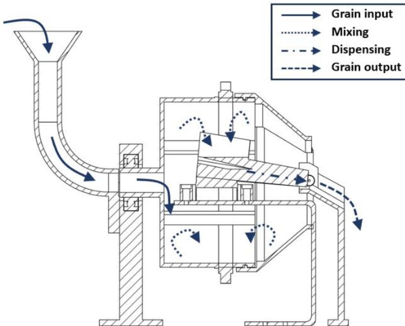
Figure 3.8: Movement of Grains within the Dispensing System
