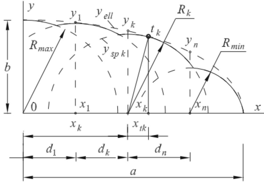
Figure 3.4: Multi-sphere model of ellipsoidal element (section geometry)
