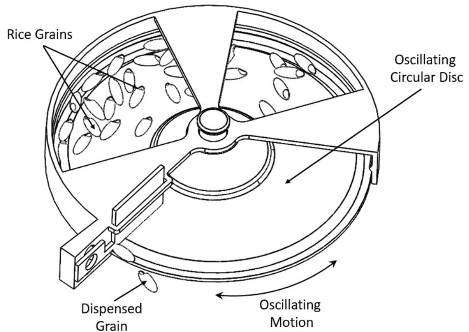
Figure 3.3: Concept Diagram of Oscillatory Feeder
