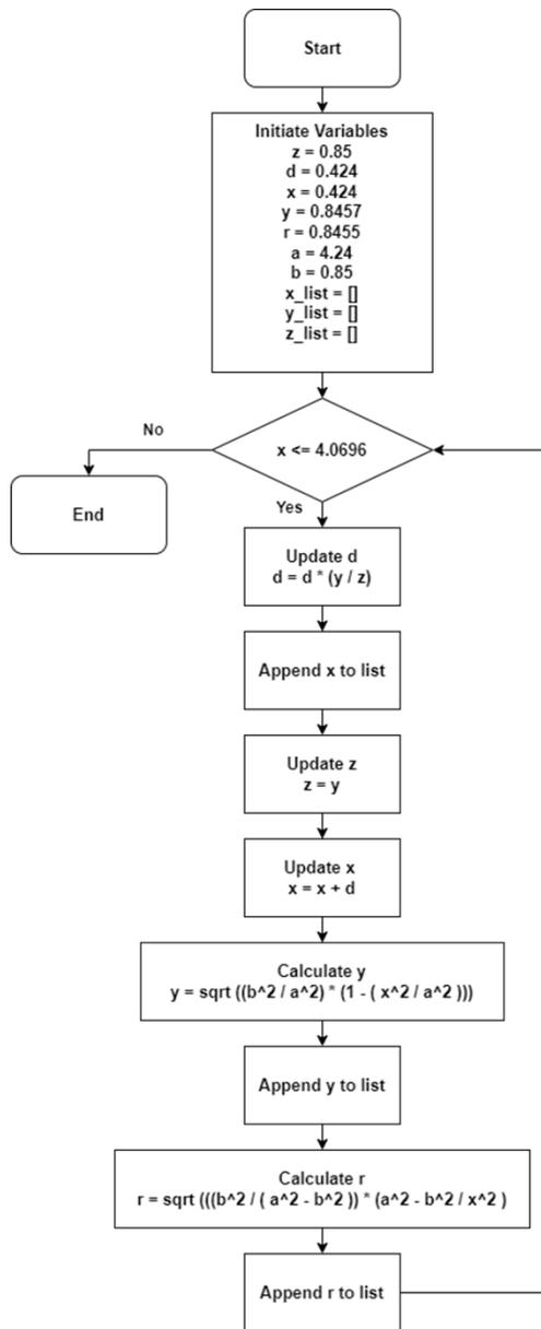
Figure 3.5: Flowchart For determining the position and dimensions of spheres in the ellipsoidal element
