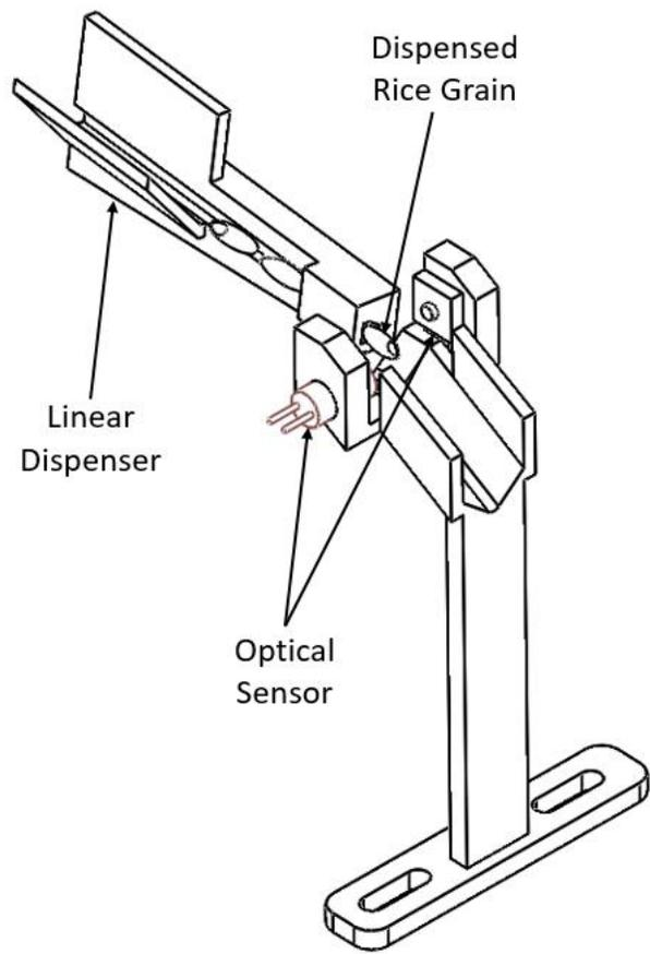
Figure 3.18: Working of Sensing System
