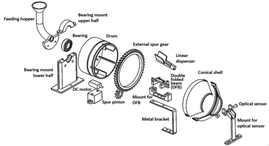
Figure 8.1: Exploded View of Dispensing System
