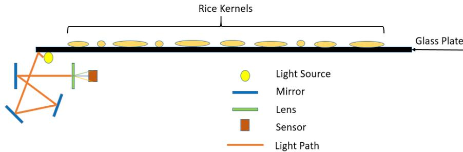
Figure 2.1: Cross Section of a Flatbed Scanner Used for Scanning Rice Kernels
