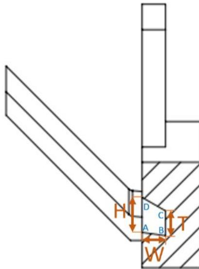
Figure 3.10: Cross-Sectional View of Linear Dispenser Showing Pathway Dimensions
