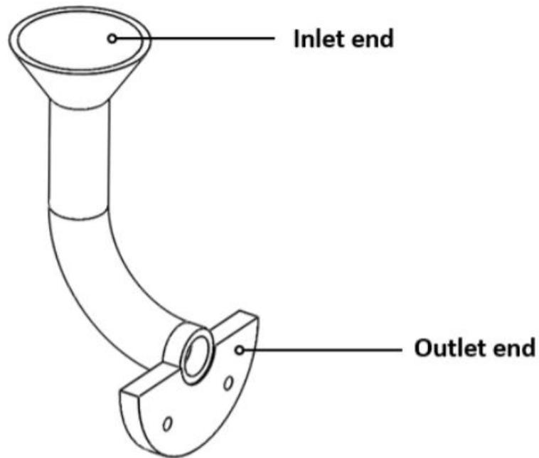
Figure 3.14: Isometric View of Feeding Hopper
