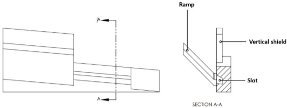
Figure 3.9: Cross-Sectional View of Linear Dispenser
