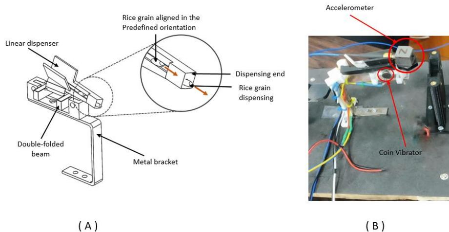
Figure 5.1: Experimental Setup to Determine the Frequency and Amplitude of Vibration of the Linear Dispenser
