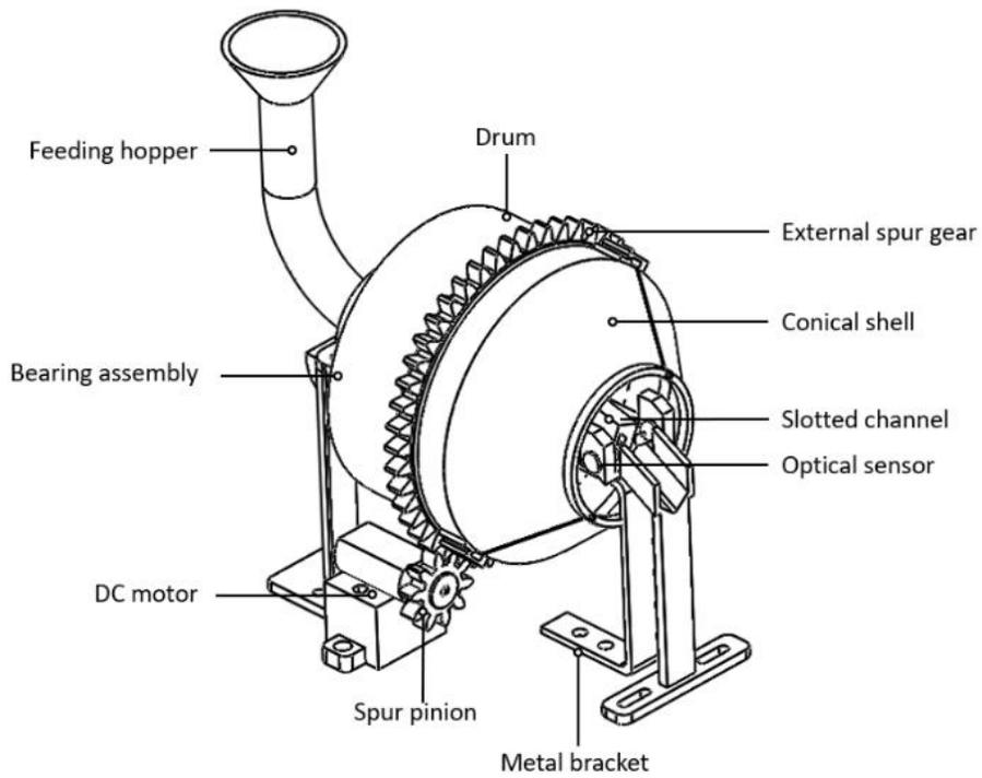
Figure 3.7: Isometric View of Dispensing System
