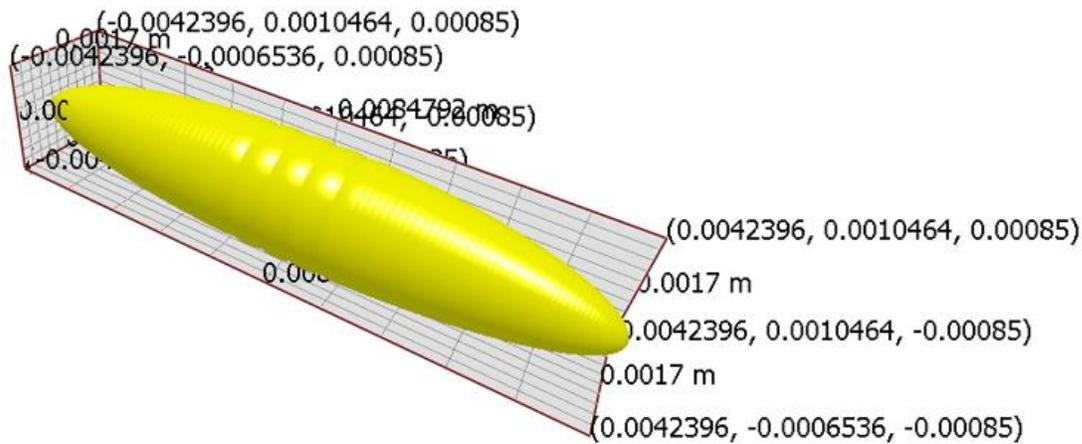
Figure 3.6: EDEM Particle Model of Rice Grain
