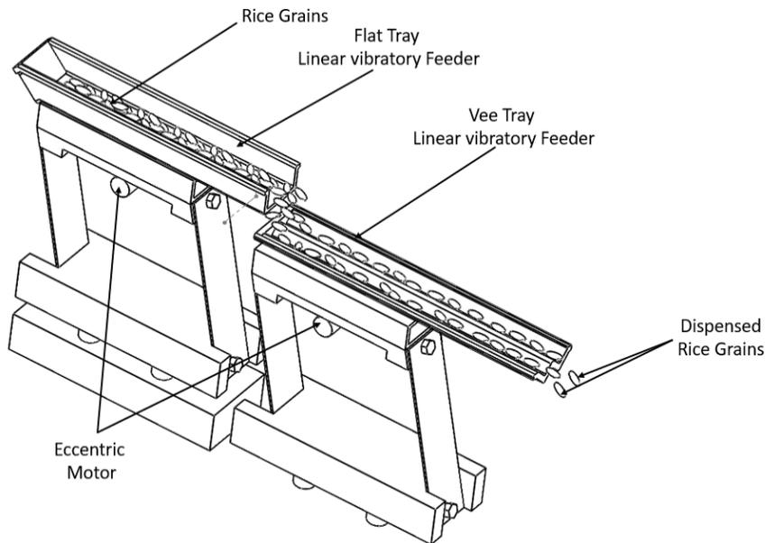
Figure 3.1: Concept Diagram of Dual Linear Vibratory Feeder
