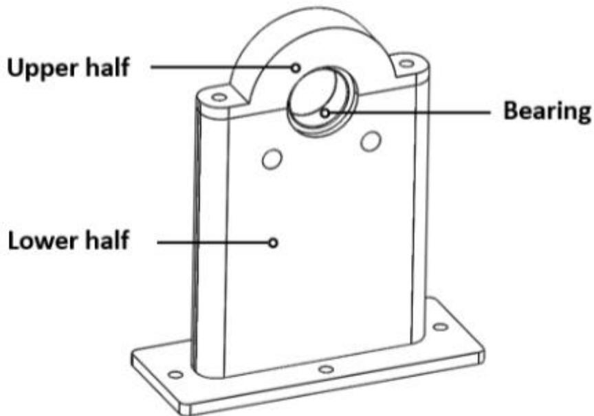
Figure 3.13: Isometric View of Bearing Mounting Assembly
