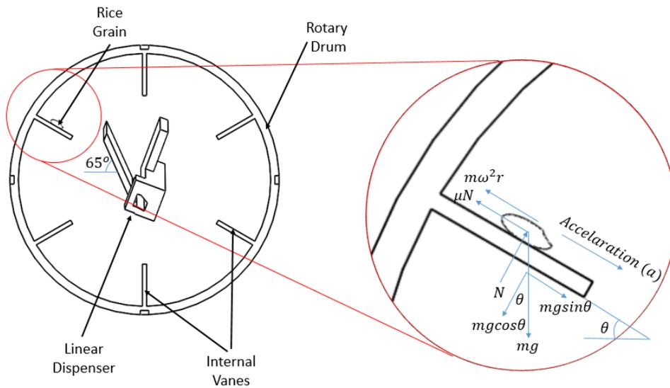
Figure 3.15: Free Body Diagram of A single Rice grain
