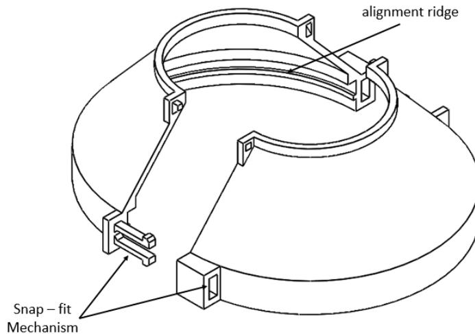
Figure 3.17: Isometric View of Conical Shell
