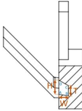
Figure 5.3: Cross-Sectional View of Linear Dispenser Showing Pathway Dimensions
