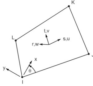
Figure 3.3 4-noded Shell element.
