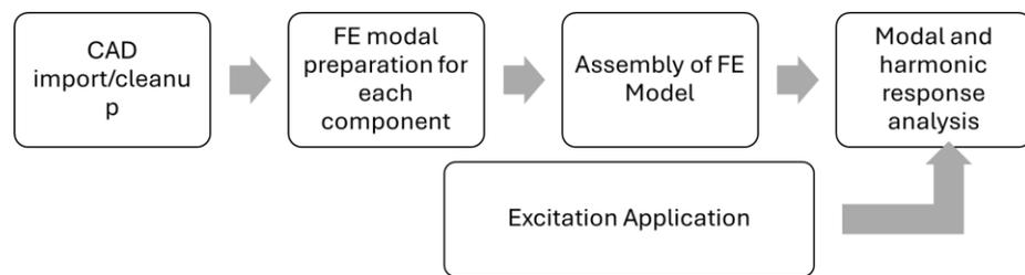
*Figure 3.1 Schematic approach to model the engine for NVH analysis.*
