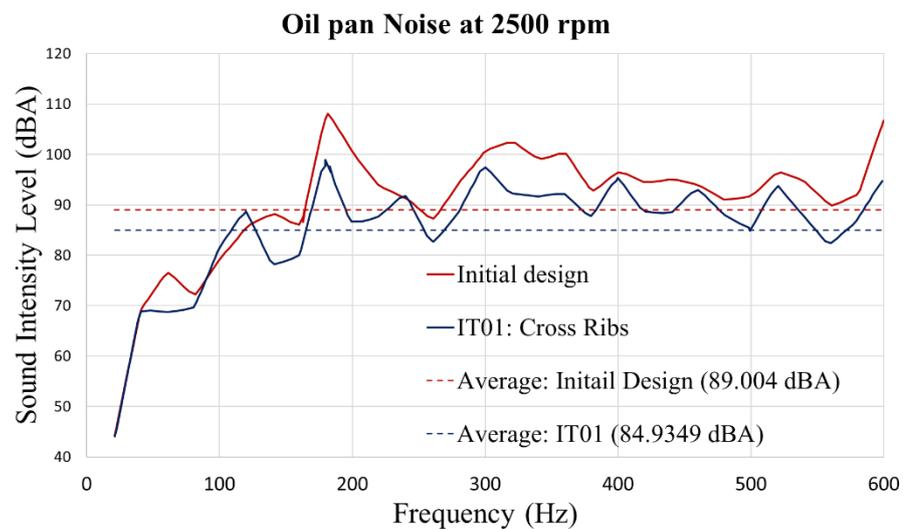
Figure 5.4 Comparison of noise level of oil pan for different design.
