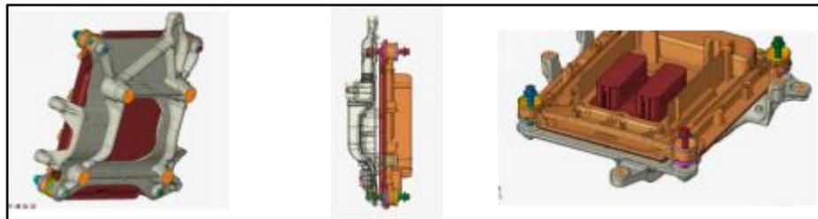
*Figure 3.11 Master nodes in the FE model (indicated by red nodes)*
