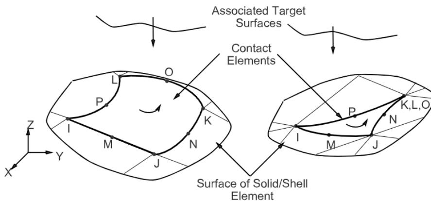
Figure 3.6 Contact Surfaces.
