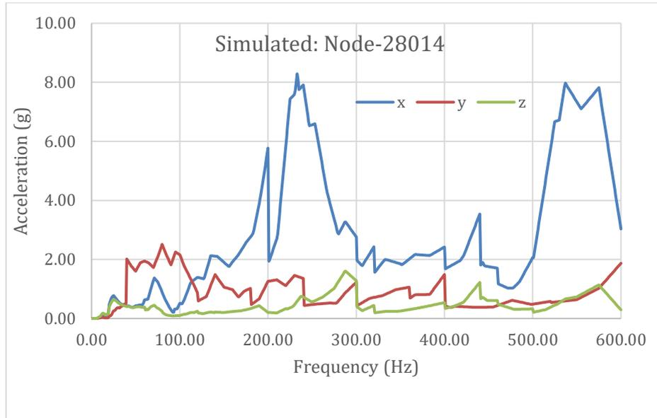
*Figure 4.5 Simulated vibration level at node 28014*
