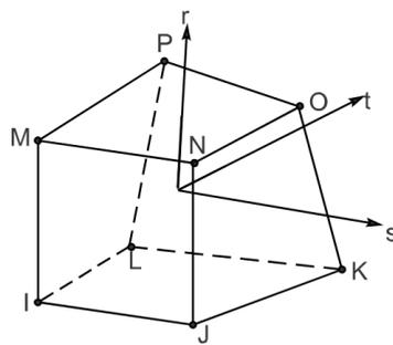
Figure 3.4 8-noded Solid element.
