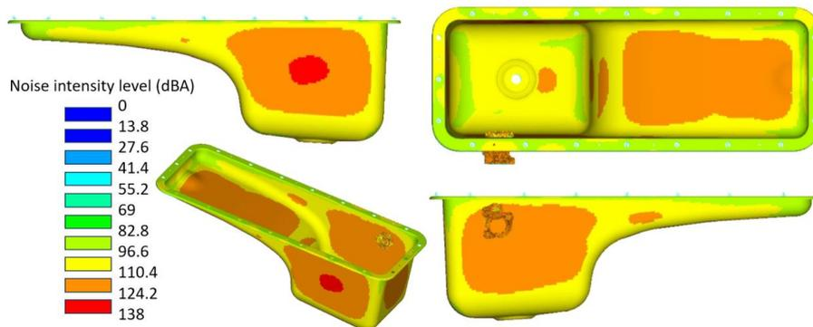
*Figure 5.1 Sound Intensity level (dBA) for the initial design.*
