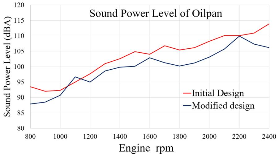
Figure 5.5 The sound Power level of the oil pan for the initial and modified design.
