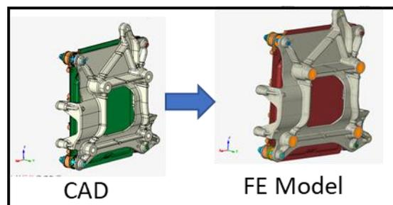
Figure 3.8 Imported CAD model of ECU and its FE model.
