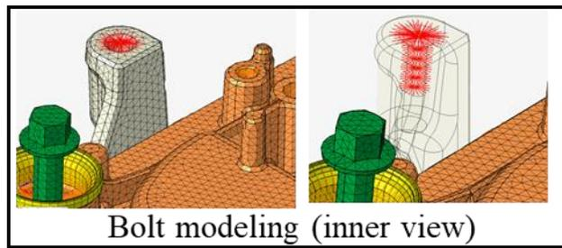
*Figure 3.9 Bolt modeling for FE model.*
