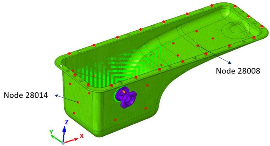
Figure 4.2 Oil Pan and its vibration measurement locations
