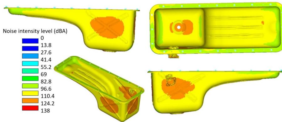
*Figure 5.2 Sound Intensity level (dBA) for Iteration 01*
