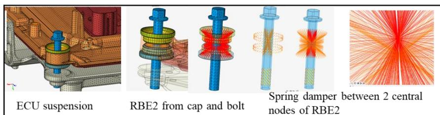
*Figure 3.10 Isolation System modeling for ECU*
