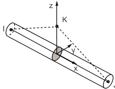
Figure 3.5 2-noded beam element.
