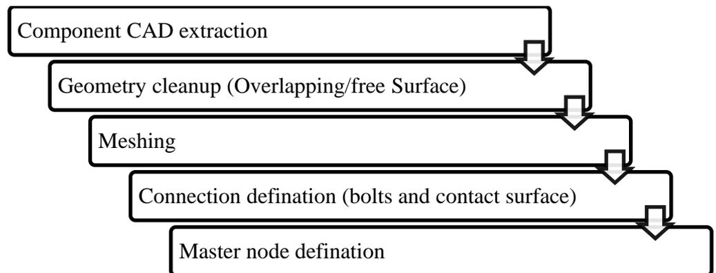
Figure 3.7 Schematic approach to generate FE model.
