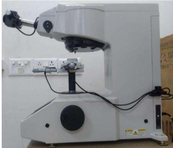
*Figure 18 Micro Hardness Tester Mitutoyo, (HM-210)*
