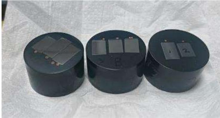
*Figure 15 Samples were hot mounted for Cross-sectional analysis*
