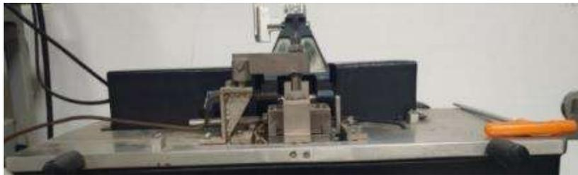
*Figure 20 Sliding Wear test machine*
