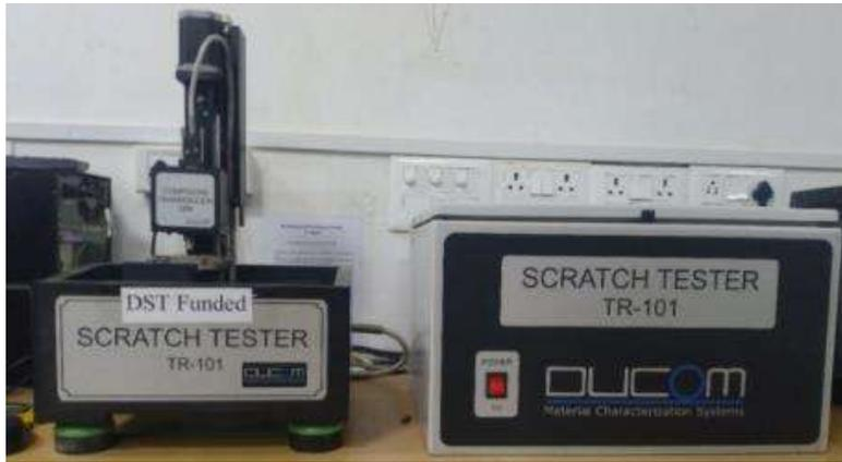
*Figure 19 Scratch Tester DUCOM (TR-101).*
