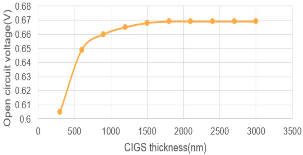
4.6 Open circuit voltage versus CIGS thickness
