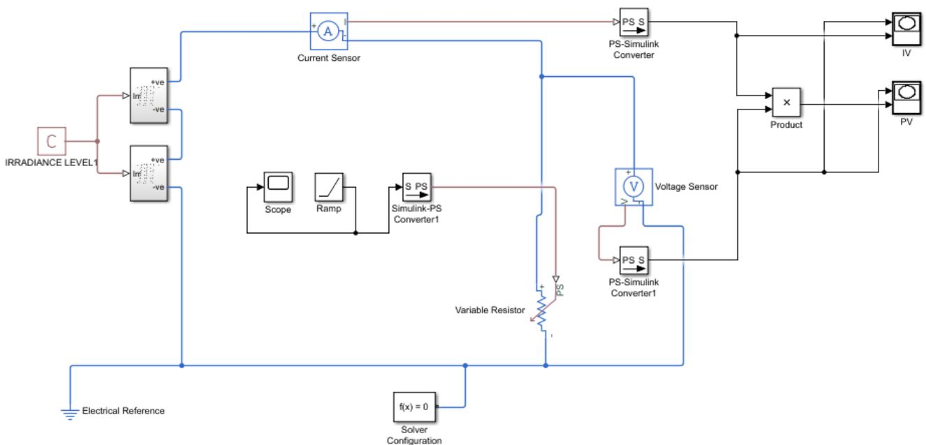
4.22 series connected solar cells
