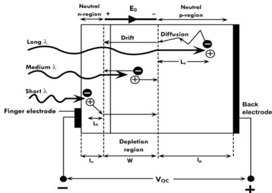
2.1 Principle of operation of a PN junction solar cell.
