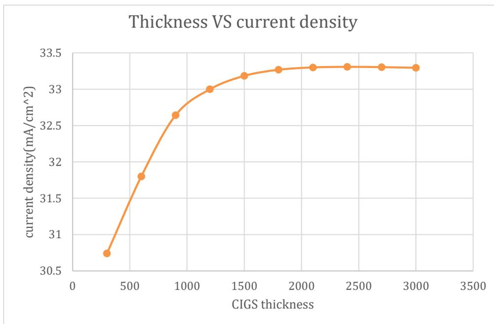
4.5 Short circuit current density versus CIGS thickness
