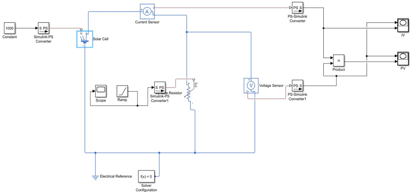
4.19 Single solar cell model in Simulink
