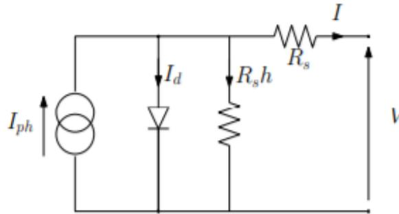
2.2 Equivalent electrical circuit of the single diode solar cell model.
