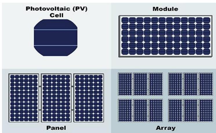
1.2 Photovoltaic cells, modules, panels and arrays
