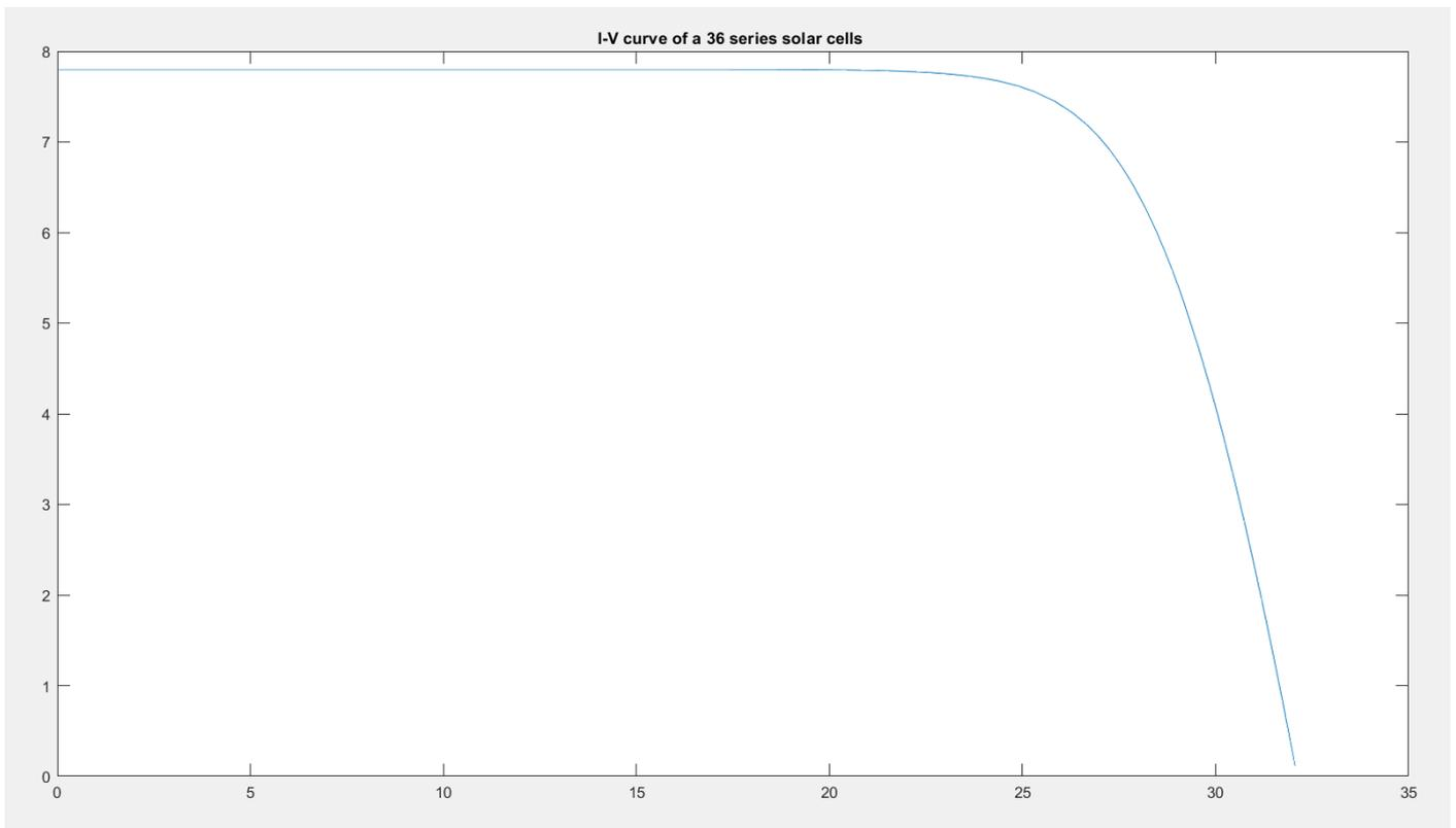
4.24 I-V curve for series connected cells
