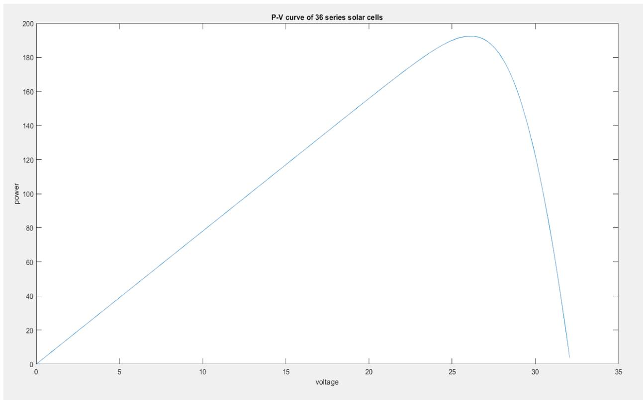
4.25 P-V curve for series connected cells
