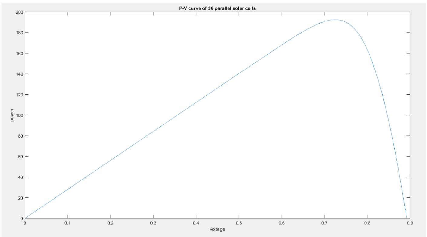
4.29 P-V Curve for parallel connected
