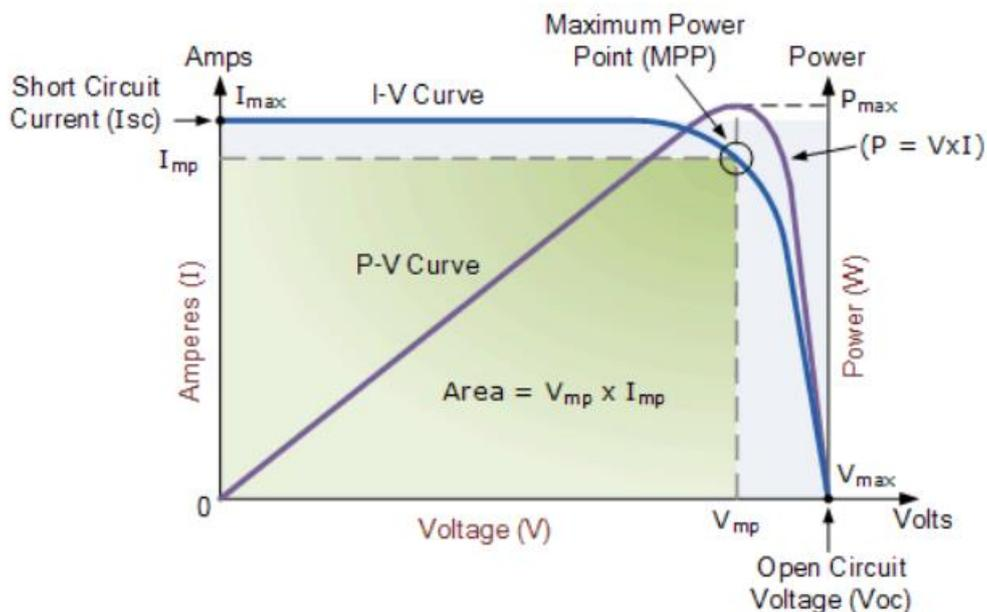
2.3 I-V and P-V characteristics of a solar cell
