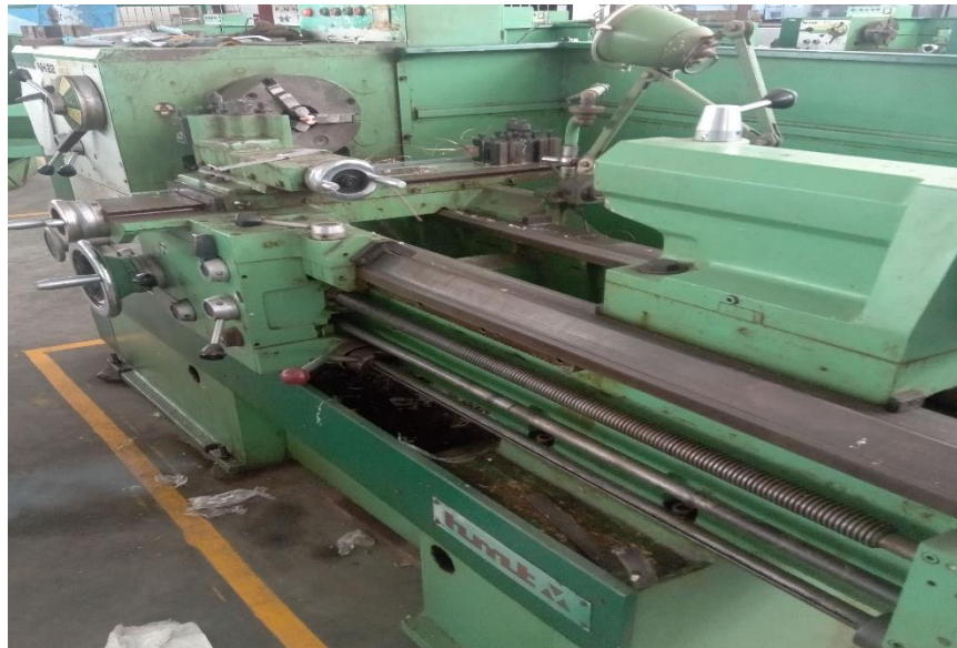
Figure 28 Lathe machine used to make electrode of Resistance Spot welding.
