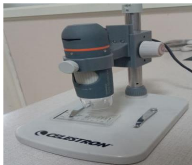
Figure 29 Digital microscope use to take image of cross-section
