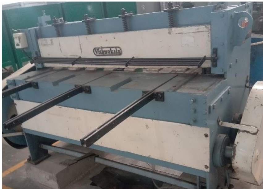
Figure 27 Shearing machine used to cut the sample to proper dimension
