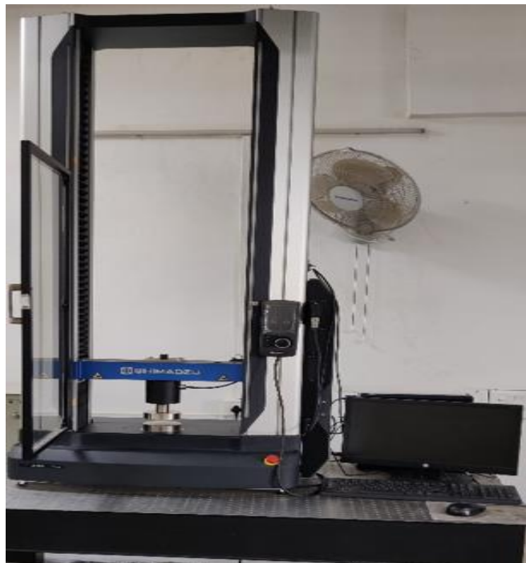
Figure 33 UTM machine of capacity 10kN was used for shear and peel test
