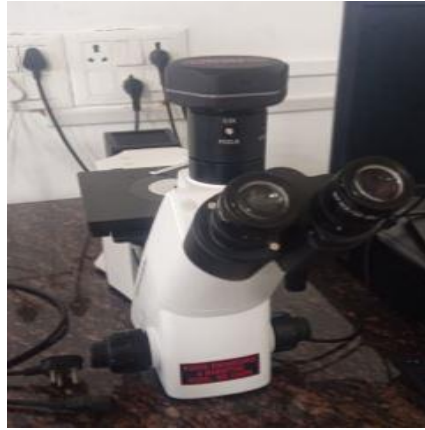
Figure 30 Optical microscope used to analyse grain structure
