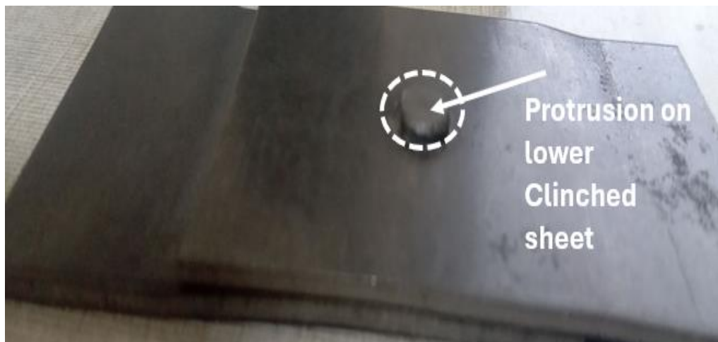
Figure 59 Protrusion on lower clinched sheet.
