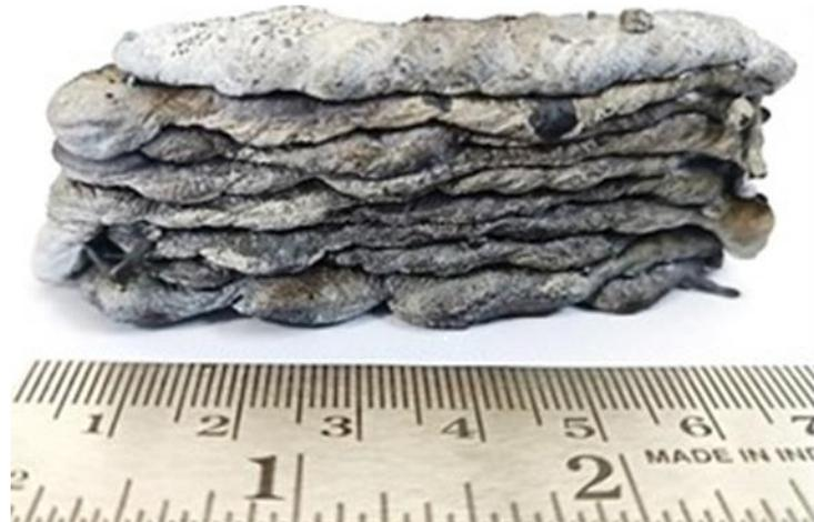
**Fig. 4.4:** Optimized multi-layer deposition of NiTi20Cu SMA fabricated by T-WAAM process.
