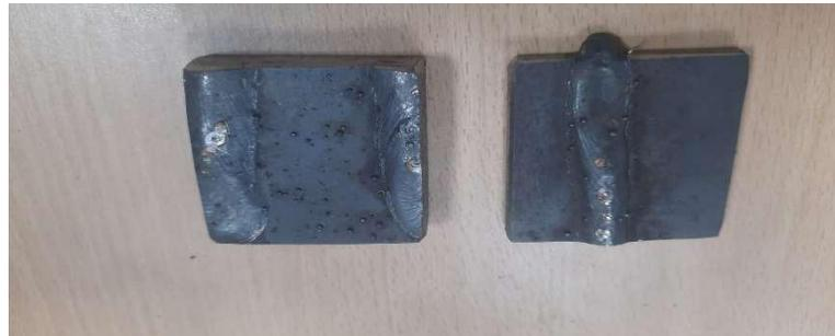
*Figure 7. Welded steel samples cut in specific dimensions suitable for the experiments*
