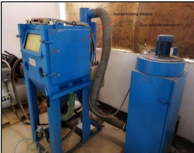
*Figure 6. Suction type blasting facility at IIT Indore*
