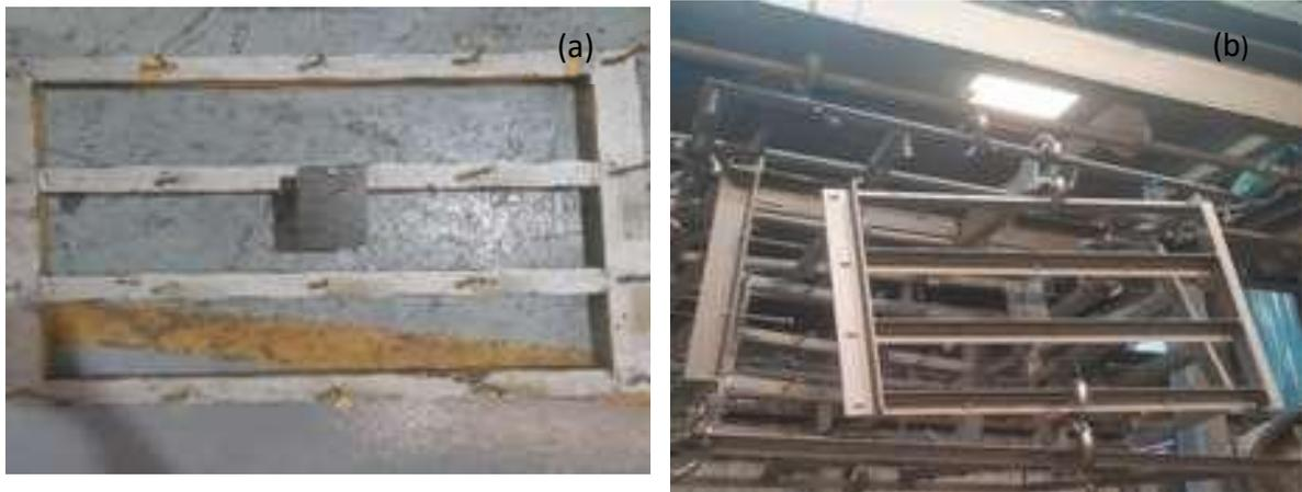
*Figure 9(a) and (b). Sample attached to the holder frame and Six holder frames hung from the conveyor shaft with the help of S-hooks*
