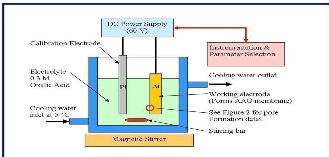
**Figure 9: Experimental setup of Aluminium anodization**
