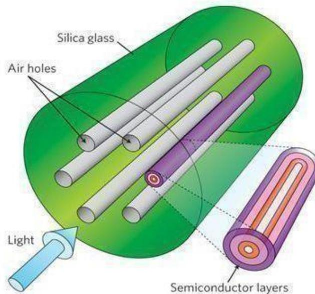
**Figure 7: Photonic crystal fibre**
