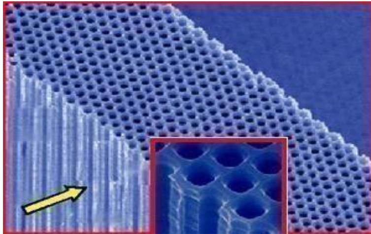
**Figure 3: (b) 2-D Photonic crystal (Nanopores in high refractive index slab)**
