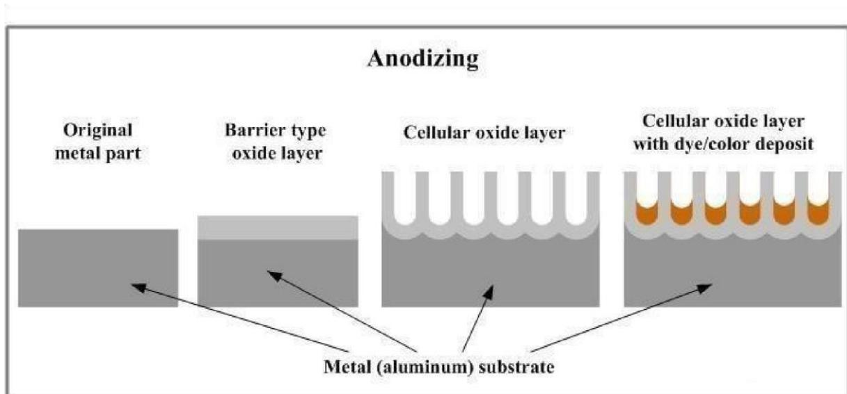
**Figure 8: Steps of Aluminium Anodization**
