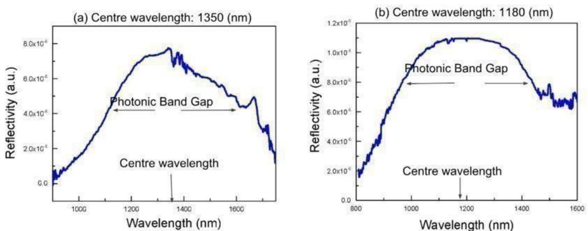
**Figure 11: Reflection characteristics of 2-D photonic crystal**
