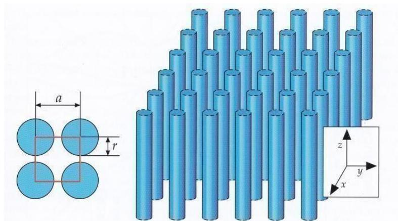
**Figure 3: (a) 2-D Photonic crystal (High refractive index rods in air)**
