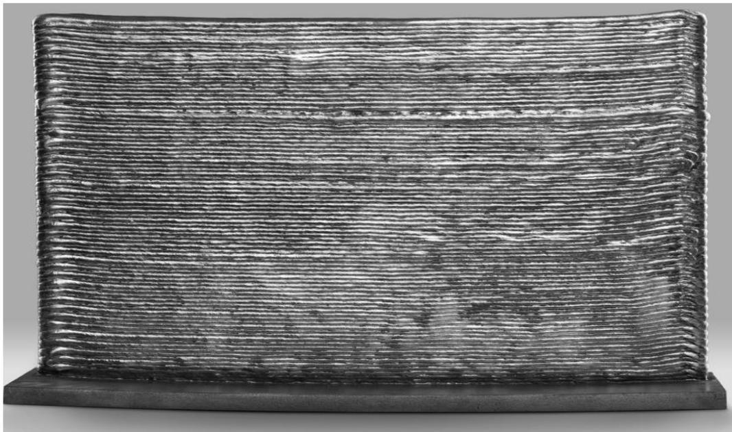
Figure 3:ER5356 Al alloy fabricated using WAAM setup
