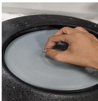
Figure 21: Polishing on #2500
