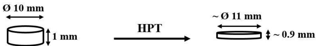
Figure 6.15: Dimensions of disk before and after HPT
