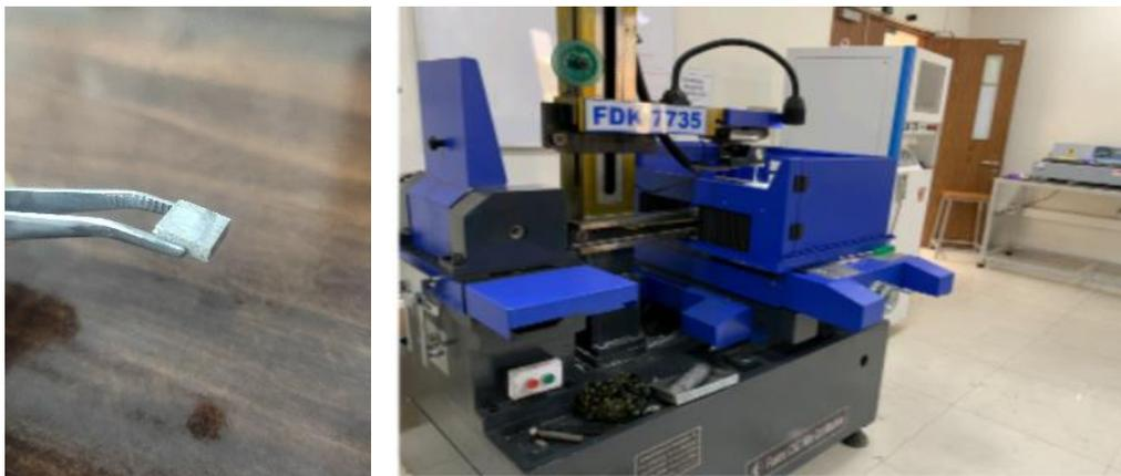
Figure 5.2: Cut Sample & FOSTEX FDK 7735 wires cutting EDM machine
