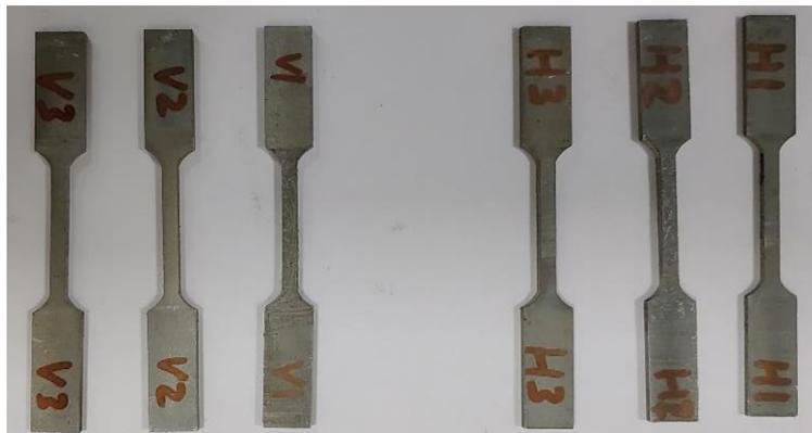
Figure 5.14: Tensile test specimens before testing
