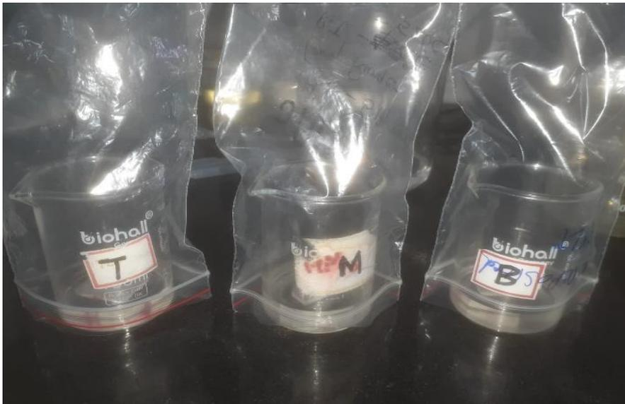
Figure 5.16: Immersed samples in nitric acid
