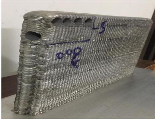
Figure 5.1: Wall manufactured by WAAM
