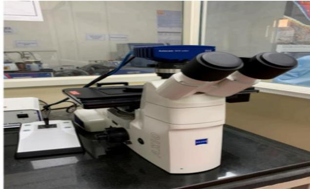
Figure 5.8: Zeiss Axiovert A1 inverted microscope
