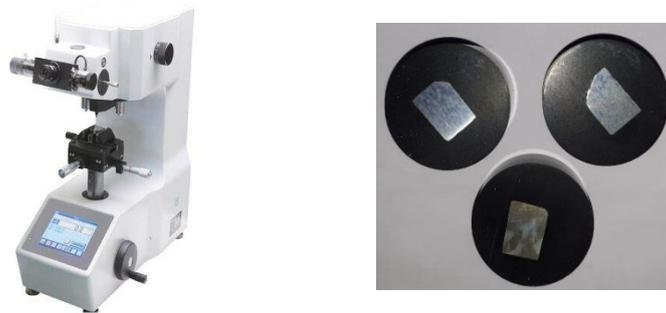
Figure 5.13: Hardness testing machine and samples
