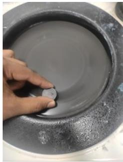
Figure 5.4: Grinding Operation
