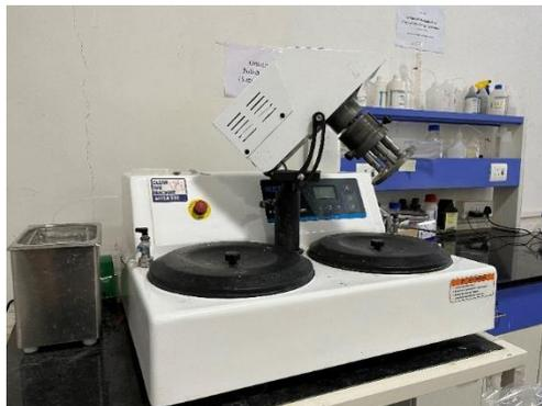
Figure 5.5: MetCo Bainpol Grinding/Polishing Machine
