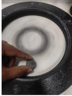
Figure 5.6: Polishing the Sample
