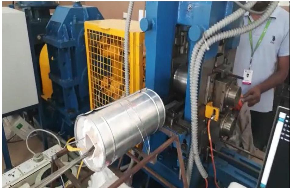
Fig 3.2: Experimental set-up of Hot Rolling Equipment
