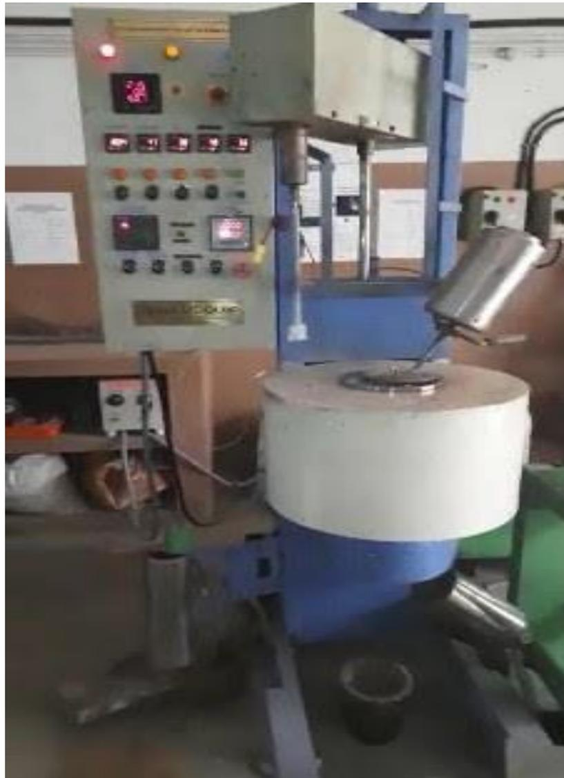
Fig 3.1: Experimental set-up of vacuum stir casting equipment
