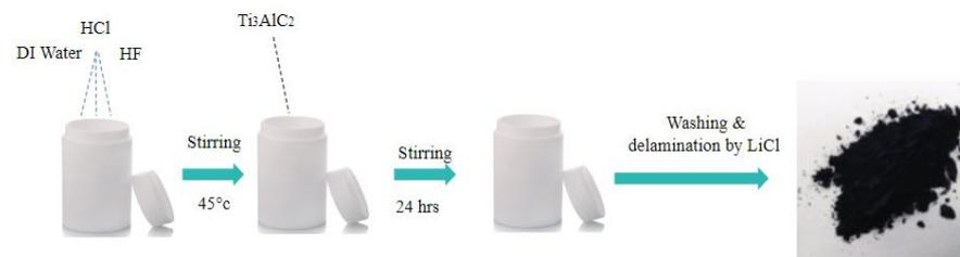
**Fig. 9.** Schematic diagram of the synthesis process of MXenes.
