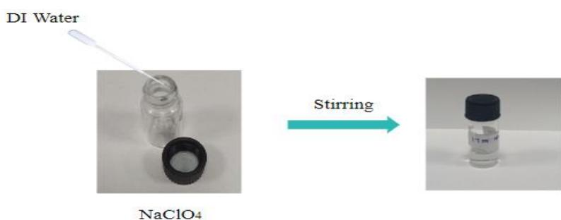
**Fig. 12.** Schematic diagram of the preparation process of electrolyte.
