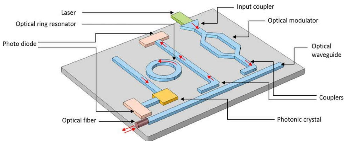
**Fig.1.1 Photonics components on a single chip**
