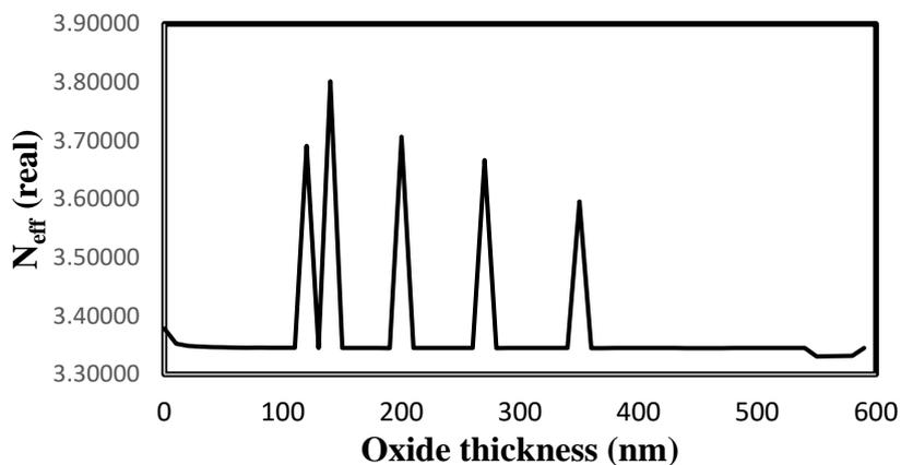
**Fig.3.2: Effective index (real) vs Oxide thickness**
