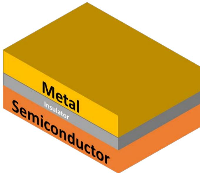
**Fig.3.1: Metal Insulator Semiconductor (MIS) structure**
