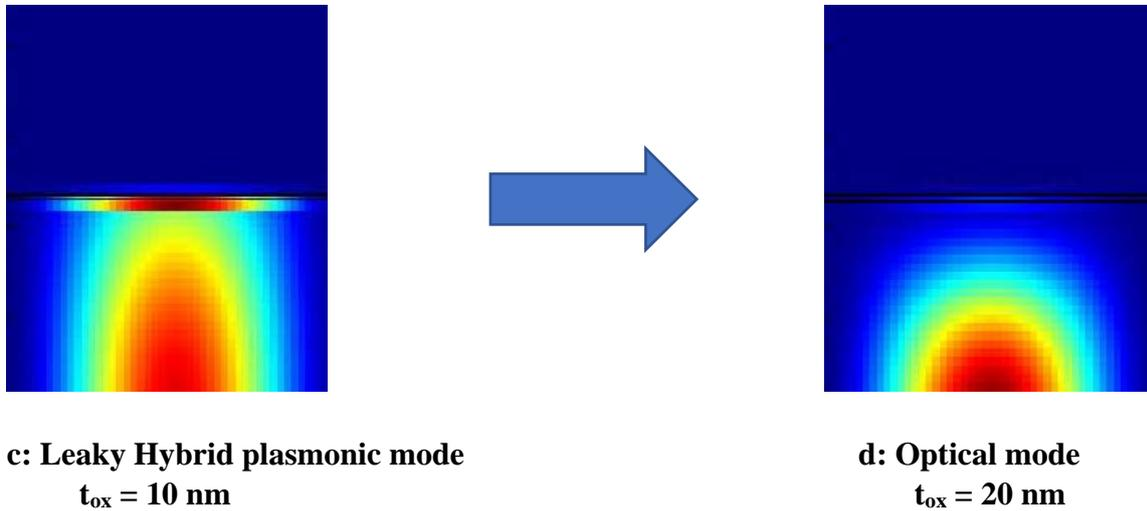
**Fig.3.4 (a,b,c,d): Transition of modes as per Oxide thickness**
