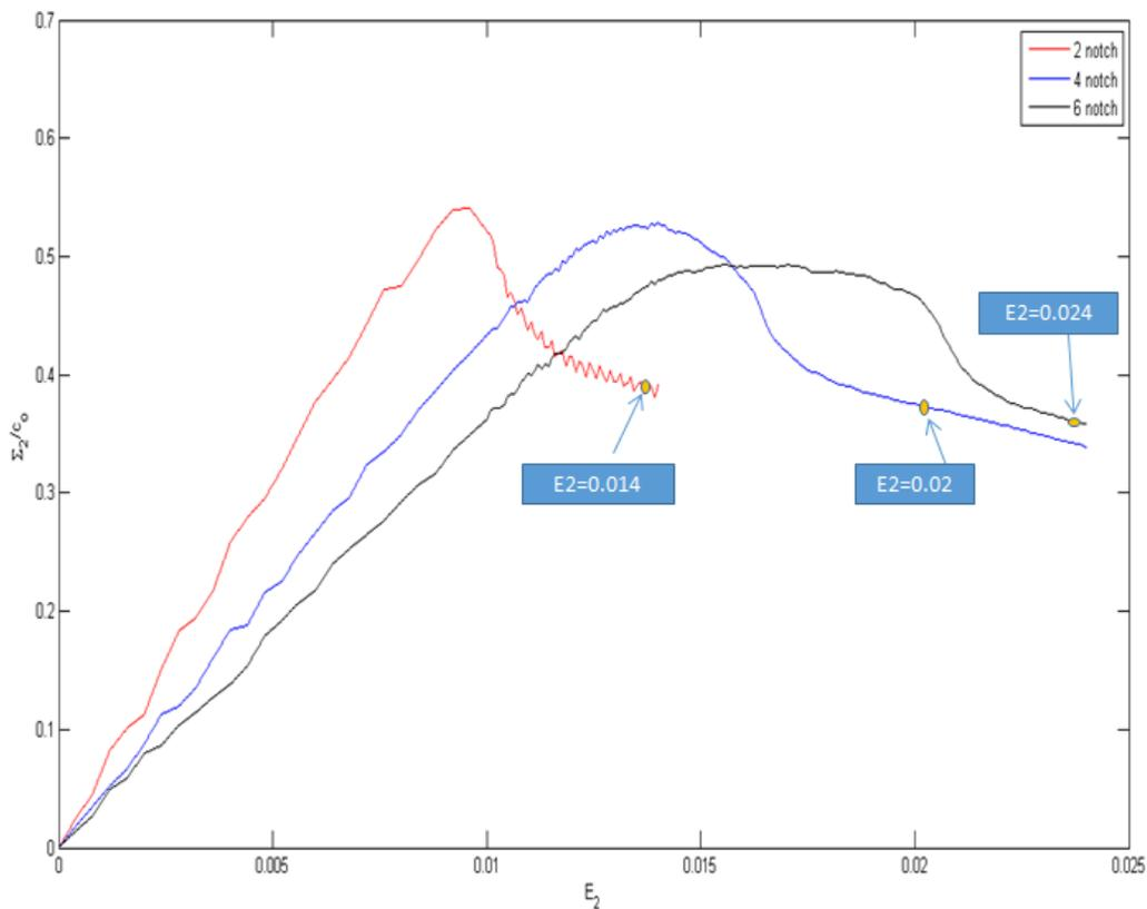
**Figure 7-** Normalized nominal stress vs strain curve for  $L_c=15\text{nm}$  for aperiodic notches
