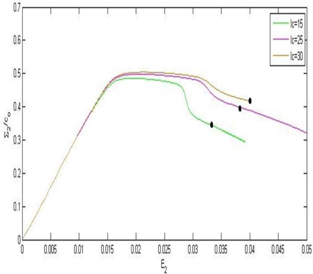
**Figure 16:-** Normalized nominal stress-strain curve for sample spacing  $S = 50\text{nm}$  and  $B = 20\text{nm}$  varying intrinsic length value.
