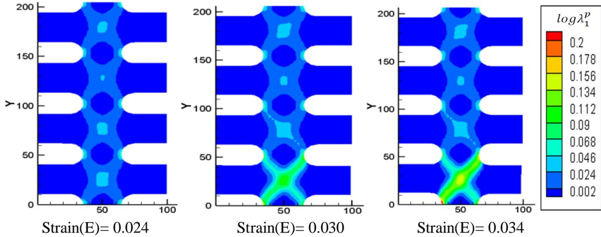
**Figure 19-** Contour plots of plastic evolution strain inside shear band for S=50 nm, Lc=15 nm. Varying Ligament length.
