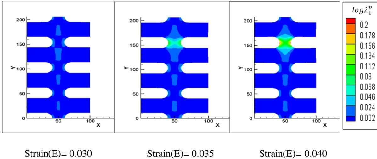
**Figure 17-** Contour plots of plastic evolution strain inside shear band for  $S=50$  nm,  $B=20$  nm. Varying intrinsic length.
