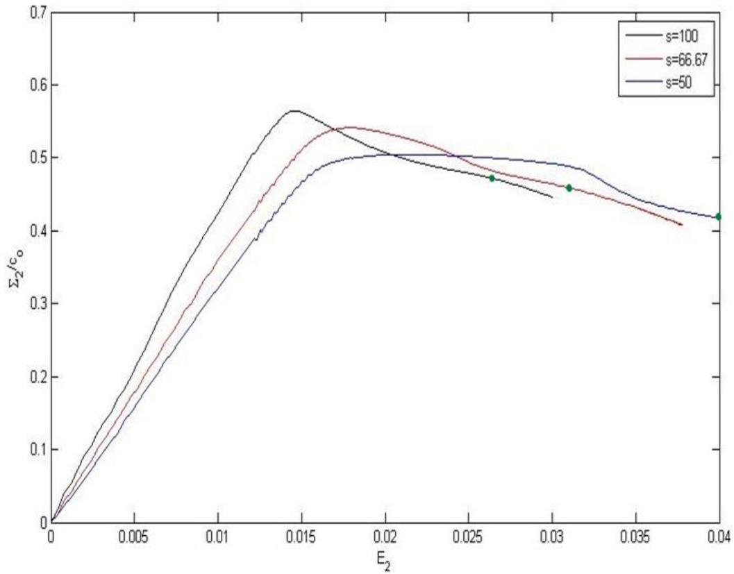
**Figure 14:-** Normalized nominal stress-strain curve for sample with  $L_c=30\text{nm}$  and  $B=20\text{nm}$  varying spacing between notches
