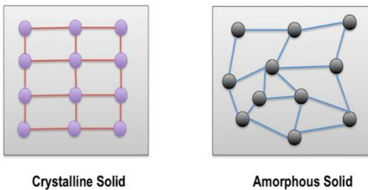
**Figure 1-:** Arrangement of Atoms
