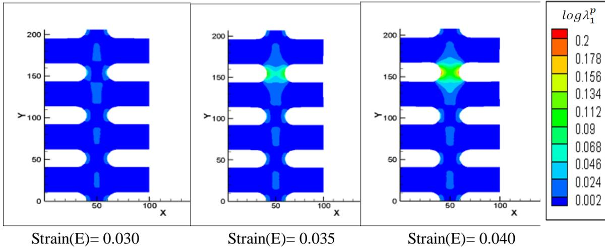
**Figure 15-** Contour plots of plastic evolution strain inside shear band for Lc=30 nm, B=20 nm. Varying spacing between periodic notches.
