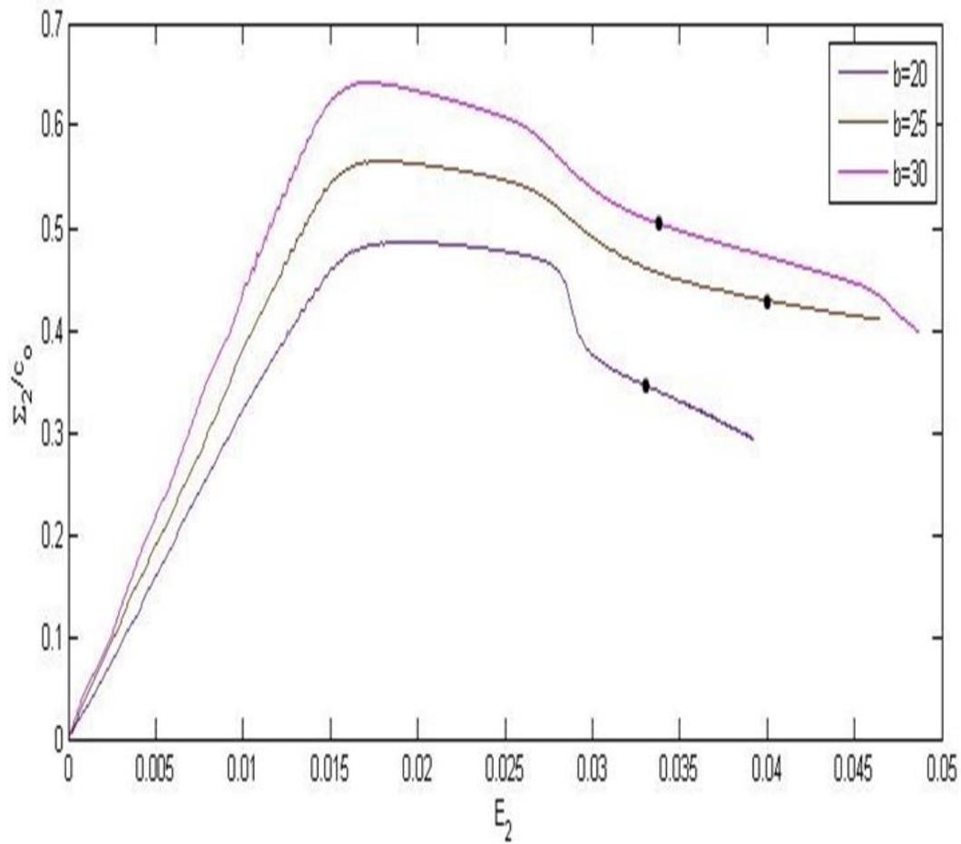
**Figure 18:-** Normalized nominal stress-strain curve for sample spacing  $S = 50\text{nm}$  and  $L_c = 15\text{nm}$  varying ligament length value.
