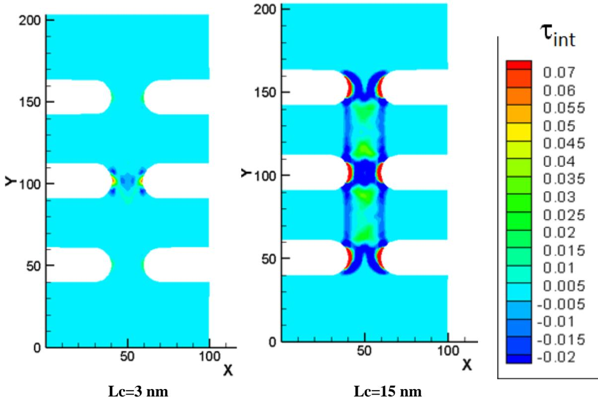
**Figure 11-** Contour plots for interaction stress ( $\tau_{int}$ ) value inside shear band
