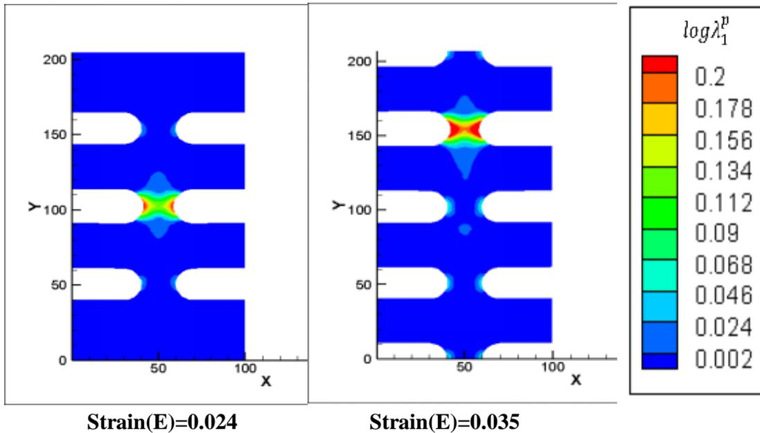
**Figure 13:-** Contour plots for Aperiodic and periodic notches.
