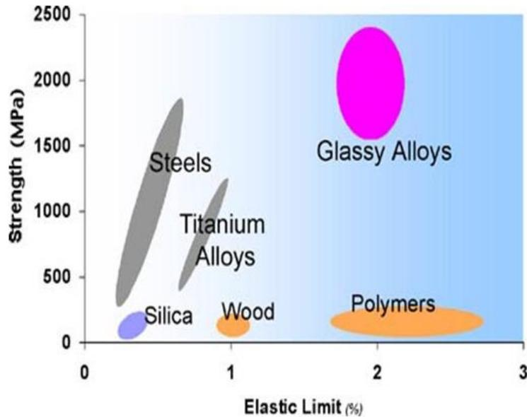
**Figure 3-:** Strength and Elastic strain plot for different materials.
