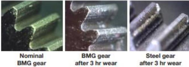
**Figure 4.4-:** (More than 3 million cycles were achieved at less than  $-100\text{ }^{\circ}\text{C}$  with dry lubricated hybrid gearbox).
