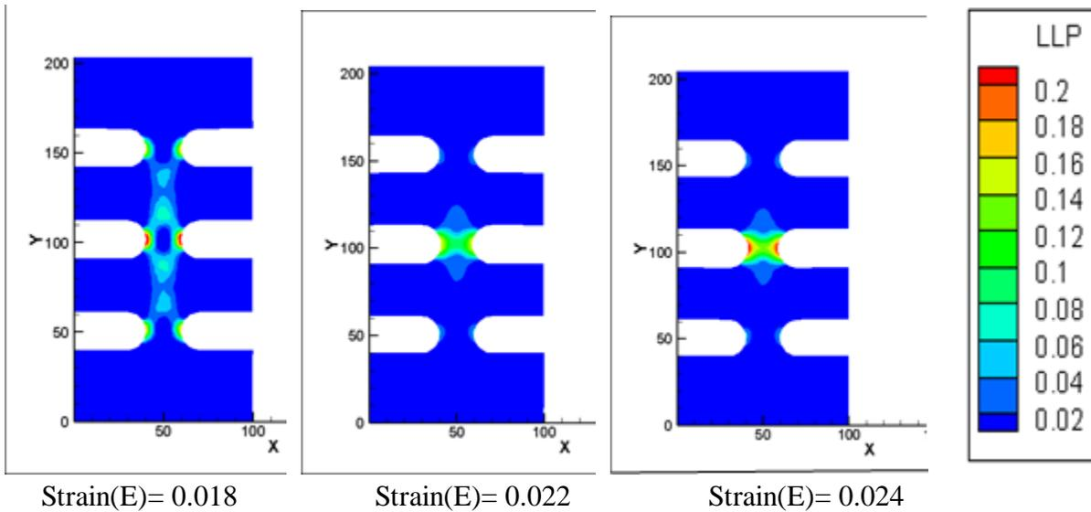
**Figure 8-** Contour plots of plastic evolution strain inside shear band for 2 and 6 notches for fixed  $L_c=15$  nm of Aperiodically placed notches.
