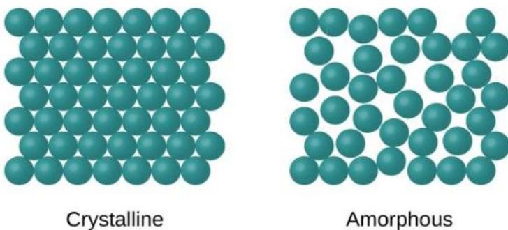
**Figure 2-:** Shape of Crystalline and Amorphous Solids
