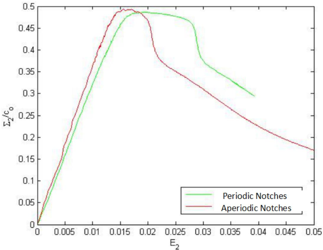
**Figure 12-** Normalized nominal stress-strain curve for Sample having periodic and aperiodic notches
