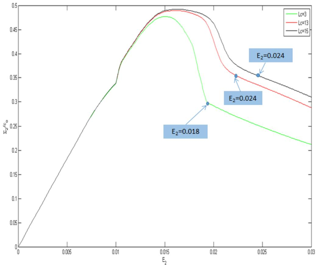
**Figure 9-** Normalized nominal stress vs strain curve aperiodically placed 6-notch sample
