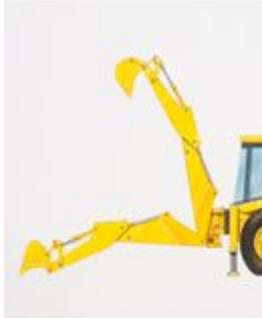
Fig 1.1 Extreme positions with minimum flexibility upon ground
