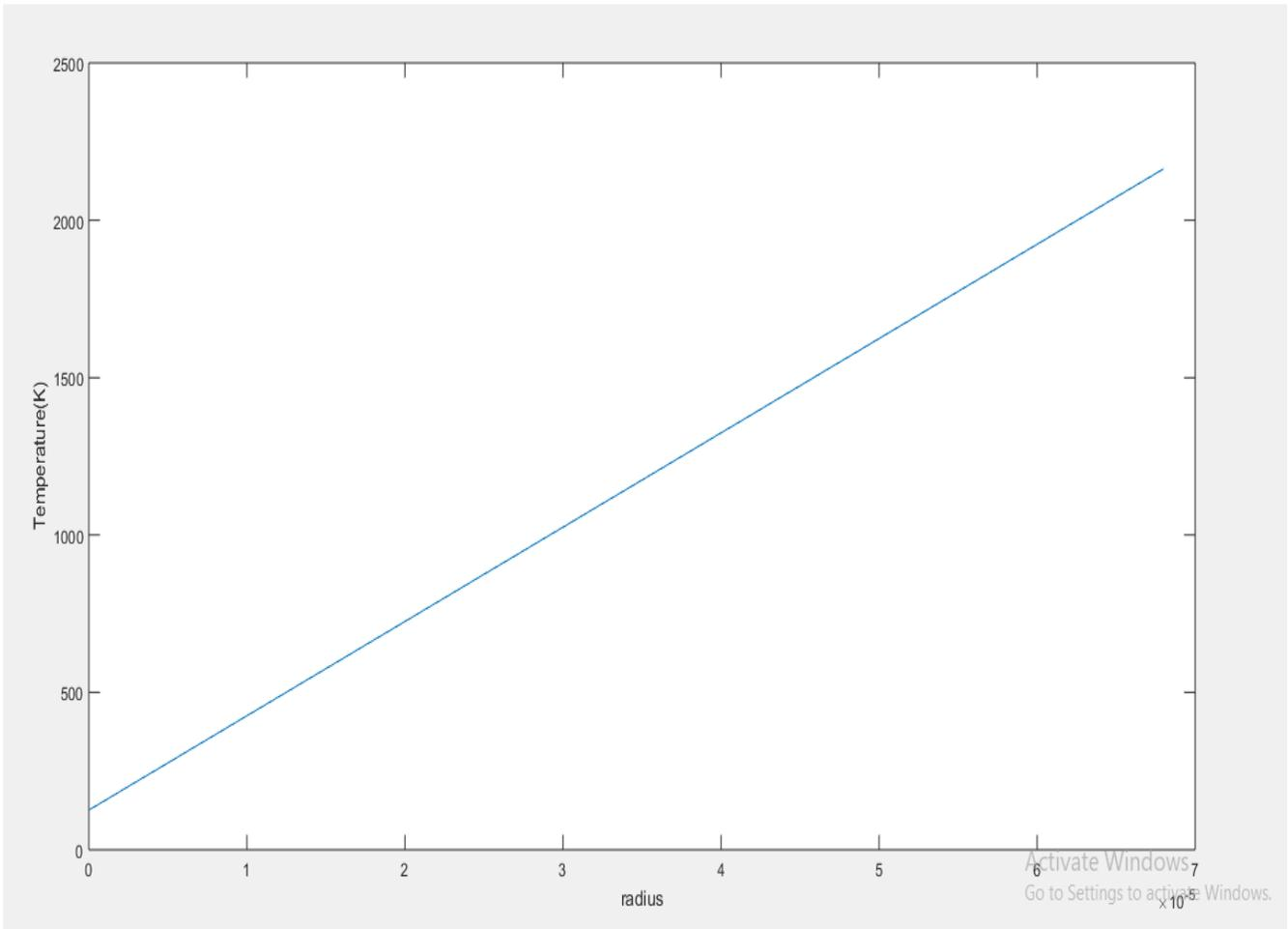
**Graph 1** shows the temperature distribution across the radius of the coal particle when thermal conductivity of the particle is constant.
