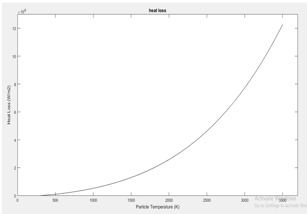
**Graph 5** shows rate of heat loss per external surface area by the particle as a function of particle temperature.
