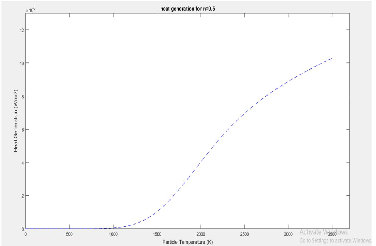
**Graph 3** shows rate of heat Generation inside the coal particle per external surface area as a function of particle temperature, for  $n=0.5$
