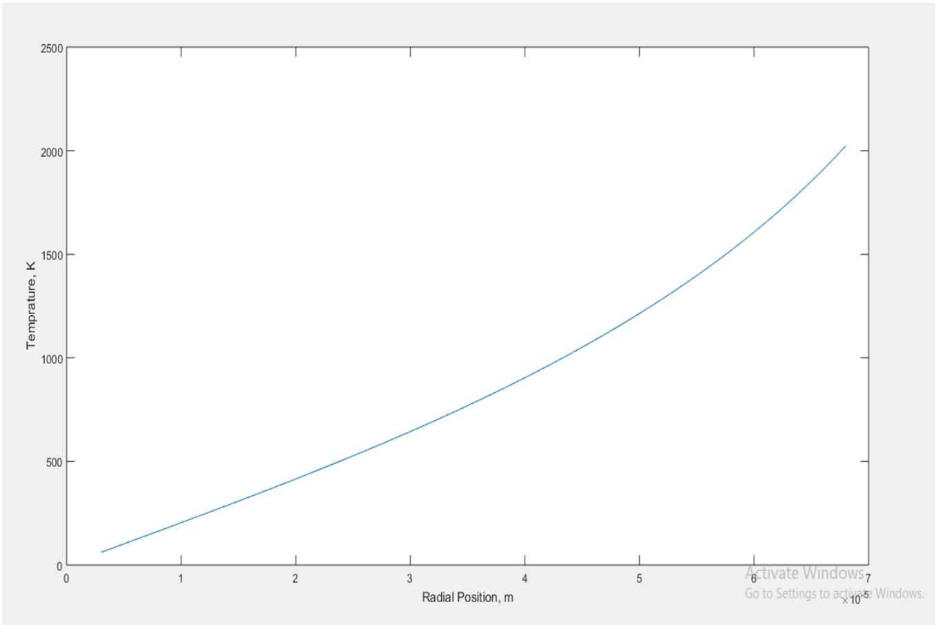
**Graph 2** shows the temperature distribution within a 136 μm carbon particle uniformly heated on its surface by a laser pulse for 150 μs.
