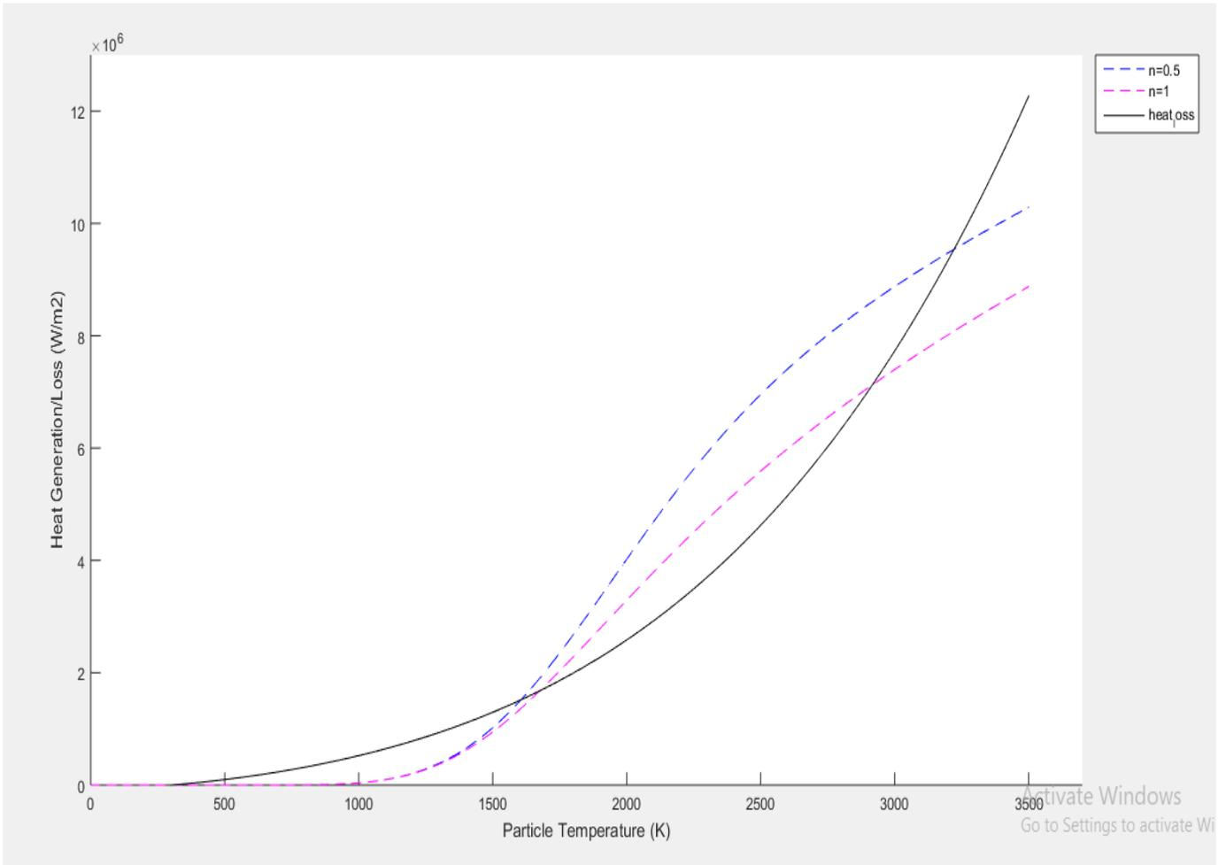
**Graph 6** shows the rates of heat loss (solid curve) and heat generation (dashed curves) per external surface area as a function of particle temperature.
