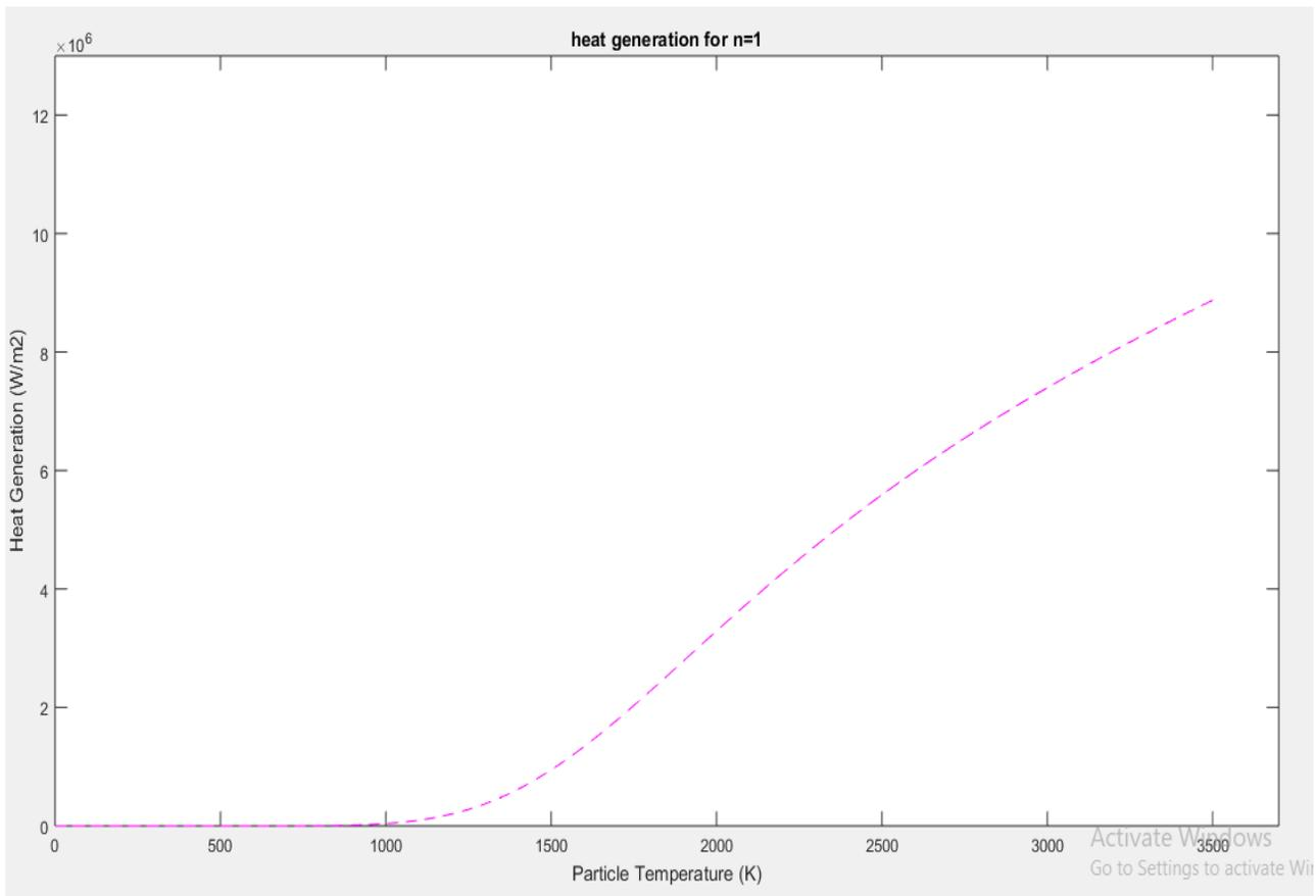
**Graph 4** shows rate of heat Generation inside the coal particle per external surface area as a function of particle temperature, for n=1.
