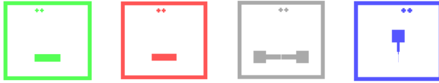
Fig. 7.1: The L-Edit image of the mask in which green color mask is for active area formation, the red one is for insulator pad formation, the gray one is for source and drain contact fabrication, and blue one is for gate contact fabrication.
