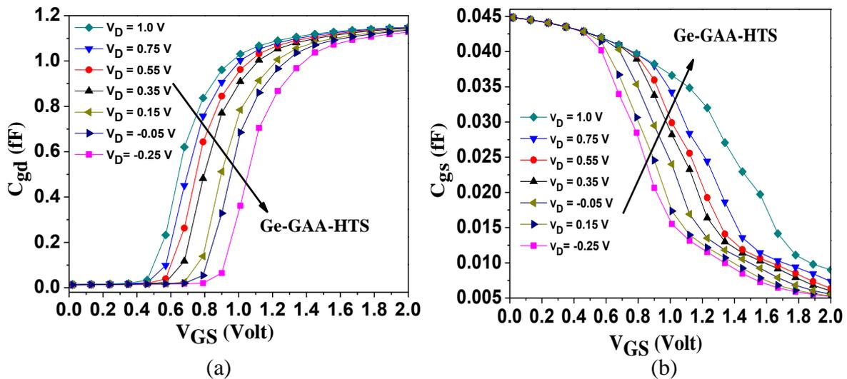
Figure 3.7 (a) Analysis of gate-to-drain capacitance ( $C_{gd}$ ), and (b) Gate to source capacitance ( $C_{gs}$ ) as function of the gate to source voltage ( $V_{gs}$ ) for different value of  $V_{ds}$  for Ge-GAA-HTS.
