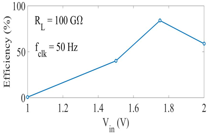
Figure 5.16 Efficiency of the proposed design with varying input voltage under the fixed value of  $R_L = 100\text{ G}\Omega$ .
