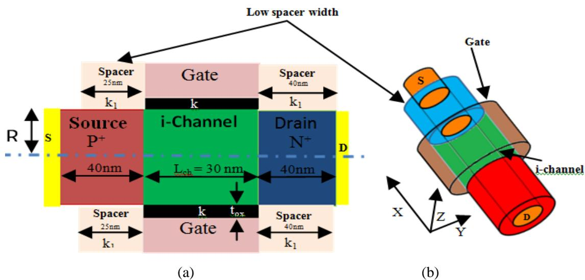
Figure 1.8 (a) Cross-Sectional view, and (b) 3D view of Cylindrical Gate-All-Around n-channel Tunnel FET based on low spacer width (LSW) along channel length direction. Here S-Source, D-Drain, C-Channel, R-radius and  $k$  and  $k_1$  are the gate/spacer dielectric.
