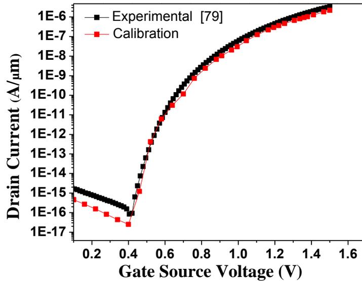
Figure 2.5 shows the calibration of our simulation result of the examined device with experimental data of [79].
