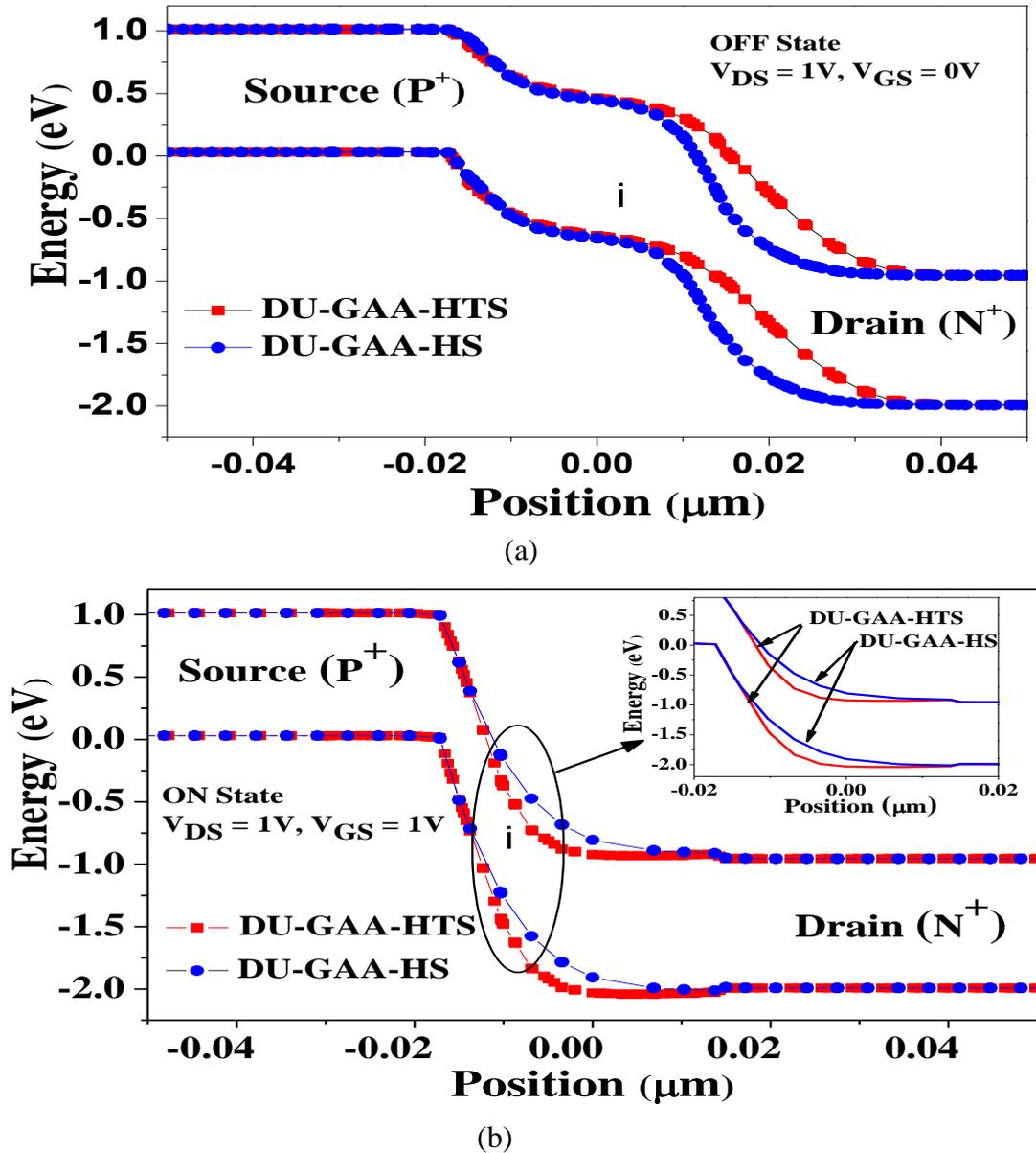
Figure 4.3 Comparison of energy band diagram for DU Cyl-GAA with hetero and homo spacer dielectric in the case of (a) OFF state, and (b) ON state. The inset shows the position of band bending between the valence band of the source and conduction band of the channel during tunneling of charge carriers.
