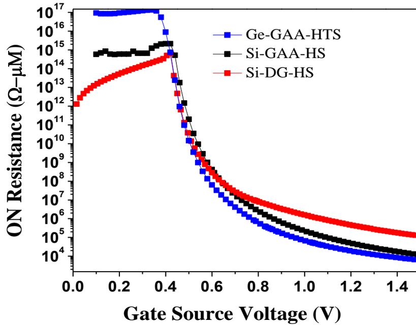
Fig. 3.6 Transfer characteristics of ON Resistance with respect to gate source voltage
