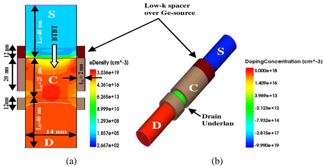
Figure 3.1 (a) A Cross-sectional view and (b) 3-D view of Drain Underlap (DU) Cyl-GAA-TFET based on Ge-Source overlapped with hetero-spacer (HTS) dielectric along channel length direction with magnitude of electron (*e*) current density and doping concentrations. Here S-Source, D-Drain, and C-Channel. Also,  $L_{cb}$ ,  $L_{ss}$ , and  $L_{ch}$  represent the drain, source, and channel length.
