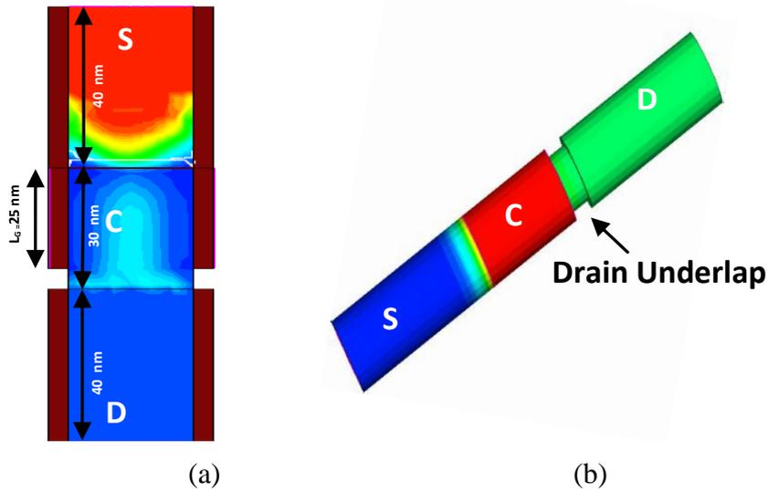
Figure 2.13 (a) Cross-sectional view (b) 3-D view of electrostatic potential of drain underlap (DU) Cyl-GAA-TFET with Ge Source. Here, S-Source, D-Drain, and C-Channel, gate length ( $L_g$ ) = 25 nm, oxide thickness ( $t_{ox}$ ) = 2 nm.
