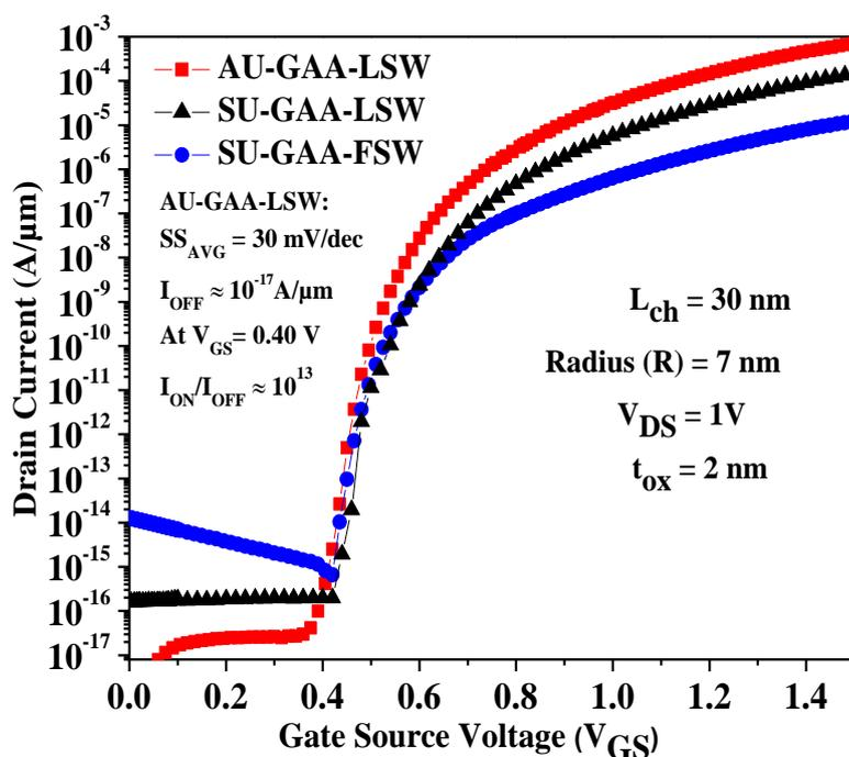
Figure 2.6 Transfer characteristic of AU, SU-Cyl-GAA with LSW/FSW of TFET.
