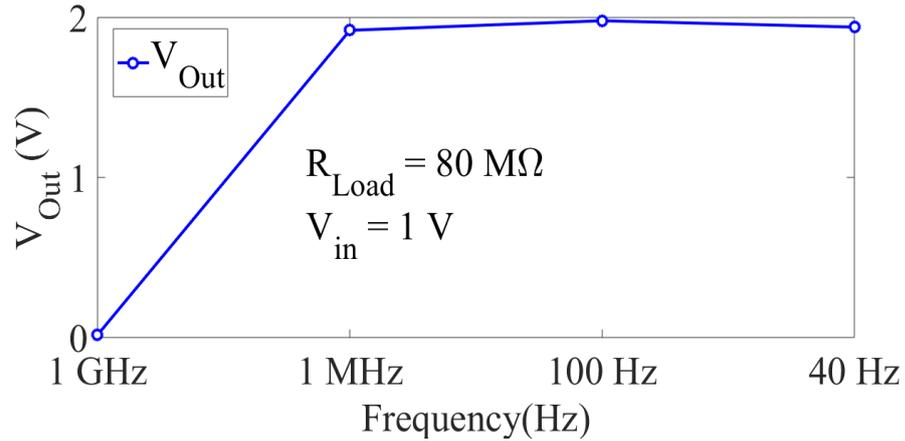
Figure 5.15 The output voltage of the proposed design under different frequency range (i.e. 40 Hz to 1 GHz) while keeping fixed value of  $R_L$ .
