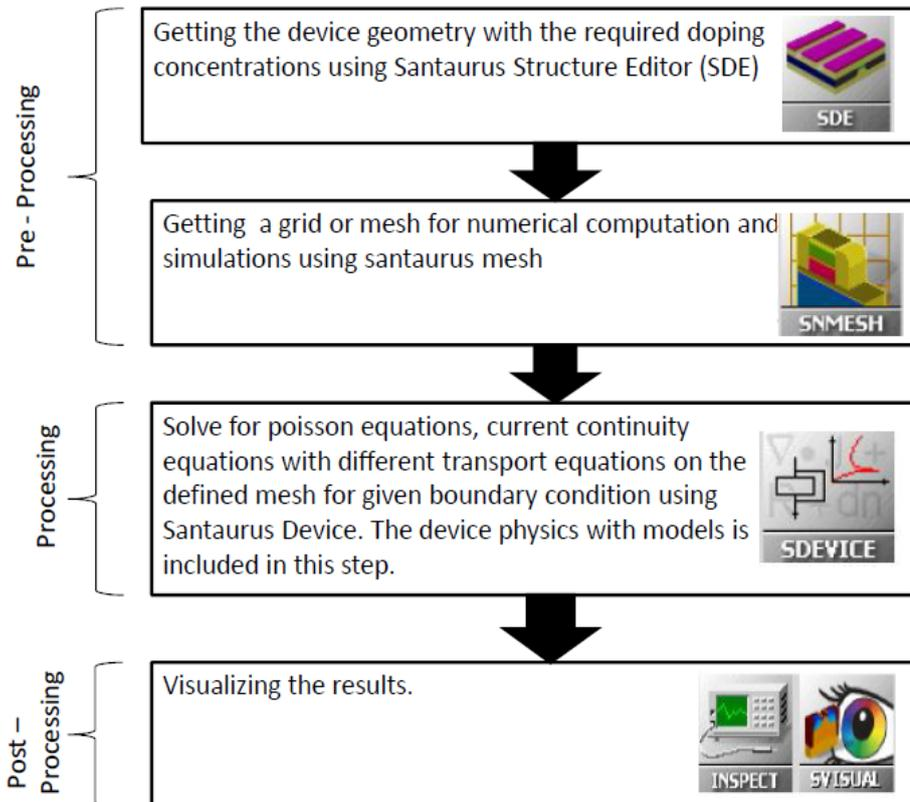
Figure 1.5: Device simulation steps with Synopsys Sentaurus Device TCAD [49].
