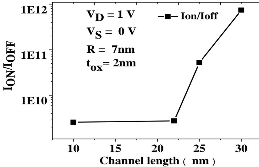
Figure 2.12 ON-OFF ratio of AS-GAA-TFET.
