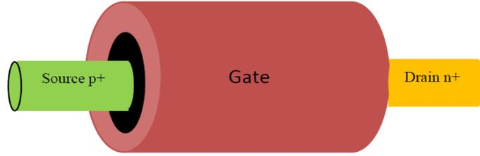
Figure 1.7 3D view of Cylindrical (Cyl) Gate-all-around (GAA) n-channel TFET
