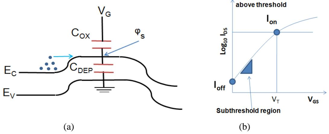
Figure 1.1 n-channel MOSFET (a) Energy band diagram model with associated capacitances (b) Transfer characteristics corresponding to ON-state current [33], [36].
