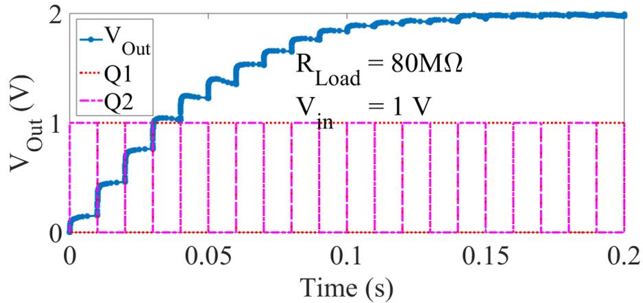
Figure 5.11 Transient response of the *CCVD* for the fixed value of load resistance  $R_L$  with non-overlapping control scheme
