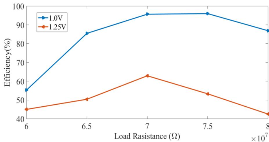
Figure 5.12 shows the efficiency of the proposed design for varying  $R_L$  under different values of drain voltage.
