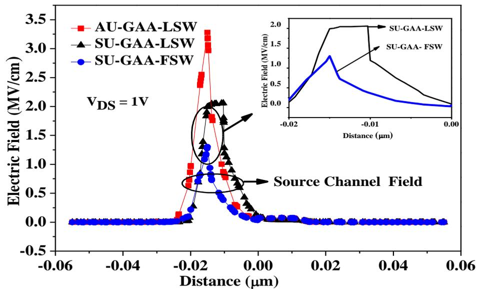
Figure 2.7 Comparison of simulated lateral electric field strengths for the three examined devices.
