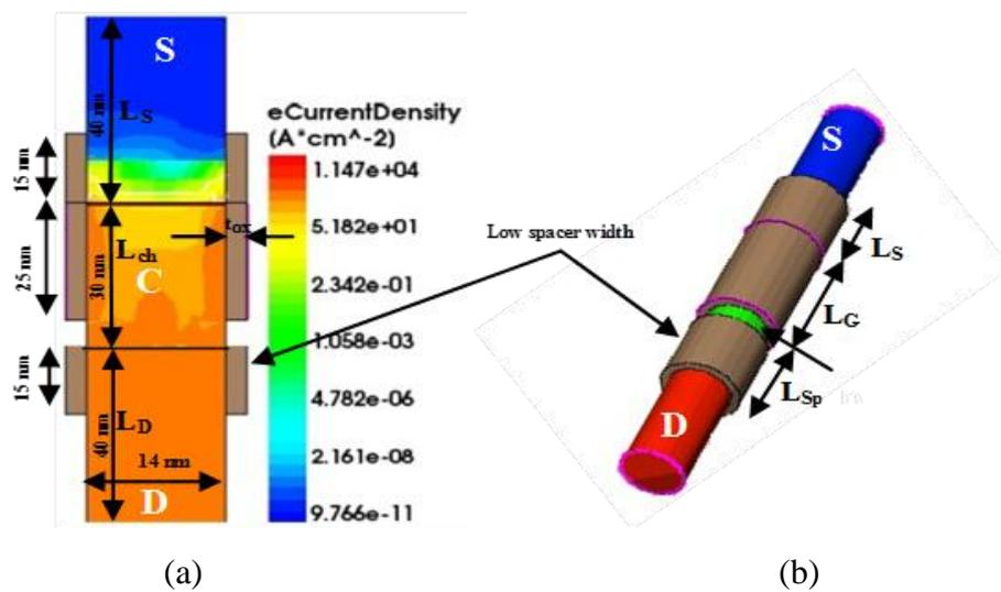
Figure 2.4 (a) Cross-sectional view, and (b) 3-D view of asymmetrical underlap (AU)-Cyl GAA-TFET with LSW. Here, gate length ( $L_g$ ) = 25 nm, spacer width ( $L_s$ ) = 15 nm, oxide thickness ( $t_{ox}$ ) = 2 nm is used.
