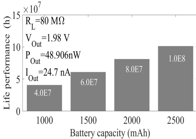
Figure 5.18 Life time performances of the proposed *CCVD* design under different battery capacity (*mAh*).
