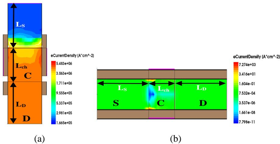
Figure 3.2 (a) Cross-sectional views of (a) DU Cyl-GAA-Tunnel FET, and (b) Double Gate-Tunnel FET based on *Si*-Source overlapped with HS along channel length direction with magnitude of electron current density.
