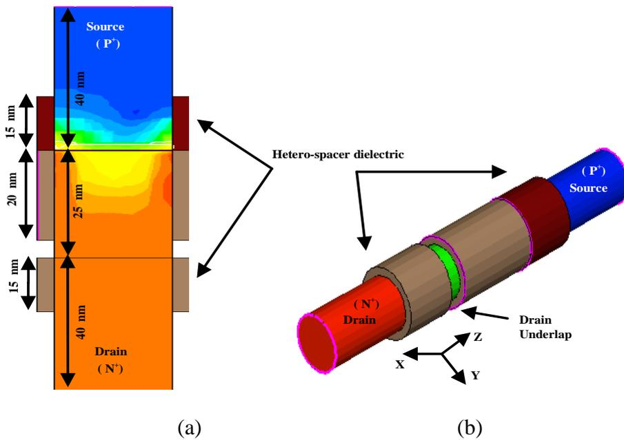
Figure 4.1 (a) Cross-Sectional view, and (b) 3D view of drain underlap (DU)-Cyl-GAA-TFET with HTS. Here, gate length ( $L_g$ ) = 20 nm, spacer width ( $L_s$ ) = 15 nm, oxide thickness ( $t_{ox}$ ) = 2 nm, and thickness of high-k dielectric ( $HfO_2$ ) = 2 nm are used.
