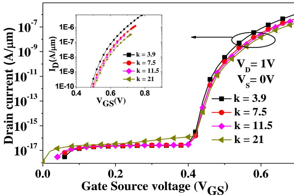
Figure 4.4 Transfer Characteristic of DU GAA-TFET for different values of the source spacer dielectric on  $V_{gs}$  scale of 0.8 V. The inset shows the output characteristics in defined gate source voltage of drain current for increase in value of source spacer dielectric ( $k$ ).
