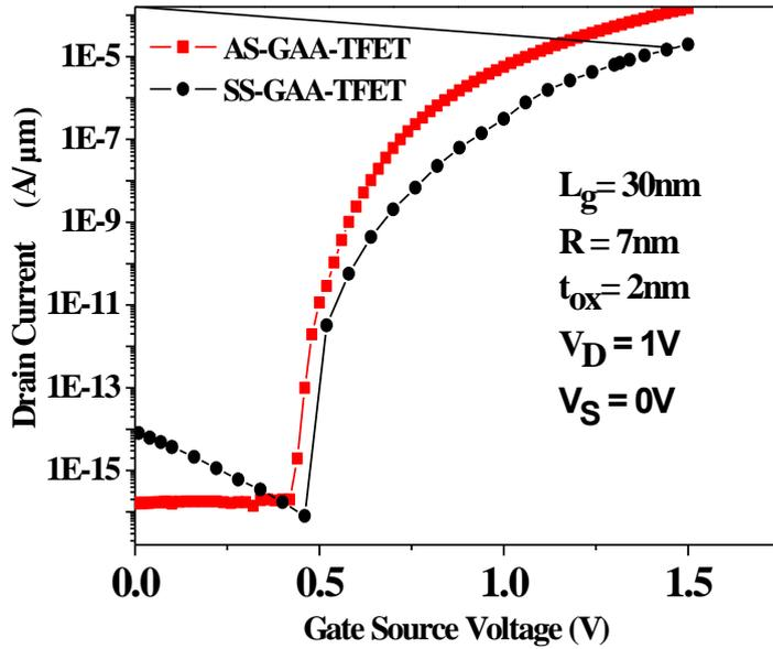
Figure 2.10 Transfer Characteristic of AS and SS-GAA-TFET at  $V_G=1.5V$ .
