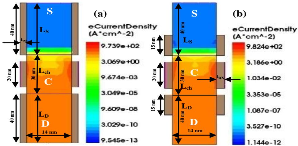
Figure 2.3 Cross-sectional views of symmetrical underlap (SU) Cyl-GAA-TFETs with (a) full spacer width (FSW), and (b) low spacer width (LSW) along channel length direction with magnitude of electron ( $e$ ) current density.
