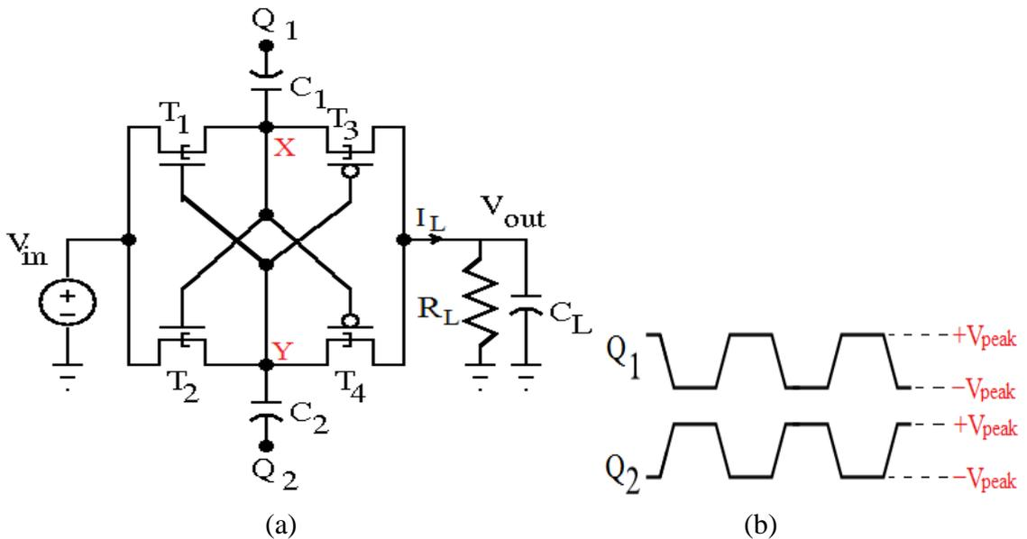
Figure 5.6 (a) Schematic diagram of the Cross Coupled Voltage Doubler (CCVD), (b) Non-overlapping control scheme
