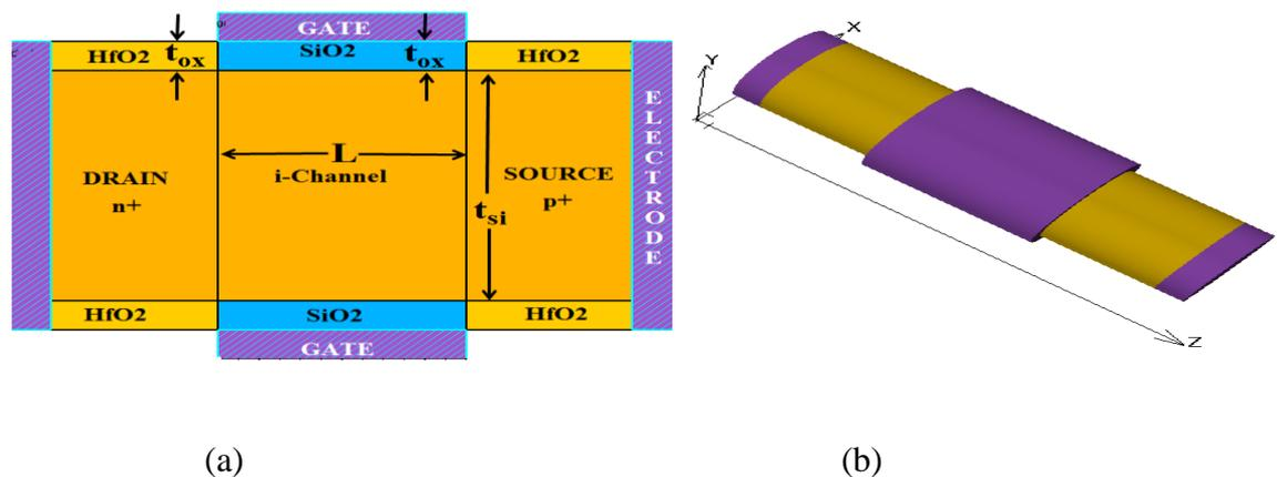
Figure 3.9 (a) 3D view, and (b) Cross-sectional view of simulated Cylindrical GAA- n channel-Tunnel FET along z axis
