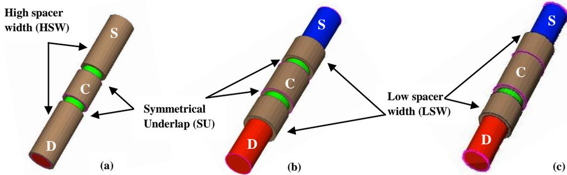
Figure 2.1 3D views of Cyl GAA Tunnel-FET, (a) Symmetrical underlap (*SU*) with full spacer width (*FSW*), (b) *SU* with low spacer width (*LSW*), and (c) Asymmetrical underlap with *LSW*. Here S-Source, D-Drain, and C-Channel.
