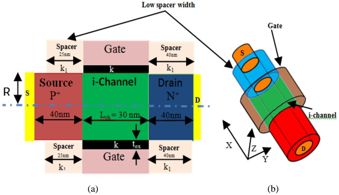
Figure 2.9 (a) Cross-Sectional view, and (b) 3D View of Cyl GAA-n-channel Tunnel FET based on asymmetrical spacer width (ASW) along channel length direction.
