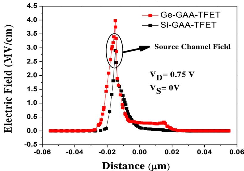
Figure 2.15 Comparison of electric field strengths in the case of Si and Ge- Cyl GAA-TFET.
