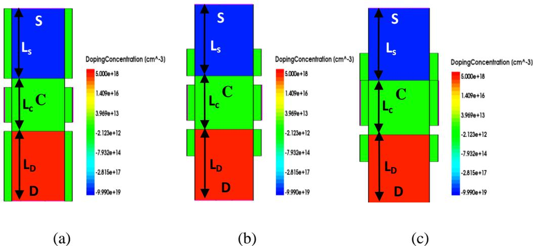
Figure 2.2 Cross-sectional views of Cyl-GAA-TFETs along channel length direction with magnitude of doping concentration. (a) *SU-FSW*, (b) *SU-LSW*, (c) *AU-LSW*. Here  $L_d$ ,  $L_s$ , and  $L_{ch}$  represents the drain, source and channel length.
