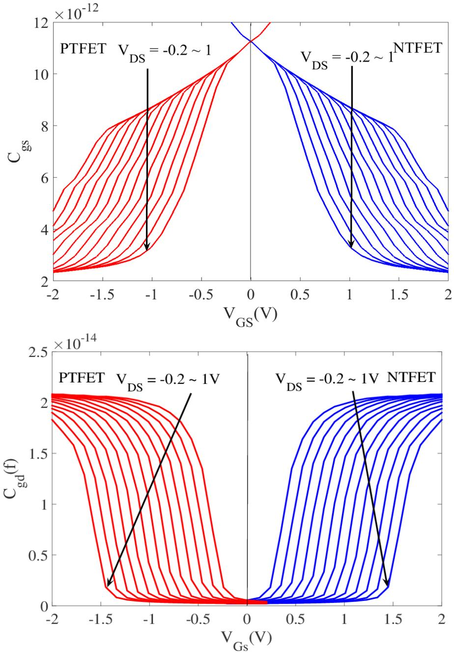
Figure 5.4 Device capacitance extraction (a) Characteristics of gate-to-drain capacitance and (b) gate-to-source capacitance as a function of gate to source voltage ( $V_{gs}$ ) for different value of  $V_{ds}$  on p and n channel Cylindrical (Cyl) GAA-Tunnel FET.
