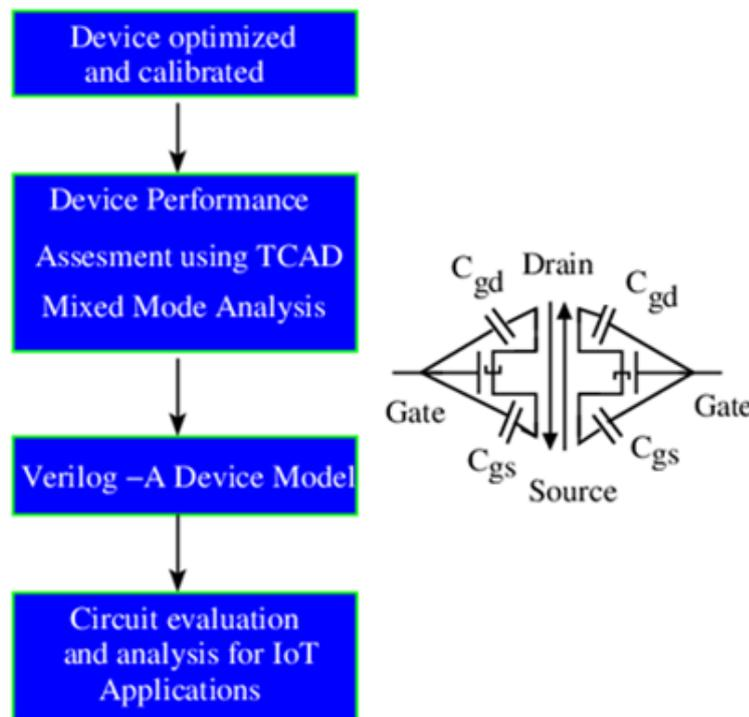
Figure 5.3 Flowchart for the simulation methodology used in the design and modeling of the CCVD design based on Cyl GAA-Tunnel FET.
