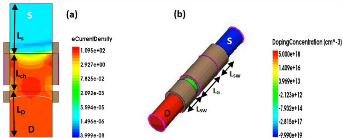
Figure 5.1 (a) Cross-sectional view and (b) 3D view of asymmetrical underlap (AU) Cyl-GAA-TFET based on Ge-source with low spacer width ( $L_{SW}$ ) along channel length direction with magnitude of e-current density and doping concentrations.
