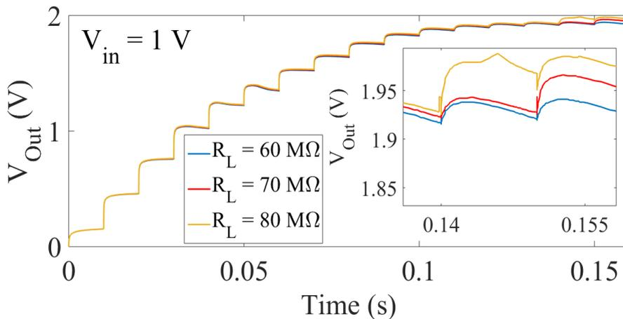
Figure 5.14 Output voltage characteristics of the proposed design for different values of  $R_L=60, 70, 80 M\Omega$ , the inset shows the detail variation of output voltage for different  $R_L$  in the given time slot
