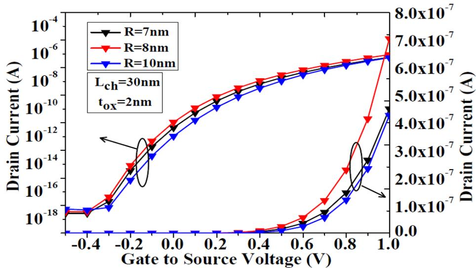
Figure 3.11  $I_{ds}$ - $V_{gs}$  characteristics of GAA-TFET for different radius on linear scale and logarithmic scale
