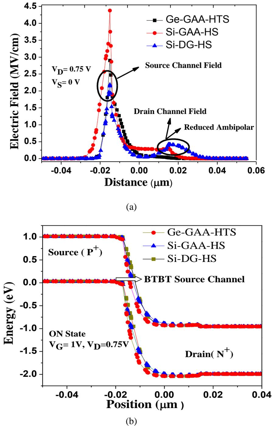
Figure 3.5 (a) Simulated lateral electric field strengths of all the three proposed structures of TFET, and (b) Comparison of energy band diagram for the three structures of Tunnel FET based on *Si/Ge*-source overlapped with HTS and HS dielectric in the case of ON state of the devices.
