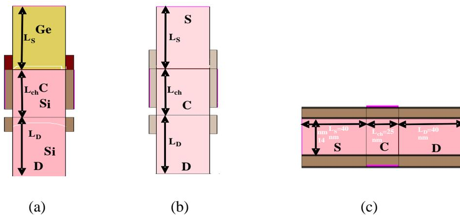
Figure 3.3 (a) Cross-sectional views of material regions of (a) DU Cyl-GAA-TFET based on Ge-Source overlapped with HTS, (b) DU Cyl-GAA-TFET, and (c) Double Gate-TFET based Si-Source overlapped with HS. Here, the gate length ( $L_G$ ) = 20 nm, spacer width ( $L_s$ ) = 12 nm, oxide thickness ( $t_{ox}$ ) for both the spacers and gate are 2 nm
