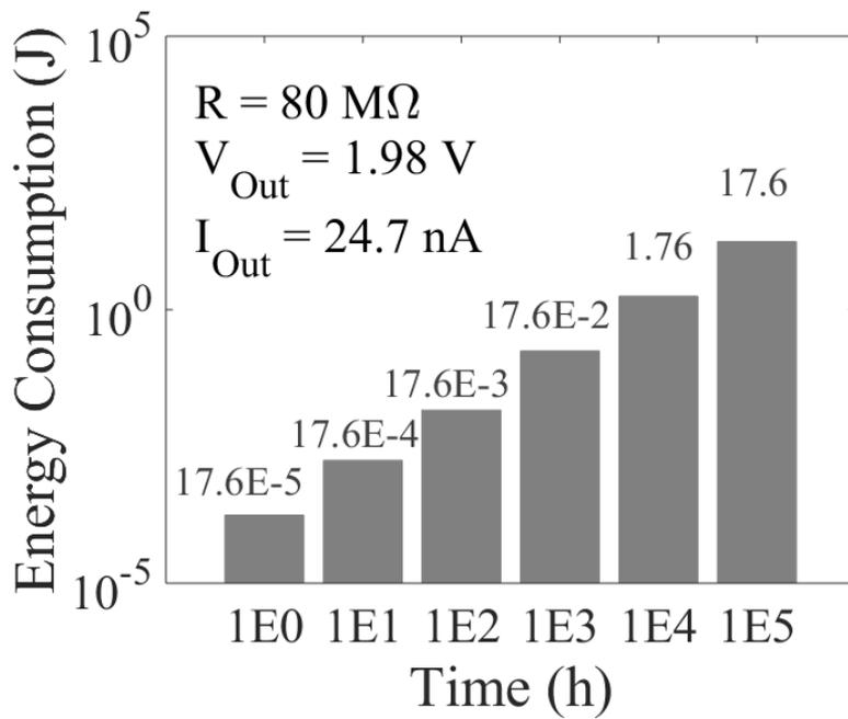
Figure 5.17 Energy consumption of the proposed design for the different time cycles
