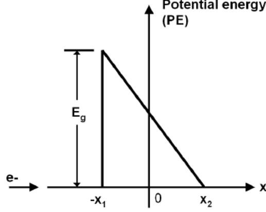
Figure 1.4 Triangular potential energy barrier approximation for band to band tunneling in TFET [45].
