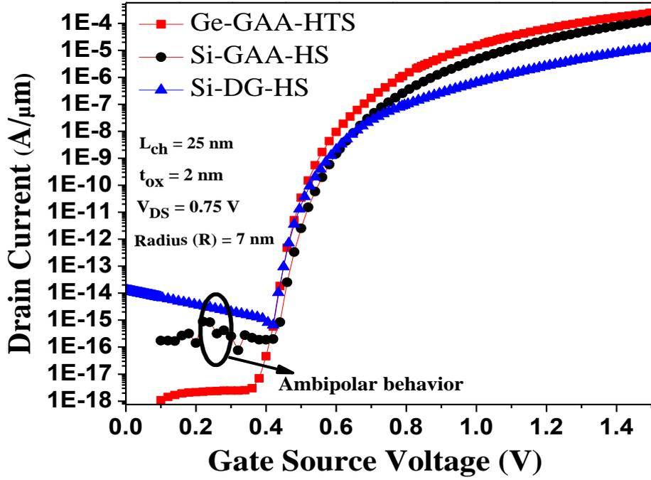
Figure 3.4 Transfer characteristics of DU GAA-TFET and DG-TFET based on Si/Ge Source overlapped with hetero and homo spacer dielectric at  $V_g=1.5$  V. The effective channel length is 25 nm. The inset shows the calibration of our simulation result with [60].
