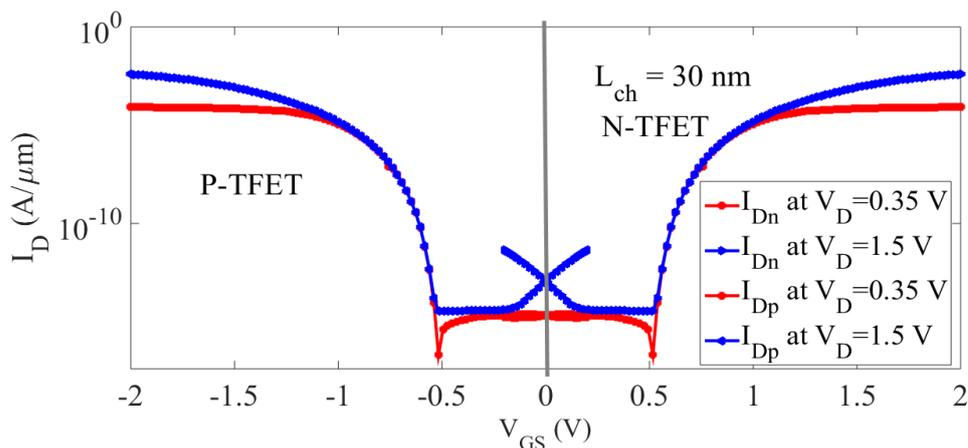
Figure 5.2 Transfer characteristics of Cyl GAA-Tunnel FET.
