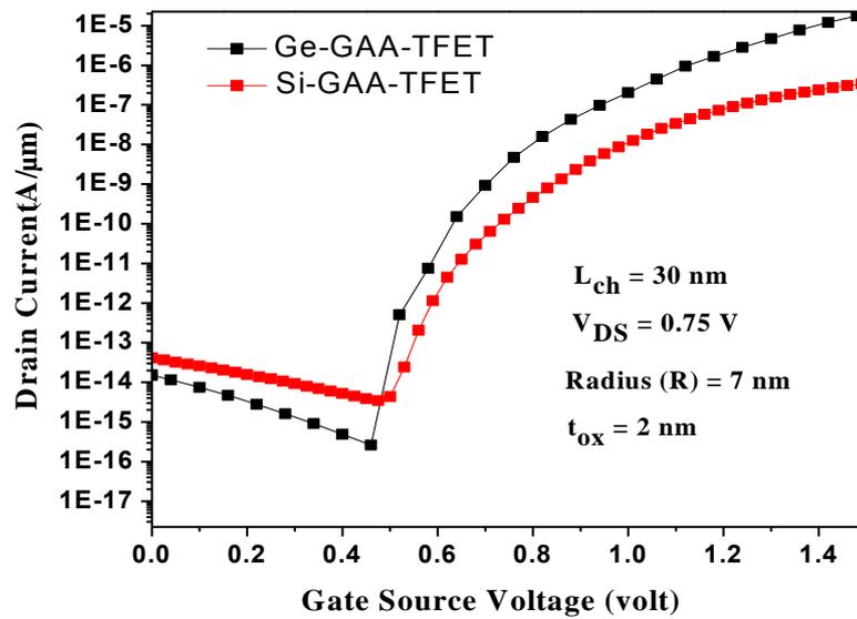
Figure 2.14 Transfer Characteristic of  $I_d$ - $V_g$  of the examined device
