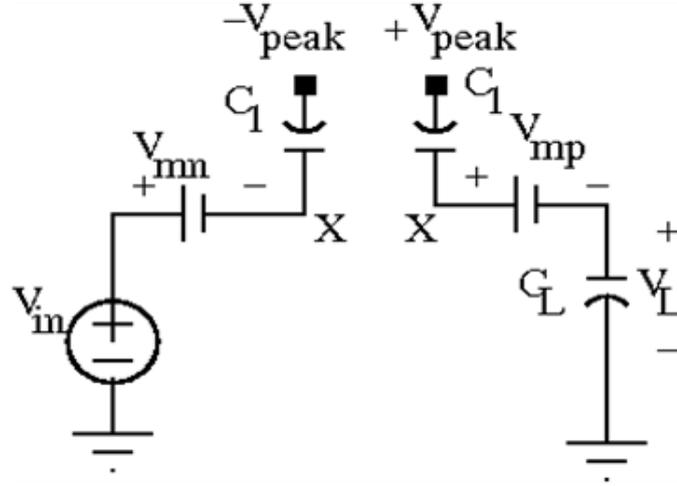
Figure 5.8 modeling of the proposed CCVD Design for charging phase and discharging phase
