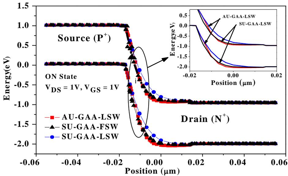
Figure 2.8 Energy band diagram in the case of AU, SU-Cyl GAA with LSW and FSW of Tunnel FET.
