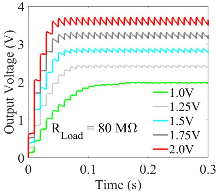
Figure 5.10 Transfer characteristics of the output voltage of the CCVD design for five different values of input voltage ( $V_{in}$ ).
