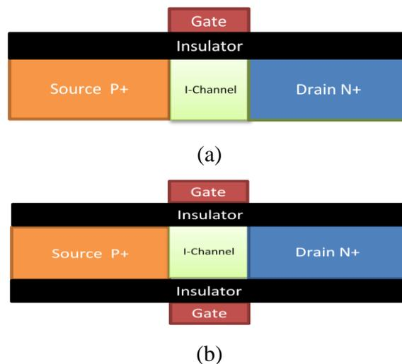
Figure 1.2 n-channel Tunnel FET device structure with (a) Single gate (SG), and (b) Double gate (DG)
