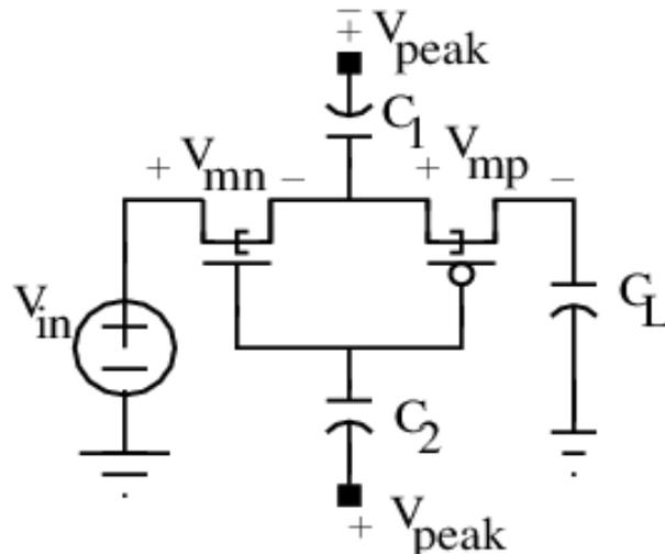
Figure 5.7 Bisector view of the CCVD circuit.
