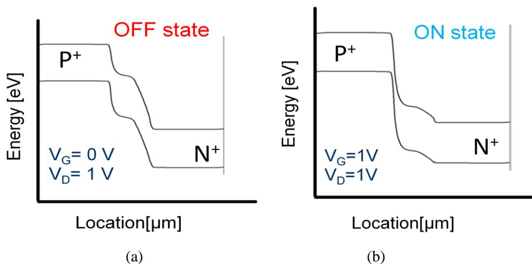
Figure 1.3 Energy band diagram of n-channel Tunnel FET (a) during OFF state (b) during ON state.
