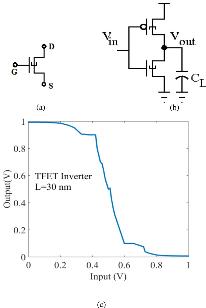
Figure 5.5 Circuit characteristics (a) symbolic representation of n-channel Cyl GAA-Tunnel FET, (b) Cyl GAA-Tunnel FET based Inverter circuit with load capacitance, and (c) Voltage transfer characteristics of proposed device based Inverter.
