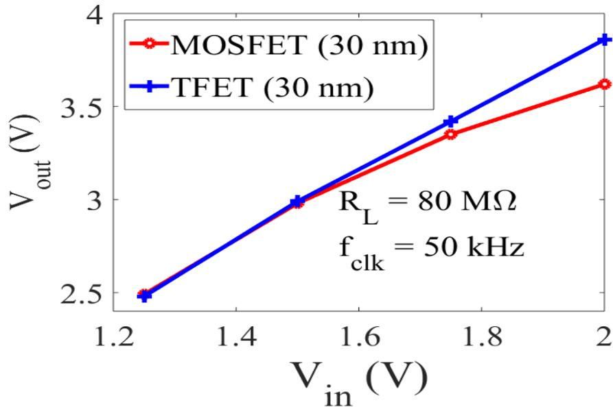
Figure 5.13 shows the comparison of transfer characteristics of output voltages for the proposed design based on TFET and MOSFET.
