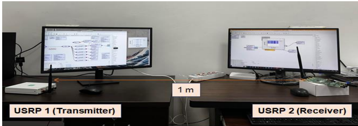
Fig. GNU Radio-based USRP B210 testbed setup
