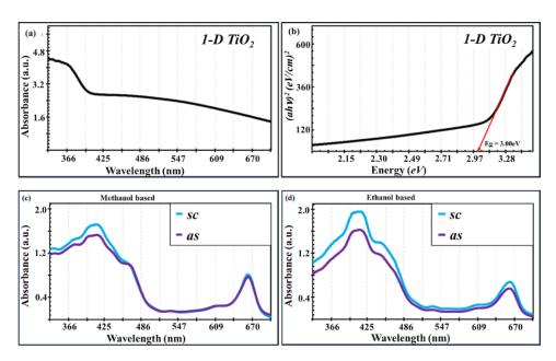
**Figure 4.7.** UV-visible absorption studies of (a) 1-D TiO<sub>2</sub> photoanodes and (b) Corresponding Tauc's plot for estimation of the bandgap,
