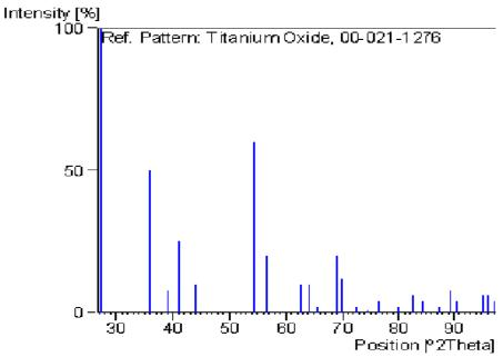
**Figure 4.5.** XRD pattern of (a) FTO substrate, and (b) 1-D TiO<sub>2</sub> nanorods, hydrothermally synthesized on the FTO substrate. (c) 21-1276 JCPDS data. FTO peaks are denoted by an asterisk (\*).
