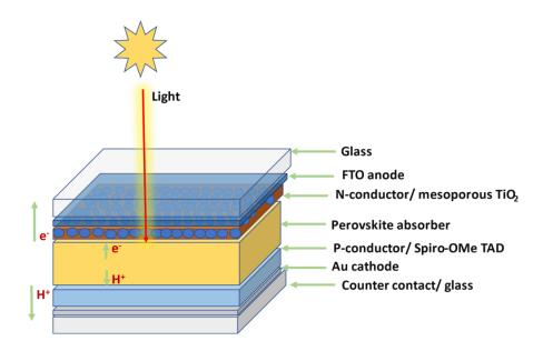
**Figure 1.3.** A simplified display of 3<sup>rd</sup> generation cells - Perovskite solar cell.
