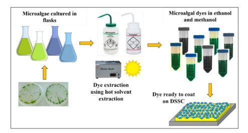
**Figure 4.1.** Typical schematic representation of microalgal-dye extraction process.
