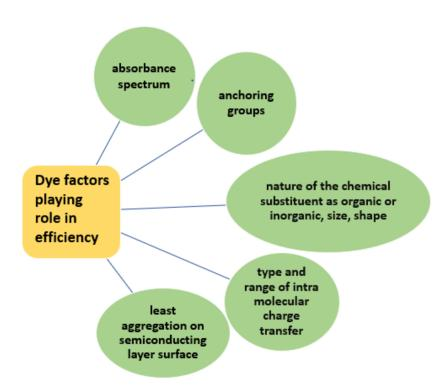
**Figure 1.6**. Representation of Dye factors playing a role in the efficiency
