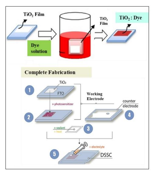
**Figure 4.2.** Step-wise schematic of the DSSC fabrication by utilizing microalgal dye and 0.05 M  $(I^-/I_3^-)$  electrolyte.
