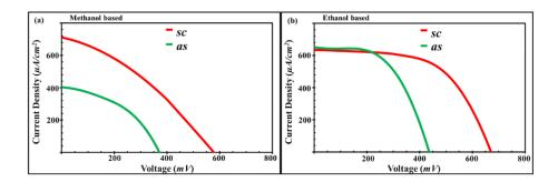
**Figure 4.9.** J-V analysis of the fabricated DSSC by utilizing microalgae (*as* and *sc*) natural photo harvesters, which are extracted in (a) ethanol, and (b) methanol.
