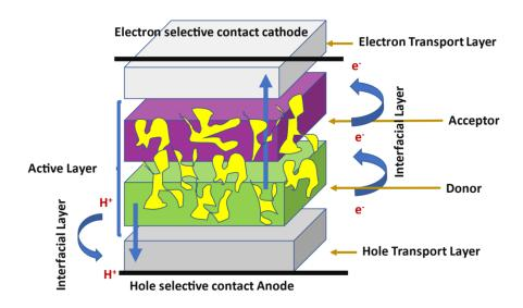
**Figure 1.2**. Schematic illustration of an organic solar cell in charge extraction mode.
