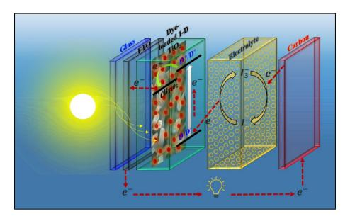
**Figure 4.3.** Typical schematics of DSSC include FTO, dye-loaded 1-D TiO<sub>2</sub> photo-anode matrix, electrolyte, and carbon counter electrode, depicting the working mechanism of the fabricated DSSC.
