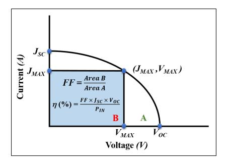
**Figure 4.4.** Schematic representation of different performance parameters for a general solar cell such as  $J_{SC}$ ,  $J_{MAX}$ ,  $V_{OC}$ ,  $V_{MAX}$ , FF, and PCE  $(\eta)$ .
