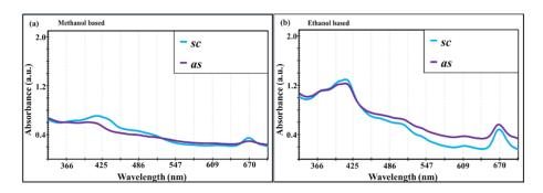
**Figure 4.8.** Absorption spectra of microalgae-based dyes extracted and coated on TiO<sub>2</sub> respectively.
