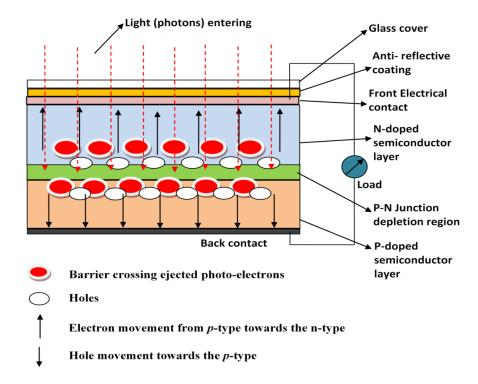
**Figure 1.1**. Structural overview of the operational mechanism in basic solar cells.
