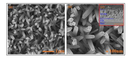
**Figure 4.6.** Morphology of hydrothermally grown TiO<sub>2</sub> nanorods, (a-b) FESEM-Top view of TiO<sub>2</sub> photoanodes at 15kX and 30kX magnifications, respectively, and (c) Cross-sectional-FESEM image showing the vertical aligned TiO<sub>2</sub> nanorods.
