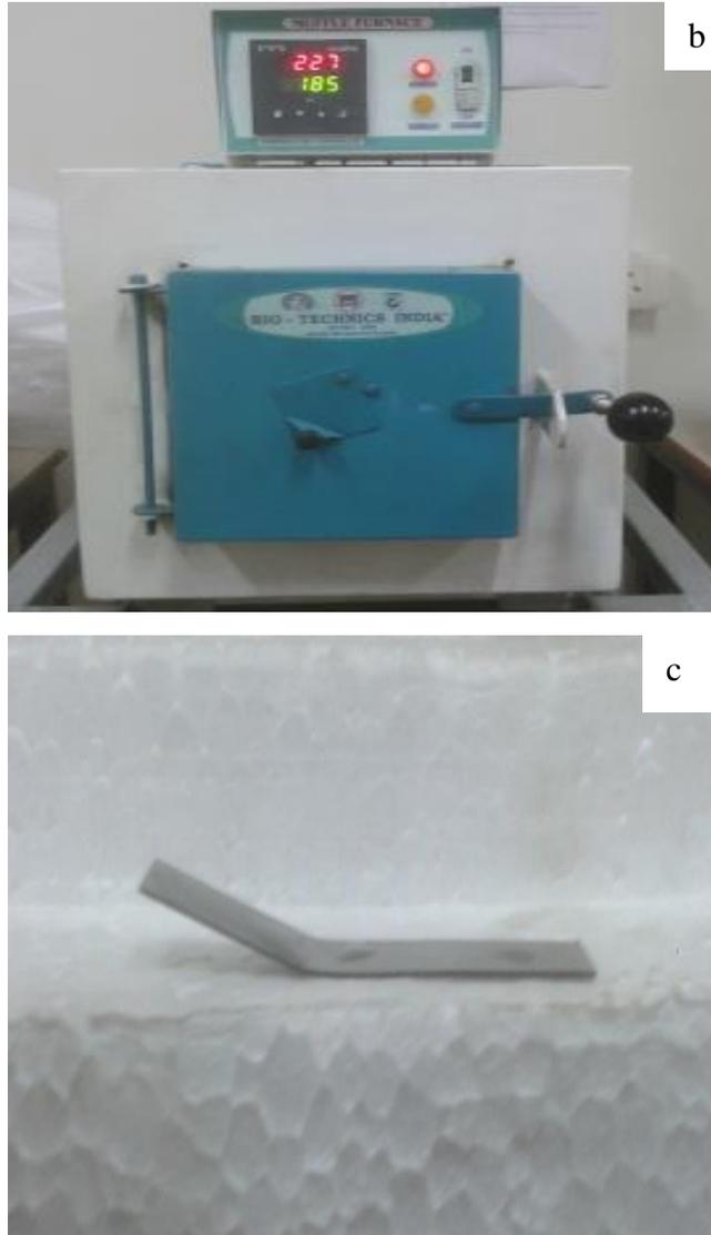
**Fig 5.11 : Apparatus used in Training a) Fixture, b) Muffle furnace, c) bent sheet**
