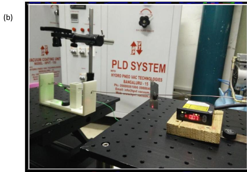
**Fig 5.27 a) Line beam generation by using quartz tube b) Displacement calculation using LDS and flapper arrangement**
