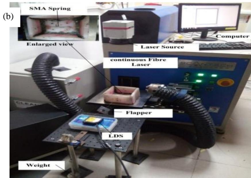
Fig. 6.1 a) schematic of laser assisted actuation and b) on line location of continuous laser assisted actuation
