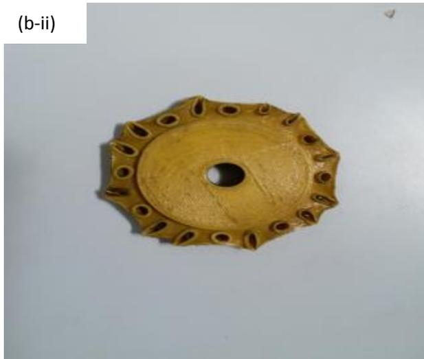
**Fig 4.27: a) Effect of exhaust gas on SMA wheel, a-ii) Thermal Image of wheel b-i) hub condition before and b-ii) after testing**
