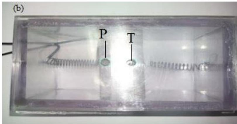
**Fig 6.15: a) A working model of Directional Control Valve, b) Top view of Directional Control Valve**
