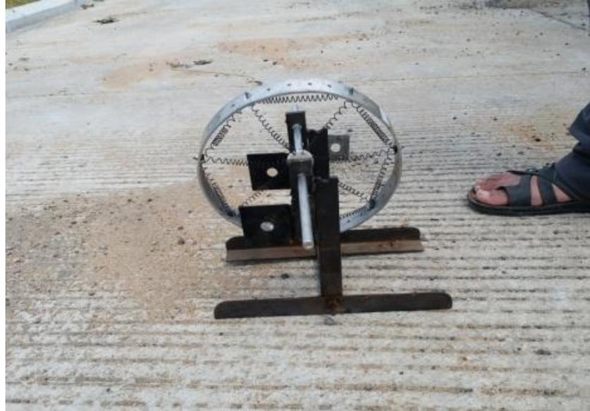
**Fig 4.29: Nitinol based wheel No. 3**
