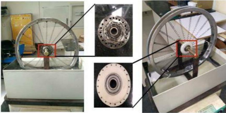
**Fig 4.16 MS bearing holder replaced by PLA material**
