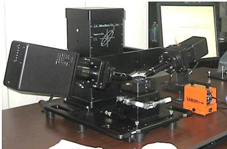
Figure 3.11. Photographic image of Variable Angle Variable Wavelength Spectroscopic Ellipsometry system.
