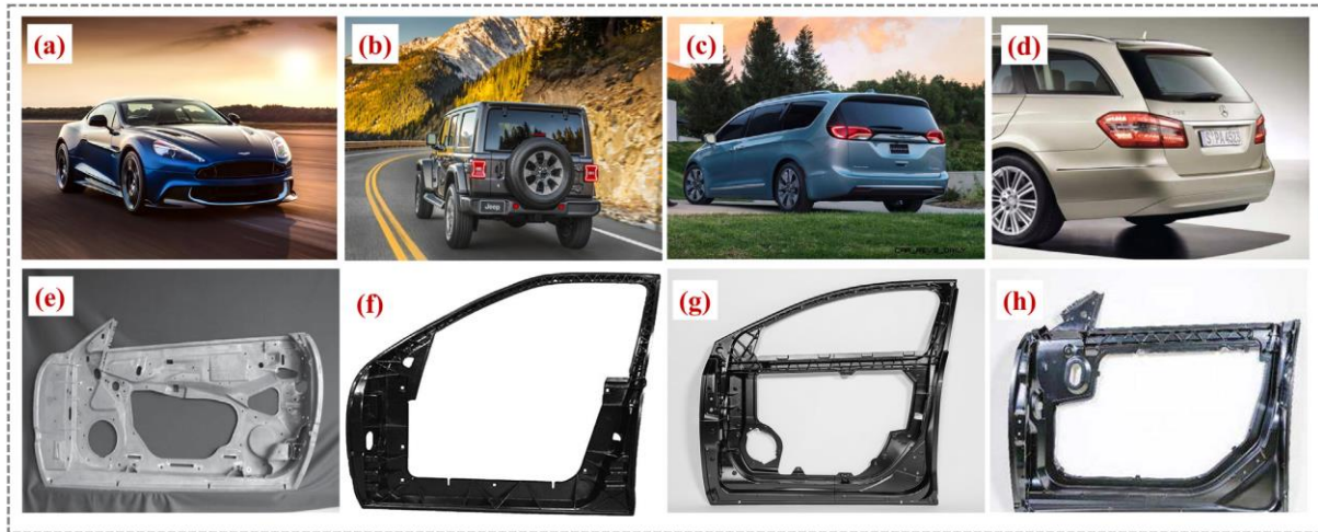
Fig. 2.35: Development and application of Mg alloys in car doors: (a) Aston Martin Vanquish S with cast Mg side door inner; (b) All-new 2018 Jeep Wrangler produced with a die-cast Mg rear swing gate; (c) Chrysler Pacifica showing the liftgate assembly highlighted by an Mg die-cast inner; (d) The rear end of the Mercedes-Benz E-Class T-Model featuring the hybrid Mg-Al hatchback; (e) Inner door frame of the Daimler-Chrysler SL Roadster; (f) Ford's concept die-cast Mg door inner with an open architecture; (g) Integrated Mg die-cast door inner designed (h) Ultra-thin and ultra-light Mg alloy door inner[1].
