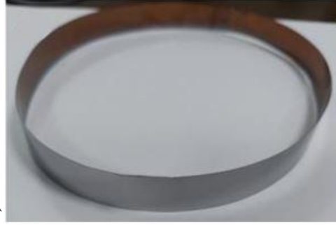
Fig 4.2: (a) Schematic of E-beam evaporation technique. (b) NiTi/Kapton polyimide belt after the deposition process.
