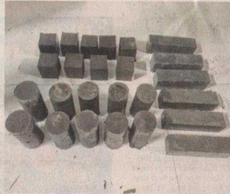
Cube, beam and cylinder sample of G-HSC for mechanical testing
