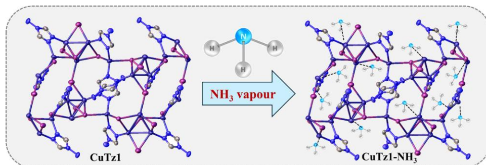
Fig. 4.13: Ammonia gas sensing mechanism with CuTz1 .
