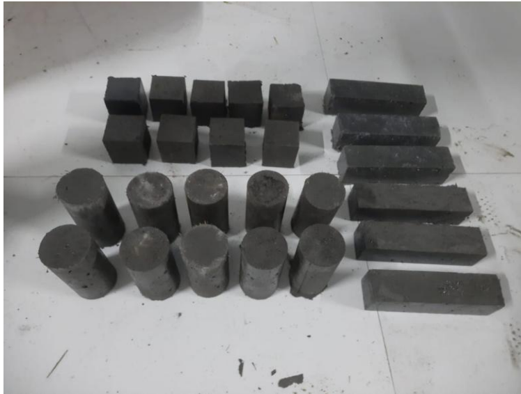
Fig.1. Cube, beam and cylinder sample of G-HSC for mechanical testing
