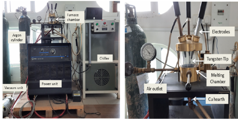
Figure 2.1: (a) Labeled image of the tri-arc furnace, and (b) the top image of the melting chamber.
