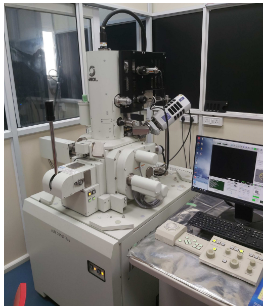
Figure 2.10: JSM-7610FPlus Schottky Field Emission Scanning Electron Microscope.
