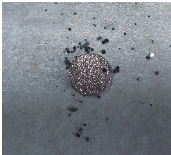
Figure 3.2: Polycrystal sample of \text{TiSe}_2
