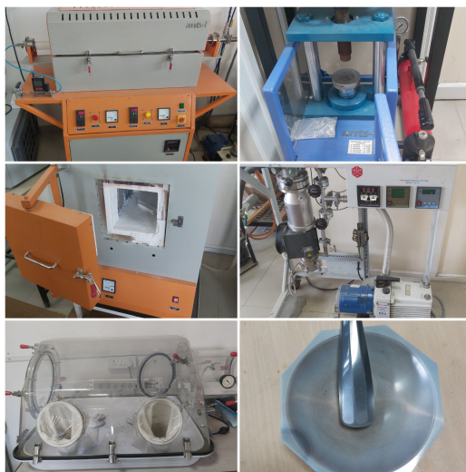
Figure 2.2: The fig. shows Two-zone furnace, Muffle furnace, Hydraulic press, Vacuum Sealing system, Glove box, and mortar-pestle.
