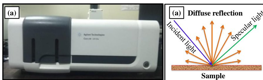
Figure 2.17: Experimental set up for diffuse reflectance measurement: (a) Carry 60 UV-Vis spectrometer and (b) schematic of diffuse reflectance.
