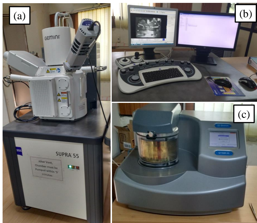
Figure 2.16: (a) Image of Supra55 Zeiss-FESEM used in our work, (b) Inca software attached within the computer for EDX and elementary mapping and (c) Gold coating set up.
