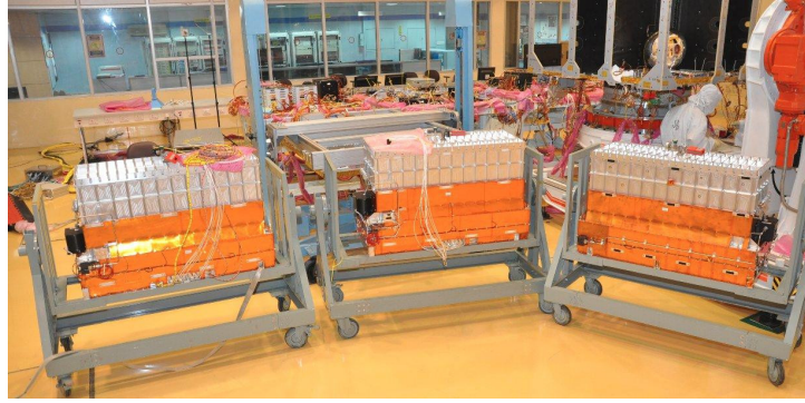
Figure 2.4: The three units of LAXPC. Image credit: TIFR.
