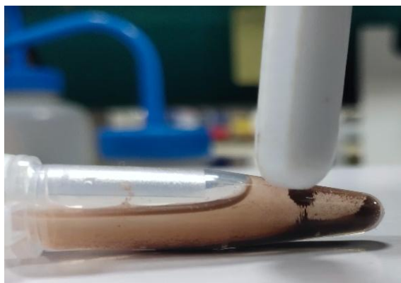
Figure 5.2: Iron oxide nanoparticles show a magnetic attraction toward a magnetic bar.
