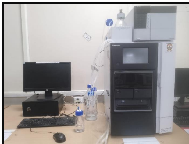
Figure 8. Prominence-i, LC-2030C 3D PLUS HPLC equipped with a fluorescence detector (RF-20A) CIF, BSBE, IIT Indore)
