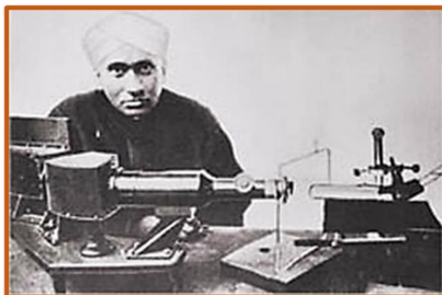
Figure 1.2: Sir C.V. Raman with the very first setup of the Raman spectrometer (image courtesy, IISc Bangalore)
