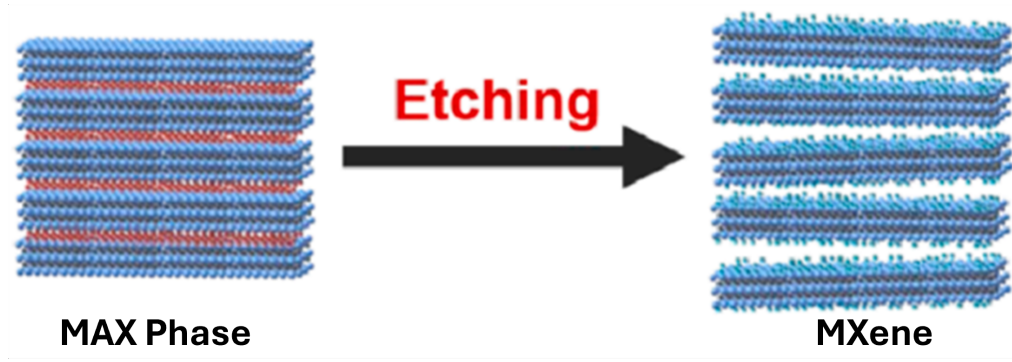
Figure 2.3: Schematic of etching of MAX phase material [26].
