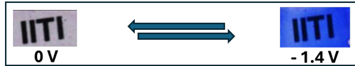
Figure 1.4: Optical modulation of EV electrode under negative bias.
