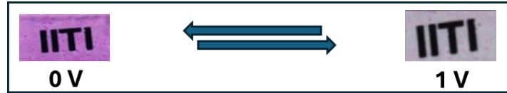
Figure 1.3: Optical modulation of P3HT electrode under positive bias.
