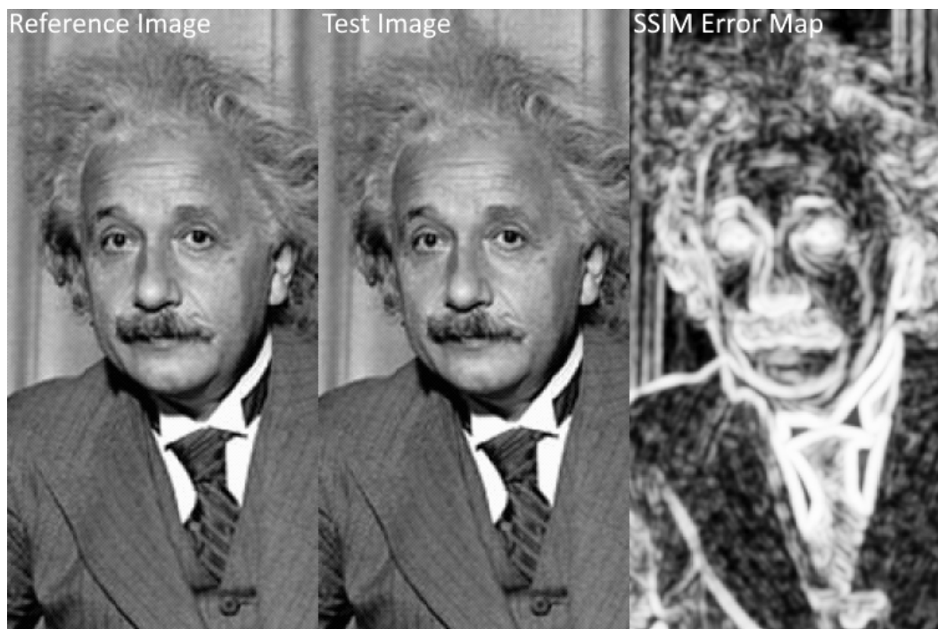
Figure 3.4: Example of SSIM ground truth map generation (Left: Reference Image, Center: Test Image, Right: SSIM Error Map)
