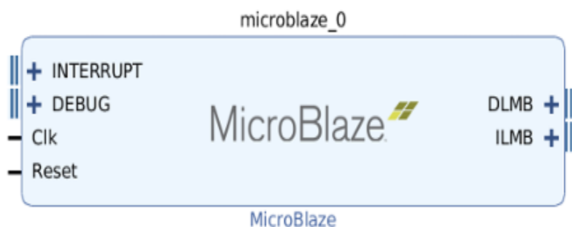
Fig.3.1 Microblaze IP block diagram
