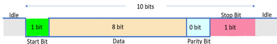
Fig.2.15 UART frame of data transmission and reception
