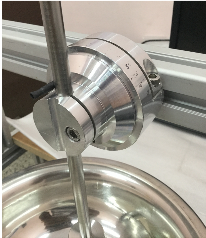
Figure 3.11: Image of Goniometer
