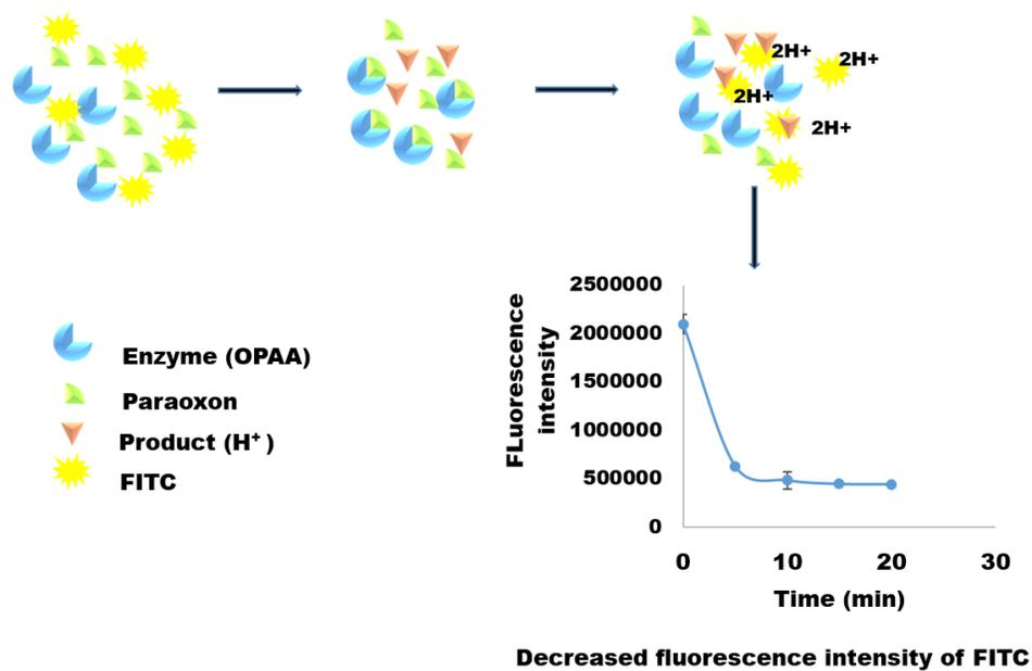
**Fig. 2.6: Diagrammatic representation of detection of OPs in FITC conjugated OPAA.** Reaction mixture containing paraoxon on hydrolysis by recombinant OPAA in presence of FITC drop the pH of the reaction mixture resulting in the intensity drop of the FITC.
