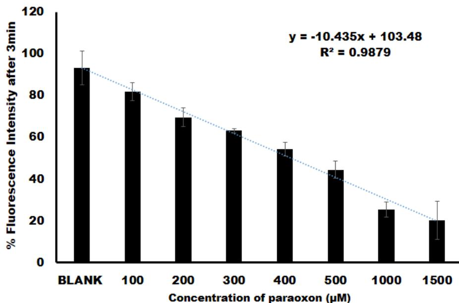
**Fig. 4.7: Histogram showing the change in the fluorescence intensity.** Change in the fluorescence intensity of FITC as compared to the blank after 3 minutes of incubation at 50° C. The linear range of paraoxon detection was observed between 100 µM to 1.5 mM.
