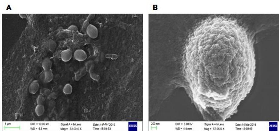
**Fig. 4.11: Characterization of encapsulated recombinant OPAA inside the alginate microsphere** A: Group of encapsulated OPAA inside 0.7 % alginate. B: Magnified image of the bead.
