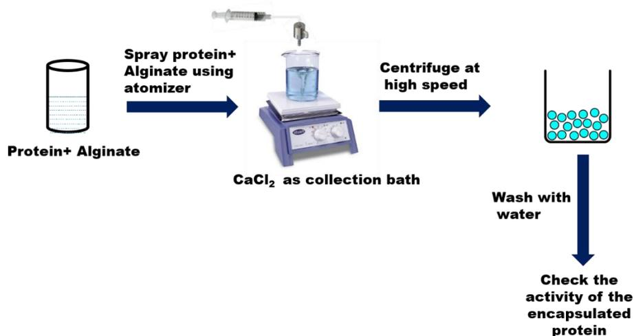
**Fig. 4.8: Diagrammatic representation of the encapsulation procedure.**
