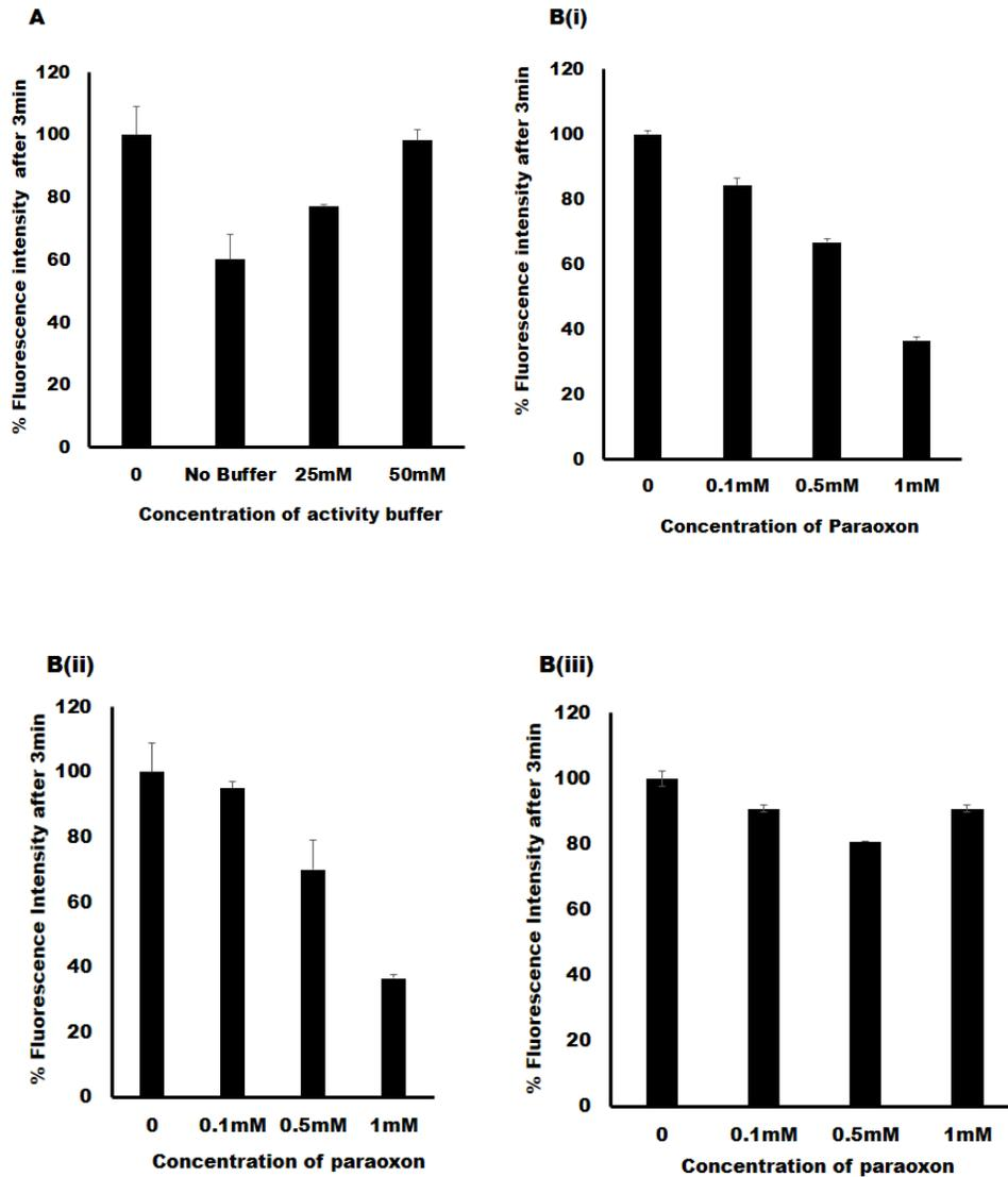
**Fig. 4.6: Optimization of activity assay** (A) Optimization of concentration of Bis-Tris Propane buffer. Drop in the intensity of FITC was more in case of the reaction mixture in which no activity buffer was used. (B) Optimization of protein: FITC (w/w). (i) 1:1 (ii) 3:1 (iii) 5:1. Highest activity was observed in case of Protein: FITC (1:1) W/W.
