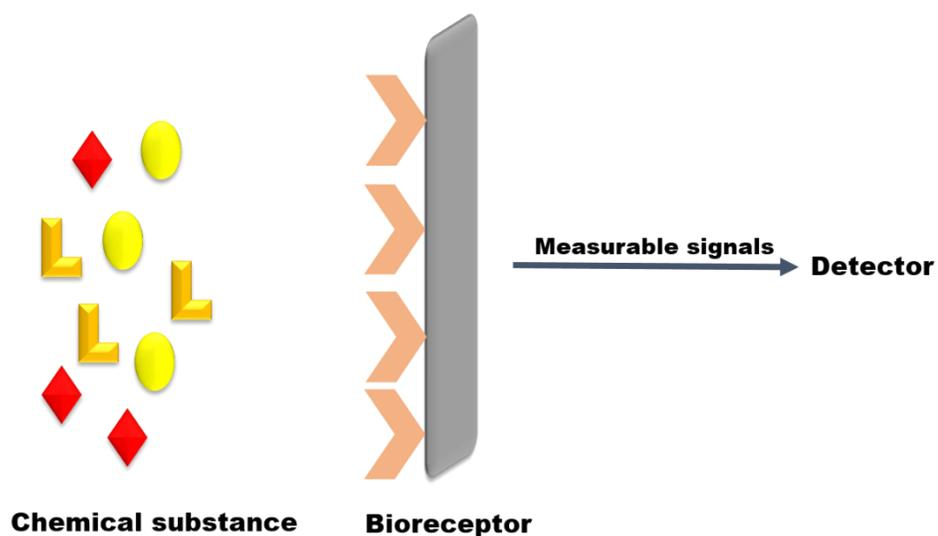
**Fig. 1.1: Diagrammatic representation of biosensor.** Biosensors includes two components, a biological component and a physiochemical detector. The biological component can be protein or the whole cell immobilized (represented as bio receptor) which on reacting with the analyte (represented as chemical substances) produces signal which are amplified and detected.
