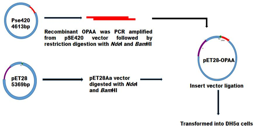
**Fig. 4.1: Construction of recombinant plasmid pET28a with recombinant OPAA gene.** Recombinant plasmid was constructed by ligating the fragments by Ligase.
