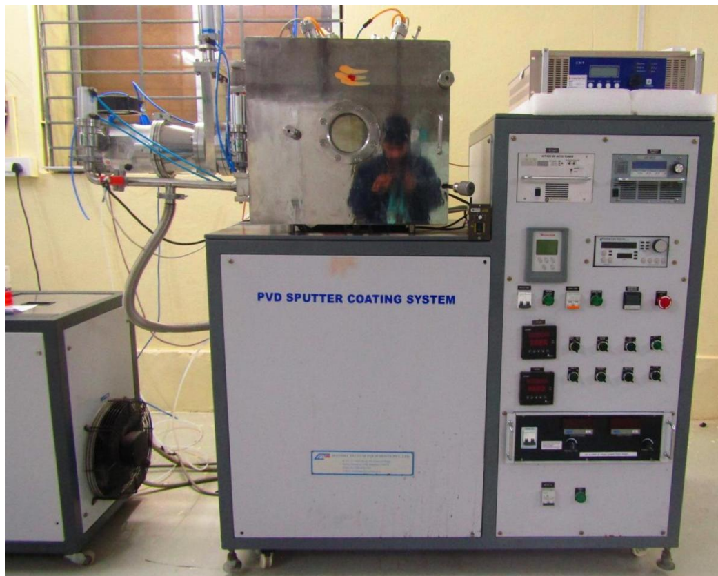
Figure 3.4: PVD sputter coating system used for thin film deposition, showing the main vacuum
