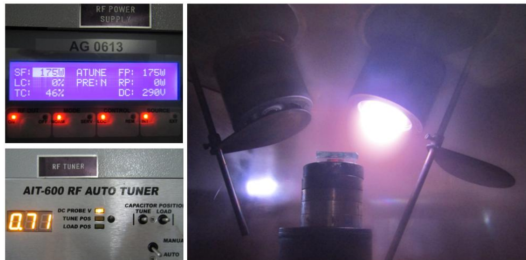
Figure 4.8: RF sputtering setup during Ti deposition, showing power supply and auto tuner settings (left) alongside plasma discharge and substrate positioning inside the vacuum chamber (right).
