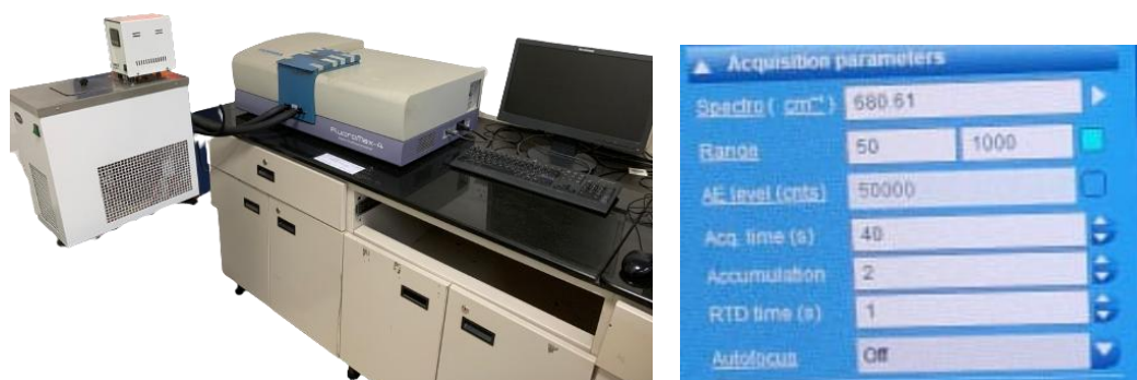
Figure 3.12. A Horiba Lab-Ram Micro-Raman spectrometer with an excitation wavelength of 632 nm was used for analyses of Ti-MoS 2 specimens
