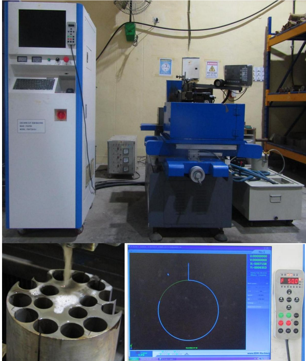
Figure 3.2: Wire EDM setup and operation: (top) CNC wire EDM machine used for precision machining; (bottom left) close-up of wire cutting multiple cylindrical samples; (bottom right) control panel and real-time display of the circular cutting path during machining.
