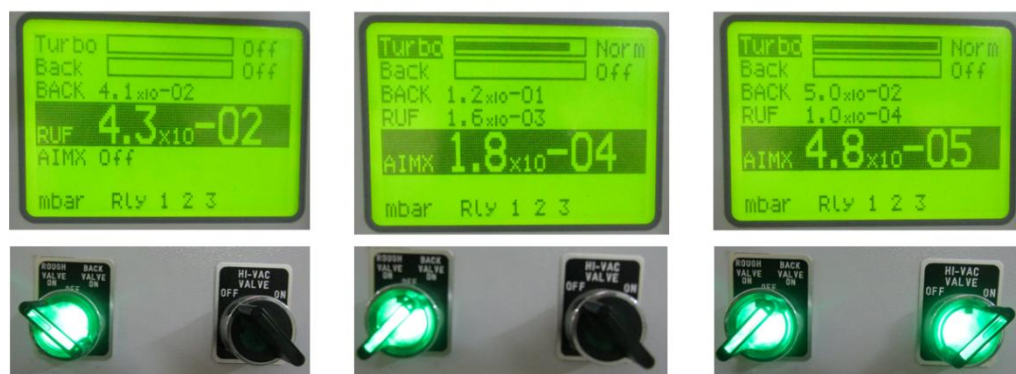
Figure 3.8: Sequential display of vacuum chamber evacuation steps for sputtering: (left) achieving sub- 5 \times 10^{-2} mbar with roughing pump; (center) switching to turbo pump and reaching 1.8 \times 10^{-4} mbar; (right) opening high vacuum valve to attain base pressure of 4.8 \times 10^{-5} mbar, with corresponding valve positions and control panel readings at each stage.
