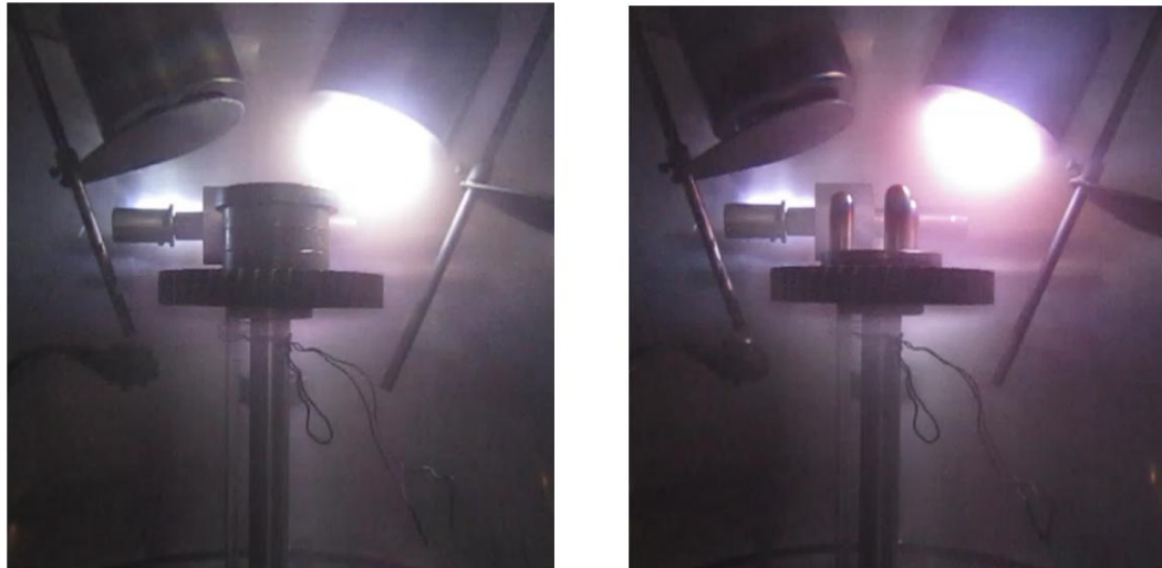
Figure 4.18: In-situ images of the custom substrate rotation mechanism during sputter coating, showing uniform plasma exposure for both disc (left) and bullet-shaped (right) samples to ensure consistent coating thickness and quality.
