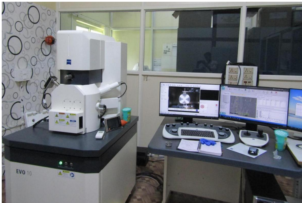
Figure 3.10: Laboratory scanning electron microscopes used for coating characterisation: (top) ZEISS EVO 10 SEM with integrated control workstation; (bottom) JEOL SEM system with high-resolution imaging capabilities, both employed for detailed surface and cross-sectional analysis of thin film coatings.
