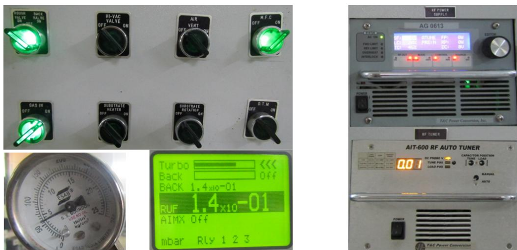
Figure 3.9: Sputtering system operation sequence: (left) Valve and gas flow control panel,
