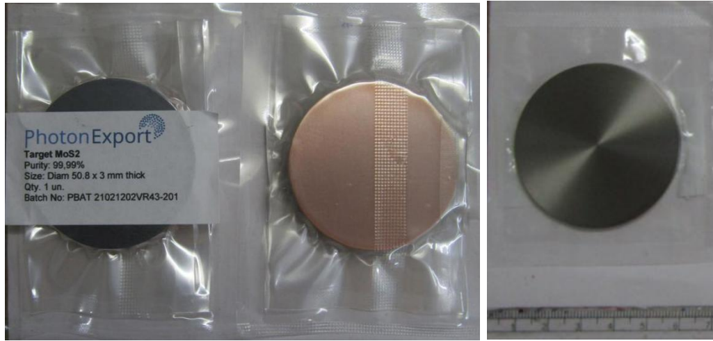
Figure 3.5: Front and back views of a MoS 2 sputtering target bonded to a copper backing plate (left and centre), and a pure titanium (Ti) sputtering target (right), both used for thin film deposition in PVD processes.
